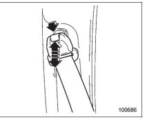
The shoulder belt anchor height should be adjusted to the best position for the passenger. To adjust the anchor height, push the release button and slide the anchor up or down. Pull down on the anchor to make sure that it is locked in place.
