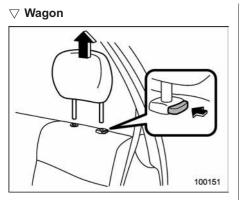
1. Remove the headrest at the windowside seating position where the child restraint system has been installed with the lower anchorages or seatbelt; lift up the headrest while pressing the release button. Store the headrest in the cargo area. Avoid placing the headrest in the passenger compartment to prevent it from being thrown around in the passenger compartment in a sudden stop or a sharp turn.
