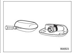
1. Remove the high mount stop light cover by prying the edge with a screw-driver.
