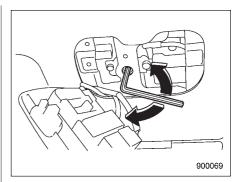
4. Insert the wrench in the end of the motor shaft.
