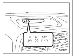
To set the hour, press the "H" button. To set the minutes, press the "M" button. To reset the minutes to "00" with a radio time signal, push the "SET" button.
