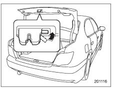
The inside trunk lid release can be canceled to prevent unauthorized entry into the trunk. To cancel the trunk lid release, set the lid release cancel lever (located on the inside of the trunk lid, mounted to the trunk lid latch) to the "CANCEL" position. When this lock is in the "CANCEL" position, the trunk can be opened only with the key.
