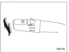
To change from low beam to high beam, push the turn signal lever forward. When the headlights are on high beam, the high beam indicator light " $\Xi$ O" on the instrument panel is also on.
