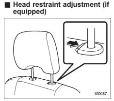
To raise the head restraint, pull it up. To lower it, push the head restraint down while pressing the release button on the top of the seatback.
