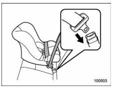
1. Place the child restraint system in the rear seating position.
