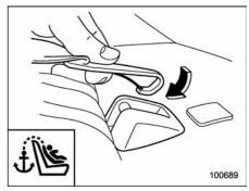
Attach the child restraint top tether hook to the appropriate upper anchorage.
