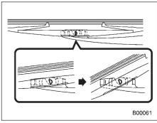
2. Turn the wiper blade assembly counterclockwise.
