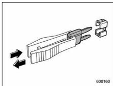
4. Pull out the fuse with the fuse puller.
