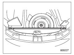
For the vehicles equipped with an underfloor storage compartment, the cargo area cover can be stowed under the cargo floor.
