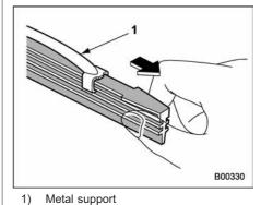
1. Grasp the locked end of the blade rubber assembly and pull it firmly until the stoppers on the rubber are free of the metal support.
