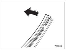
1. Pull out the end of the blade rubber assembly to unlock it from the plastic support.
