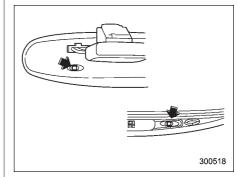
The mirror has a photosensor attached on both the front and back sides. If the glare from the headlights of vehicles behind you strikes the mirror, these sensors detect it and make the reflection surface of the mirror dimmer to help prevent you from being blinded. For this reason, use care not to cover the sensors with stickers, or other similar items. Periodically wipe the sensors clean using a piece of dry soft cotton cloth or an applicator.
