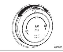
This dial is used to set the desired interior temperature. With the dial set to your desired temperature, the system automatically adjusts the temperature of air supplied from the outlets such that the desired temperature is achieved and maintained.
