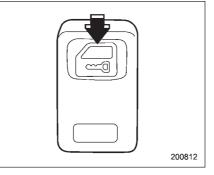
5. Before the electronic tone stops sounding, push the lock side of the power door lock switch the same number of times as the leftmost digit of the transmitter code. For example, push the lock switch eight times if the leftmost digit of the code is 8.
