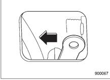
3. Unlock the rear gate by pressing the lever inside the trim to the left.
