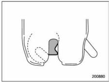
3. Move the release handle, from outside the vehicle, in the direction of the arrow to check if the latch is released. If the latch is not released, contact your SUBARU dealer.
