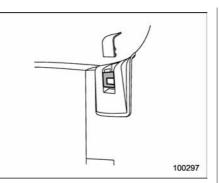
2. (For both window-side seating positions) Remove the cap from the anchor fitting cover.
