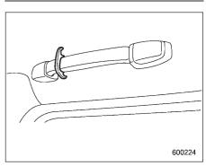
The coat hook is attached to the rear left and rear right passenger's hand grip.
