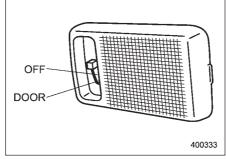
**DOOR:** The light comes on only when the rear gate is opened. **OFF:** The light stays off.
