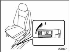
Pull the trunk lid release lever upward.
