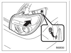
7. Put the rear combination light assembly into place while aligning the clip with the guide on the vehicle and fasten the bolts.
