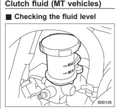
Check the fluid level on the outside of the reservoir. If the level is below "MIN" level mark, add the recommended clutch fluid to "MAX" level mark.
