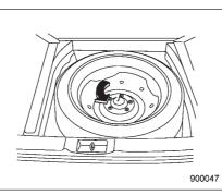
**Sedan:** Remove the floor cover from the trunk. Turn the attaching bolt counter-clockwise, then take the spare tire out.
