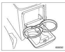
A dual cup holder is located at the back of the center console. To use the cup holder, open the lid by pulling its upper edge.
