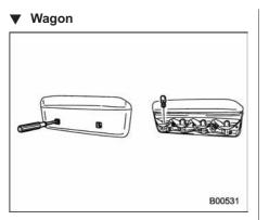
1. Remove the mounting screws using a Phillips screwdriver and then remove the high mount stop light cover.
