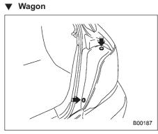
1. Using a Phillips screwdriver, remove the upper and lower clips that secure the side cover of the rear combination light assembly.
