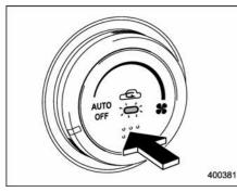
**ON position (Recirculation):** Interior air is recirculated inside the vehicle. Push the air inlet selection button to the ON position
