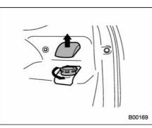
The tank is located on the right-hand side of the trunk.
