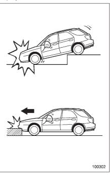
Only the driver's SRS frontal airbag or both driver's and front passenger's SRS frontal airbags may be activated when the vehicle sustains a hard impact in the undercarriage area from the road surface (such as when the vehicle plunges into a deep ditch, is severely impacted or knocked hard against an obstacle on the road such as a curb). ▽ Examples of the types of accidents in which deployment of the driver's/ driver's and front passenger's SRS frontal airbag(s) is unlikely to occur.
