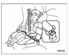
4. To remove the booster seat, press the release button on the seatbelt buckle and allow the belt to retract.
