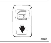
6. When you have finished entering the number, push the unlock side of the lock
