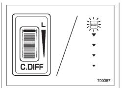
Turn the dial forward to increase the initial LSD torque; when the white line on the dial reaches the frontmost position, the initial LSD torque setting is maximum. The center differential will then be almost completely locked and the "LOCK" indicator light will come on.
