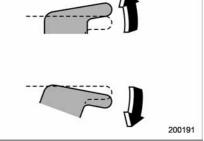
To open the passengers' windows, push the appropriate switch down and hold it until the window reaches the desired position.
