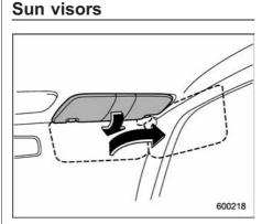
To block out glare, swing down the visors. To use the sun visor at a side window, swing it down and move it sideways. ■ Vanity mirror (if equipped)
