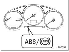
The ABS warning light comes on when the ignition switch is turned to the "ON" position and goes out after approximately 2 seconds.
