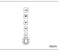
The bottom indicator light "[]" flashes in the event of failure of the driver's control center differential. Have the vehicle inspected by your SUBARU dealer. For details, refer to Chapter 7, "Driver's Control Center Differential (DCCD) (WRX-STI)".
