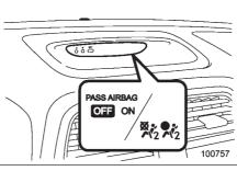
ON or \$\$2: Front passenger's frontal airbag ON indicator
