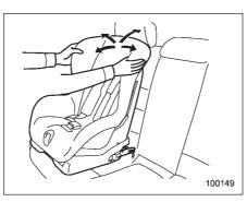
3. [If your child restraint system is of a flexible attachment type (which uses tether belts to connect the child restraint system properly to the lower anchorages)] While pushing the child restraint into the seat cushion, pull both left and right lower tether belts up to secure the child restraint system firmly by taking up the slack in the belt.
