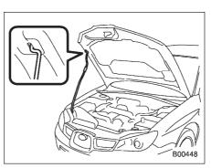
Lift up the hood, release the hood prop from its retainer and put the end of the hood prop into the slot in the hood.
