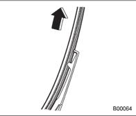
2. Pull the blade rubber assembly out of the plastic support.
