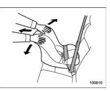
6. Push and pull the child restraint system forward and from side to side to check if it is firmly secured. Sometimes a child restraint can be more firmly secured by pushing it down into the seat cushion and then tightening the seatbelt.
