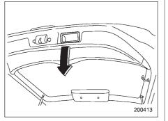
To close the rear gate, lower it slowly and push down firmly until the latch engages. The rear gate can be lowered easily if you pull it down holding the recessed grip.
