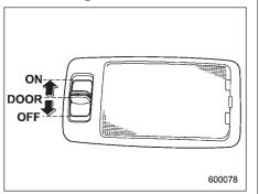
The dome light switch has three positions:
