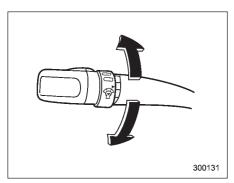
To brighten, turn the control dial upward. To darken, turn the control dial downward. Headlight beam leveler (U.S.spec. WRX-STI)
