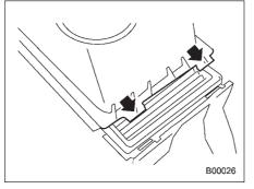
4. To install the air cleaner case cover, insert the two projections on the air cleaner case cover into the slits on the air cleaner case and then snap the two clamps on the air cleaner case cover.
