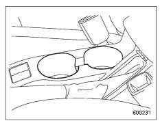
A dual cup holder is built in the center console, beside the parking brake lever.
