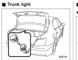
1. Remove the cover by squeezing its sides and pulling it.
