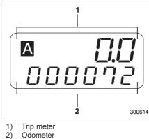
This meter displays the odometer and two trip meters.
