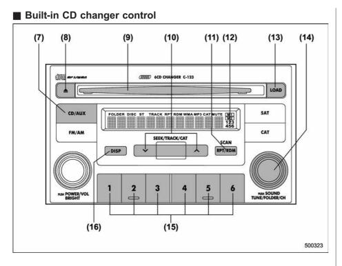
(7) CD button(8) Eject button(9) Disc slot
