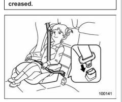
1. Place the booster seat in the rear seating position and sit the child on it. The child should sit well back on the booster seat.
