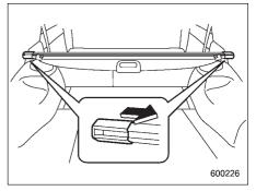
2. Pull either sleeve on the end of the cover housing to shorten the cover's length.
