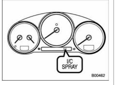
• The intercooler water spray warning light comes on when the water level in the tank has dropped to the lower limit. If the warning light illuminates, refill the tank with water. The tank is located on the right-hand side of the trunk. For the tank refilling method, refer to the "Intercooler water spray (WRX-STI)" section in chapter 11.
