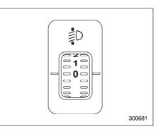
The WRX-STI version has High-Intensity Discharge (HID) headlights on the low beam setting. The HID headlights generate more light than conventional halogen headlights. Therefore a driver of an oncoming vehicle may experience too much glare when your headlight beam height adjustment is high due to the vehicle carrying heavy load.
