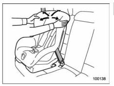
6. Before having a child sit in the child restraint system, move it back and forth and right and left to check if it is firmly secured. Sometimes a child restraint can be more firmly secured by pushing it down into the seat cushion and then tightening the seatbelt.
