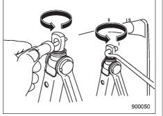
If the jackscrew is too tight to be loosened by hand, loosen it using a screwdriver or the jack handle.
