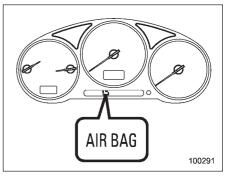
A diagnostic system continually monitors the readiness of the seatbelt pretensioner while the vehicle is being driven. The seatbelt pretensioners share the control module with the SRS airbag system. Therefore, if any malfunction occurs in a seatbelt pretensioner, the SRS airbag system warning light will illuminate. The SRS airbag system warning light will show normal system operation by lighting for approximately 6 seconds when the ignition switch is turned to the "ON" position.
