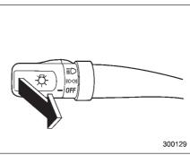
To flash the headlights, pull the lever toward you and then release it. The high beam will stay on for as long as you hold the lever. The headlight flasher works even though the light switch is in the "OFF" position.
