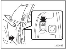
6. Push the front side ("LOCK" side) of the power door locking switch to set the door locks.
