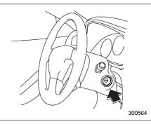
The ignition switch has four positions: LOCK, Acc, ON and START.
