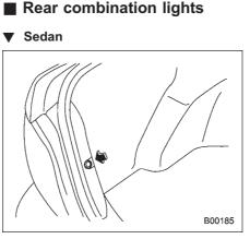
1. Remove the clip from the rear trunk trim with a screwdriver.
