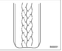
Rolling resistance is high, so fuel consumption is also higher. • Abnormally high tire pressure (tread worn in center)
