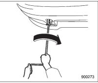
4. Tighten the towing hook securely using the jack handle.
