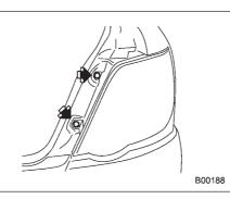
3. Remove the upper and lower bolts. Then, slide the rear combination lamp assembly to the rear and remove it from the vehicle.
