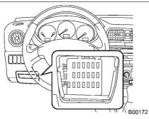
One is located under the instrument panel behind the coin tray on the driver's seat side.
