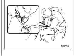
3. After confirming that the webbing is not twisted, insert the connector (tongue) attached at the webbing end into the buckle on the right-hand side until a click is heard.
