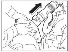
2. Push the air cleaner case cover in the direction of the arrow shown in the drawing.
