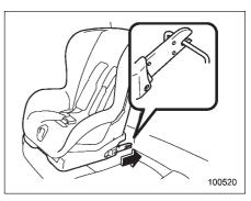
2. While following the instructions supplied by the child restraint system manufacturer, connect the lower hooks onto the lower anchorages located at "(a)" marks on the bottom of the rear seatback. When the hooks are connected, make sure the adjacent seatbelts are not caught.
