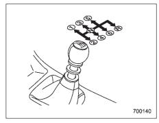
The manual transmission is a fully synchromeshed, 6-forward-speed and 1-reverse-speed transmission.
