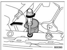
Before replacing the left-hand (batteryside) high-beam light bulb, remove the screw that retains the windshield washer nozzle and tip the windshield washer nozzle sideways.
