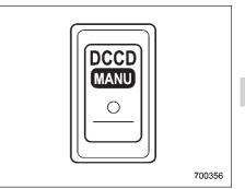
Press the "DCCD-MANU" switch on the center console to switch from auto mode to manual mode. The "AUTO" indicator light in the combination meter will go off. Press the switch again to go back to auto mode. The "AUTO" indicator light in the combination meter will come on.
