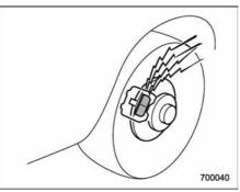
The disc brake pad wear warning indicators on the disc brakes give a warning noise when the brake pads are worn.
