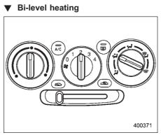
This setting allows you to direct air of different temperatures from the instrument panel and foot outlets. The air from the foot outlets is slightly warmer than from the instrument panel outlets.
