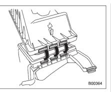
5. To install the air cleaner case cover, insert the three projections on the air cleaner case into the slits on the air cleaner case cover and then snap the two clamps on the air cleaner case cover.
