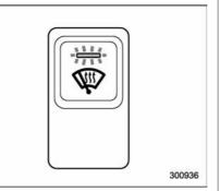
The windshield wiper deicer operates only when the ignition switch is in the "ON" position.
