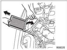
2. Open the air cleaner case cover and remove the air cleaner element.
