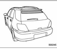
The antenna is printed on the inner surface of the rear window glass.
