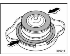
3. After refilling the reserve tank and the radiator, reinstall the caps and check that the rubber gaskets inside the radiator cap are in the proper position.
