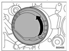
1. Remove the bulb cover, by turning it counterclockwise.
