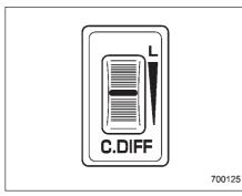
The control dial is located beside the parking brake lever. By turning the control dial forward and rearward, it is possible to change the initial LSD torque.
