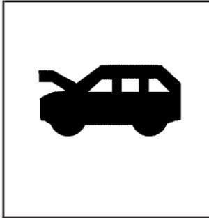
1. Pull the handle with this symbol on it. It is located under the instrument panel on the driver side of the vehicle.
