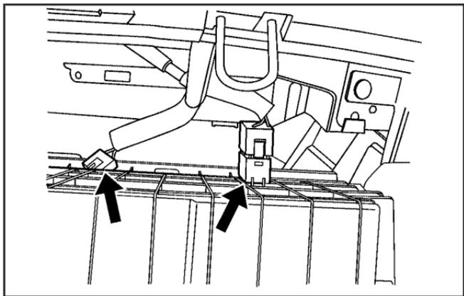
3. Unplug both wire cables and remove the glove box.
