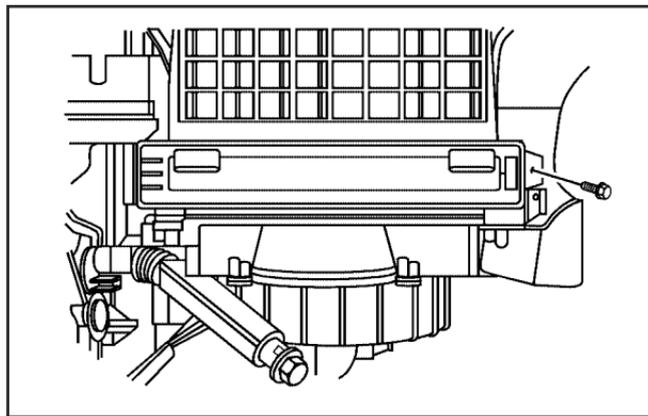
4. Remove the air filter cover screw.
