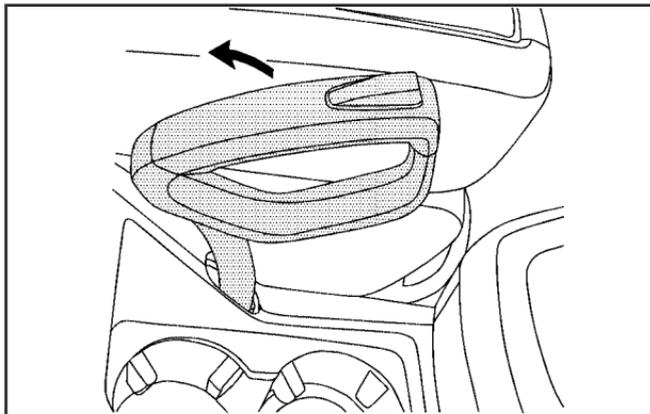
The parking brake lever is located to the right of the driver's seat.
