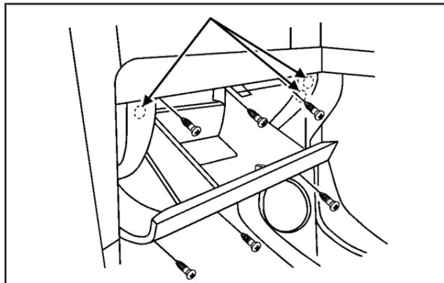
2. Lower the loosened glove box housing.
