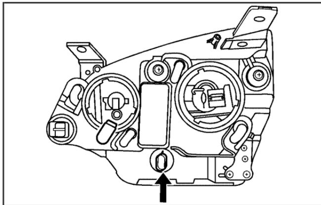
2. Turn the bulb to be replaced counterclockwise to remove it from the headlamp assembly.
