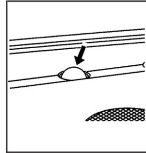
There is a light sensor located on top of the instrument panel. Make sure it is not covered, or the headlamps will come on when they are not needed.
