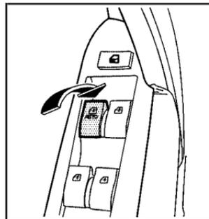
The window switches for all doors are located on the driver's door.
