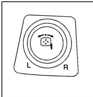
The outside power mirror control is located on the driver side door.
