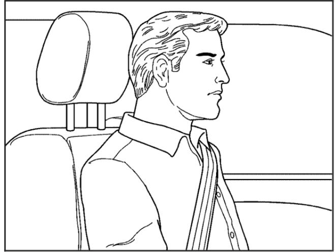
Adjust the head restraint so that the top of the restraint is at the same height as the top of the occupant's head. This position reduces the chance of a neck injury in a crash.
