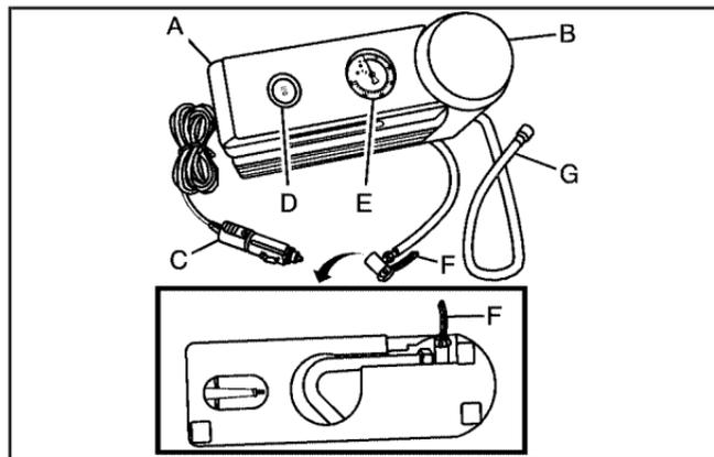
1. Unlock the air only hose (F) from the sealant canister (B) by pulling up on the lever.
