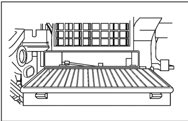
5. Remove the filter cover and pull out the old air filter.
