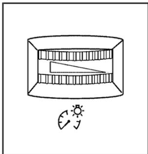
The thumbwheel for this feature is located on the left side of the steering wheel next to the exterior lamps control.
