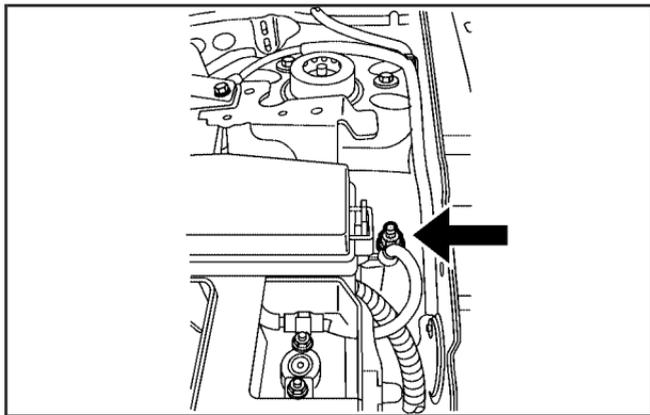
5. The remote negative (-) terminal is a stud on the driver side near the underhood fuse block.
