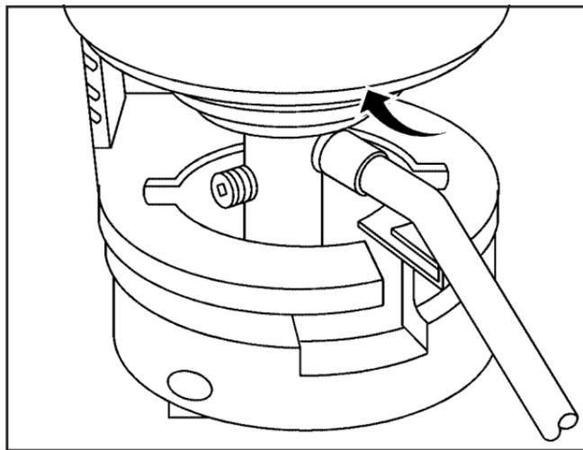
3. Turn the sealant canister so the inflator filling hose is aligned with the slot in the compressor.
