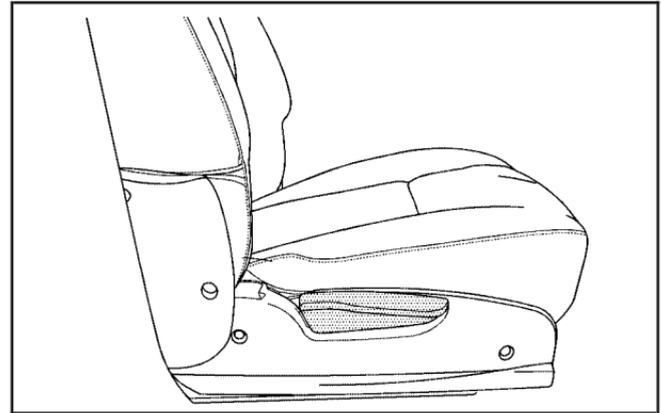
3. Lift up fully on the recliner lever, located on the outboard side of the seat, and fold the seatback forward until it disengages.
