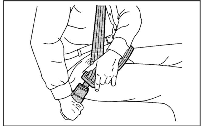
3. Push the latch plate into the buckle until it clicks. Pull up on the latch plate to make sure it is secure. If the belt is not long enough, see *Safety Belt Extender on page 1-30*.
