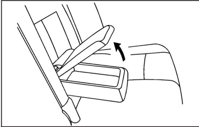
To access the rear seat armrest, pull the handle down. Lift the top of the armrest to access the storage area.
