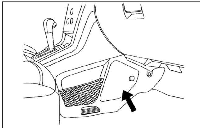
Pull the latch of the fuse box cover straight back to access the fuses.
