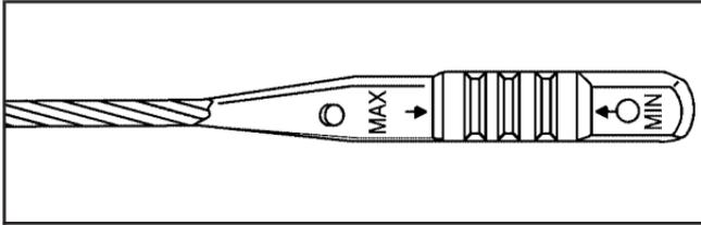
If the oil is below the MIN (minimum) mark, add at least one quart/liter of the recommended oil. This section explains what kind of oil to use. For engine oil crankcase capacity, see *Capacities and Specifications on page 5-98*.
