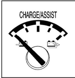
The CHARGE/ASSIST gage displays the charge (current) into and out of the hybrid battery.
