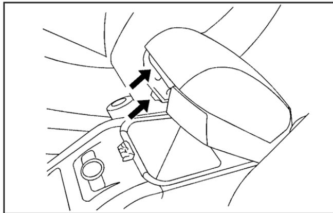
Your vehicle has a center console with an upper, lower and rear storage area. To access the upper storage area, lift up on the top lever. To access the lower storage area, lift up on the bottom lever. The top of the center console can extend forward. To adjust, hold the top of the lever up and pull the top of the center console forward.
