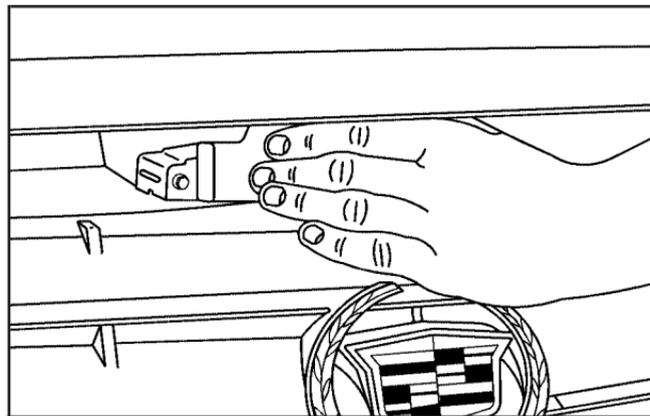
2. Then go to the front of the vehicle and find the secondary hood release lever. The lever is located under the front edge of the grille near the center. Move the release lever to the side and raise the hood.
