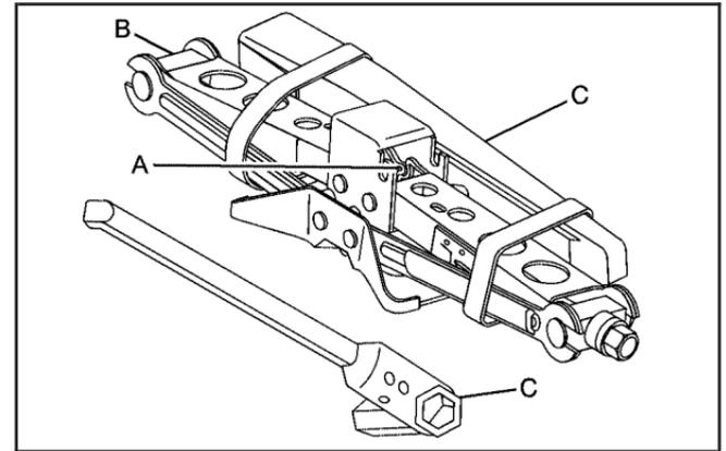
2. Turn the wing nut (A) holding the jack (B) (and storage tray, if applicable) counterclockwise and remove it.
