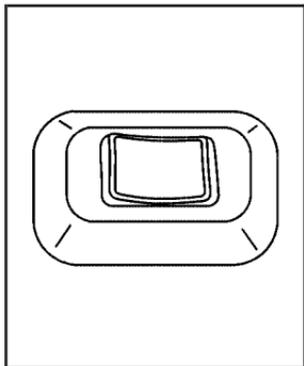
The vehicle may have this feature. The driver and passenger seatback lumbar support can be adjusted by moving the control located on the outboard side of the seat cushions.
