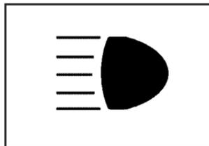
The highbeam light on the instrument panel cluster, comes on while the high-beam headlamps are on.
