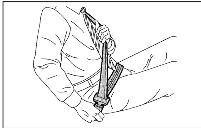
4. Push the latch plate into the buckle until it clicks. Pull up on the latch plate to make sure it is secure. If the belt is not long enough, see *Safety Belt Extender* on page 1-32. Make sure the release button on the buckle is positioned so you would be able to unbuckle the safety belt quickly if necessary.
