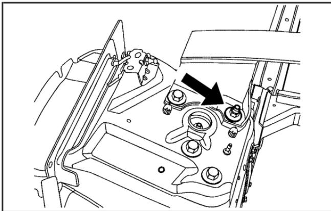
Your vehicle has a remote negative (-) ground location, as shown in the illustration. It is located on the passenger side front shock tower. See *Engine Compartment Overview on page 5-12*. You should always use this remote ground location, instead of the terminal on the battery.
