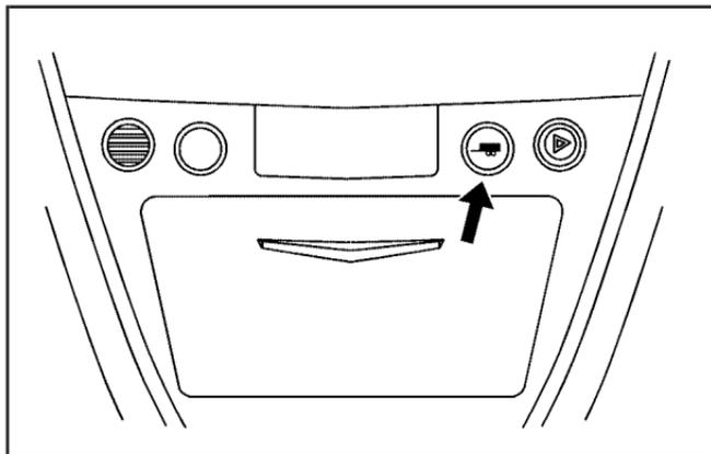
The vehicle may be equipped with a Tow/Haul mode. The button is located on instrument panel under the climate controls. You should use this feature to assist when towing or hauling a heavy load.
