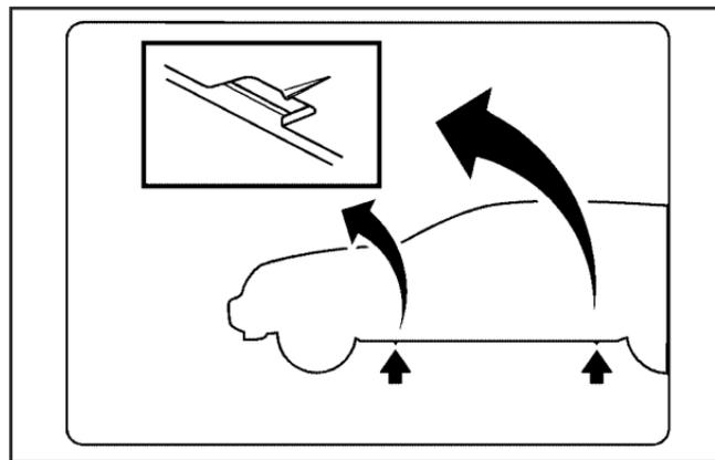
3. Find the jacking location using the V-shaped notches located in the plastic molding.
