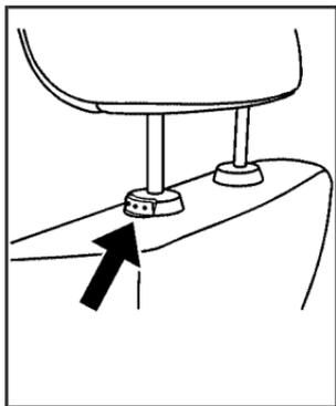
Pull the restraint up to raise it. To lower it, press the button, located on the top of the seatback, and push the head restraint down.
