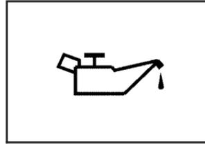
For vehicles with an oil pressure light, if there is a problem with the oil, the light may stay on after the engine is started, or comes on while driving.
