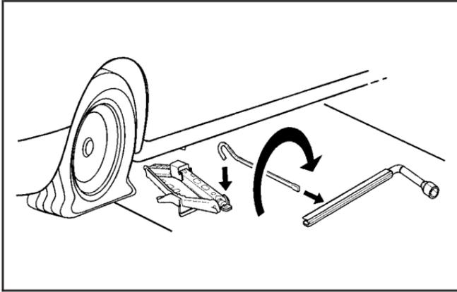
8. Raise the vehicle by turning the wheel wrench clockwise. Raise the vehicle far enough off the ground for the compact spare tire to fit under the vehicle.
