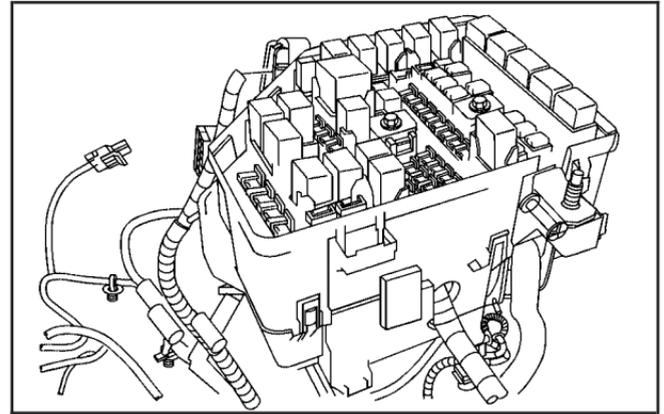
To access the fuses, push in the two tabs located on each side of the fuse block cover. Then lift the cover off.
