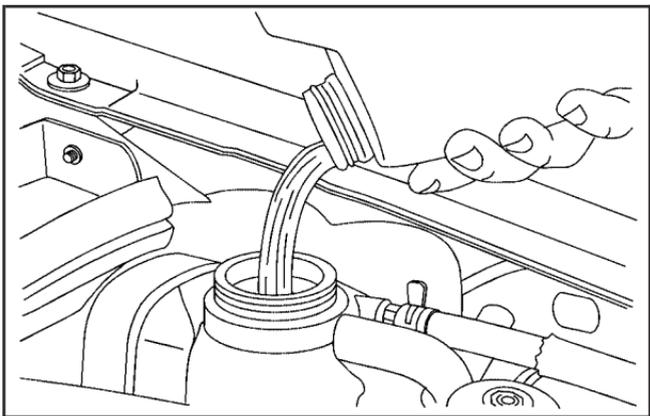
3. Fill the coolant surge tank with the proper DEX-COOL® coolant mixture, to slightly above the FULL COLD/FROID line on the side of the coolant surge tank.
