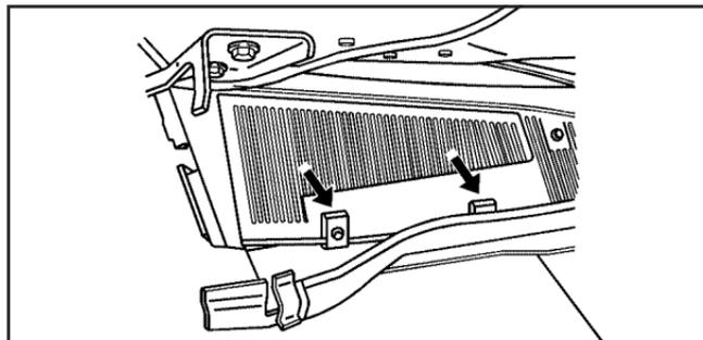
2. Push the two tabs on the access panel door towards the windshield.
