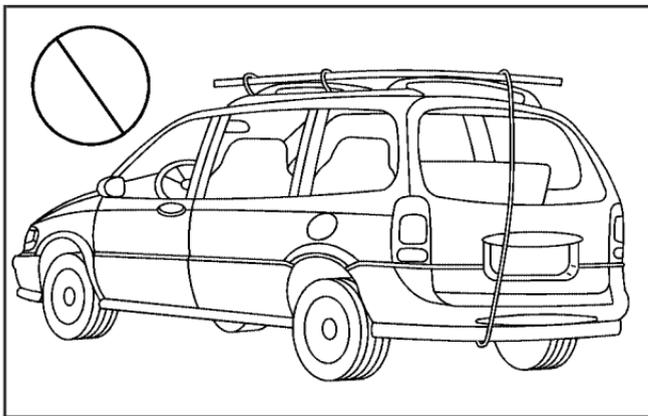
If your vehicle has a luggage carrier, you can load things on top of your vehicle. The luggage carrier has side rails attached to the roof. You can get sliding crossrails through your dealer to use for tying things down. These let you load some things on top of your vehicle, as long as they are not wider or longer than the luggage carrier.
