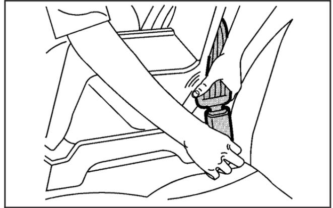
4. Push the latch plate into the buckle until it clicks. Make sure the release button is positioned so you would be able to unbuckle the safety belt quickly if necessary.
