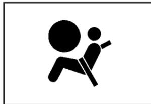
The airbag readiness light flashes for a few seconds when the engine is started. If the light does not come on then, have it fixed immediately.
