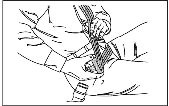
3. If the belt stops before it reaches the buckle, tilt the latch plate and keep pulling until you can buckle the belt.
