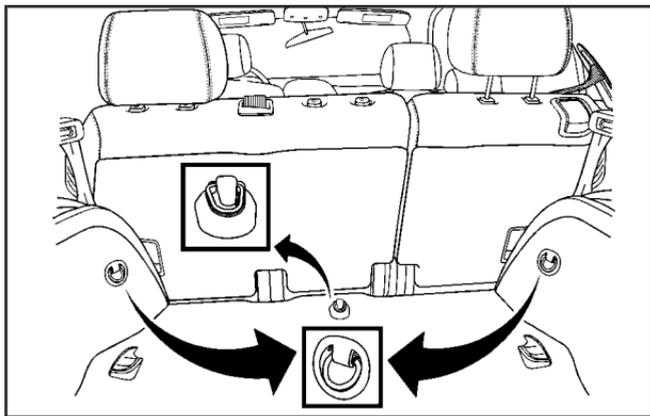
There are two top tether anchors located on the side of the wheel well in the rear cargo area. There is another top tether anchor in the center of the rear cargo area. Be sure to use an anchor located on the same side of the vehicle as the seating position where the child restraint will be placed.
