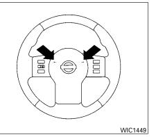
To sound the horn, push the area between the horn icons on the steering wheel.
