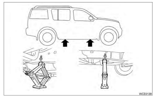
Place the jack directly under the jack-up point as illustrated so the top of the jack contacts the vehicle at the jack-up point. The jack-up points are indicated by stamped arrows on the side of the frame. The jack should be used on firm and level ground.
