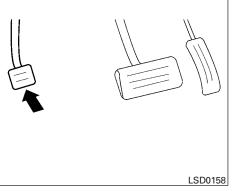
To engage: Firmly depress the parking brake.
