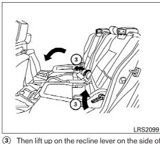
Then lift up on the recline lever on the side of the outboard seats to fold the outboard seatbacks flat. To fold the center seatback flat, pull up on the strap on the edge of the center seat cushion and fold the seatback toward the front of the vehicle.
