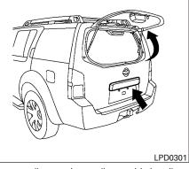
To open, pull up on the smaller outside handle to release the glass hatch, then pull up on the glass hatch. To close, lower and push the glass hatch down securely.
