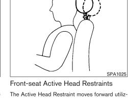
The Active Head Restraint moves forward utilizing the force that the seatback receives from the occupant in a rear-end collision. The movement of the head restraint helps support the occupant's head by reducing its backward movement and helping absorb some of the forces that may lead to whiplash-type injuries.
