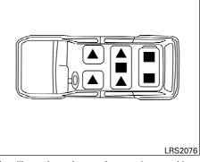
The illustration shows the seating positions equipped with adjustable headrests. All of the headrests are adjustable.
