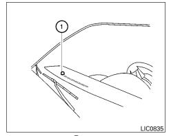
The sunload sensor (1), located on the top center of the instrument panel, helps the system maintain a constant temperature. Do not put anything on or around this sensor. Rear seat temperature and fan speed can be controlled from both the front seat overhead console controls or the rear seat controls (on back of center console).
