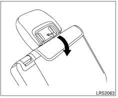
2. Pull the strap to release the head restraint rearward.
