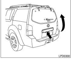
The power door lock system allows you to lock or unlock all doors including the lift gate simultaneously.
