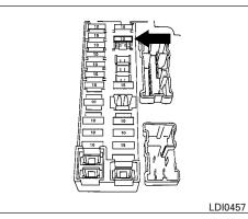
If a type A fuse is used to replace a type B fuse, the type A fuse will not be level with the fuse pocket as shown in the illustration. This will not affect the performance of the fuse. Make sure the fuse is installed in the fuse box securely.
