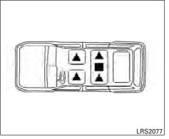
The illustration shows the seating positions equipped with head restraints. The second row head restraints are removable but not adjustable.
