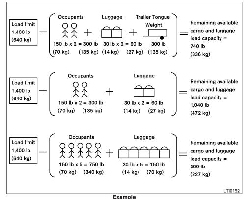
Steps for determining correct load limit
