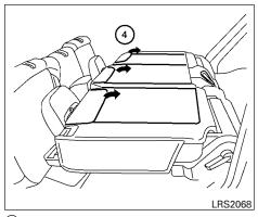
(4) There is a carpet panel flap on the back of each seat that can be folded toward the back of the vehicle.
