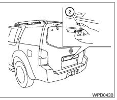
or liftgate does not unlock after returning the handle, push the door handle request switch to unlock the door and liftgate.
