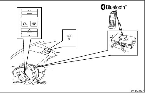
Your NISSAN is equipped with the Bluetooth<sup>®</sup> Hands-Free Phone System. If you have a compatible Bluetooth<sup>®</sup> enabled cellular phone, you can set up the wireless connection between your cellular phone and the in-vehicle phone module. With Bluetooth<sup>®</sup> wireless technology, you can make or receive a hands-free telephone call with your cellular phone in the vehicle.
