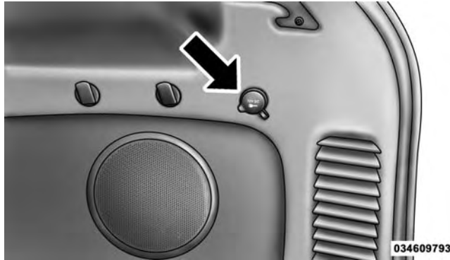
Rear Power Outlet
