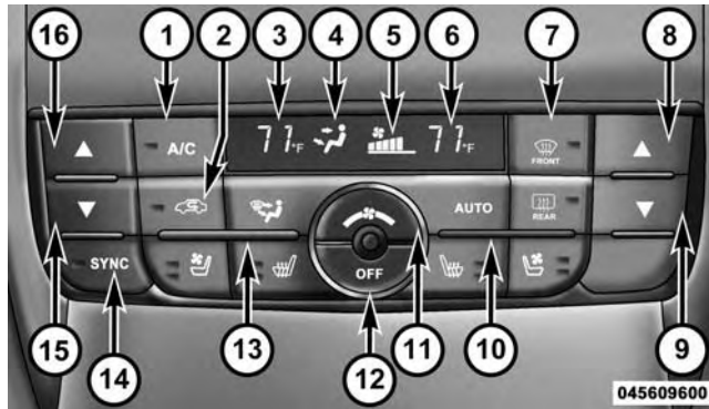
Automatic Temperature Control (ATC) Panel
