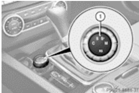
Drive program selector with manual drive program
