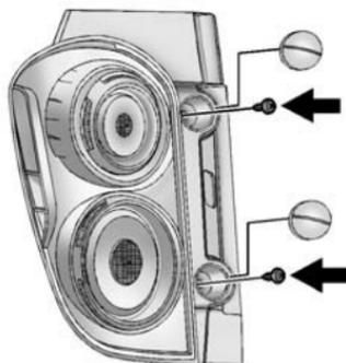
3. Remove the two screws securing the taillamp assembly.
