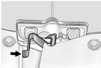
2. Go to the front of the vehicle to find the secondary hood release handle. The handle is under the front edge of the hood near the center. Push the handle to the right and at the same time raise the hood.
