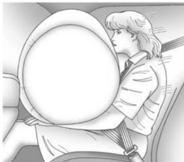
The front outboard passenger frontal airbag is in the instrument panel on the passenger side.
