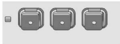
If equipped, these buttons are in the overhead console. The system can replace up to three remote control transmitters used to activate
