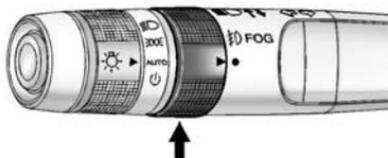
For vehicles with fog lamps, the control is located on the turn signal lever.
