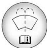
Open the cap with the washer symbol on it. Add washer fluid until the tank is full. See *Engine Compartment Overview* on page 10-5 for reservoir location.
