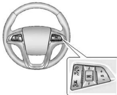
Some audio steering wheel controls can be adjusted at the steering wheel.
