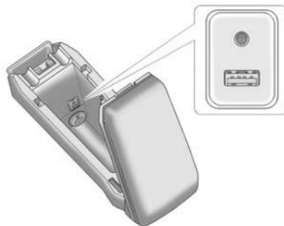
This jack is not an audio output. Do not plug headphones into the auxiliary input jack. Drivers are encouraged to set up any auxiliary device while the vehicle is in P (Park).
