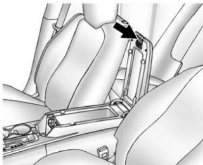
There is storage in the center console; lift the lever on the front to open. There may be a USB port and auxiliary input jack inside.
