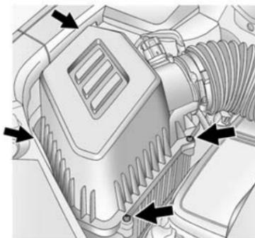
3. Remove the four air cleaner housing cover screws.
