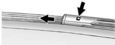
2. Press the square button on the top side, at the end of the wiper arm, and pull the wiper blade out of the end of the wiper arm.
