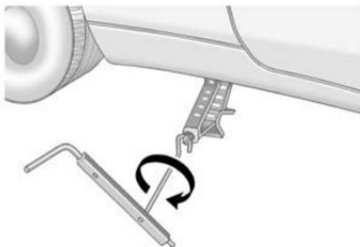
8. Raise the vehicle by turning the jack handle clockwise. Raise the vehicle far enough off the ground so there is enough room for the road tire to clear the ground.
