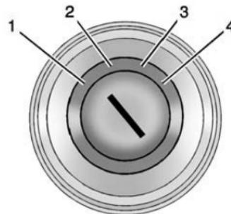
The ignition switch has four different positions.
