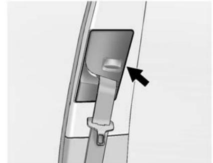
Move the height adjuster up to the desired position by pushing up on the height adjuster.
