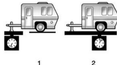
If a weight-carrying hitch or a weight-distributing hitch is being used, the trailer tongue (1) should weigh 10 to 15 percent of the total loaded trailer weight (2).
