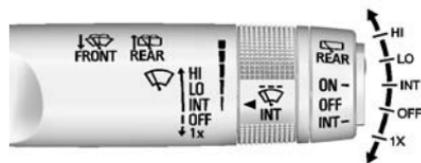
The windshield wiper/washer lever is located on the right side of the steering column. With the ignition in ACC/ACCESSORY or ON/RUN/START, move the windshield wiper lever to select the wiper speed.
