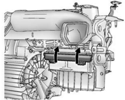
6. Push the two tabs upward and release the latches holding the service door. Lift the service door.
