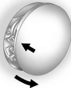
The fuel cap is behind the fuel door on the passenger side of the vehicle. To open the fuel door, push and release the rearward center edge of the door.
