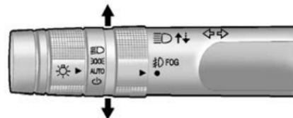
Move the lever all the way up or down to signal a turn.
