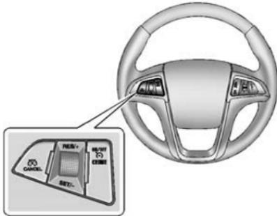
**CRUISE** : Press to turn the cruise control system on and off.
