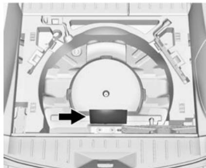
1. Remove the cable package. The cable is stored in a plastic bag under the compact spare tire.
