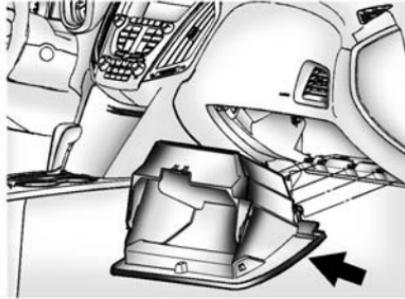
2. Push the stop tab upward until the stop tab is under the instrument panel assembly and the glove box is released.
