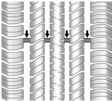
Treadwear indicators are one way to tell when it is time for new tires. Treadwear indicators appear when the tires have only 1.6 mm (1/16 in) or less of tread remaining. See *Tire Inspection* on page 10-49 and *Tire Rotation* on page 10-49.
