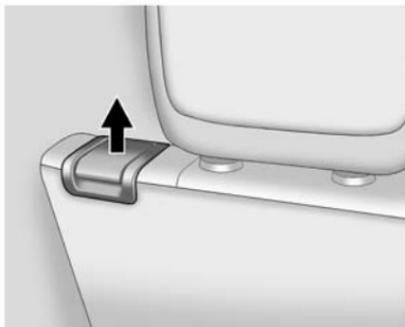
2. Lift the lever on the top of the seatback.
