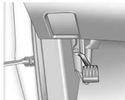
To set the parking brake, hold the regular brake pedal down, then push the parking brake pedal down. If the ignition is on, the brake system warning light will come on. See *Brake System Warning Light* on page 5-16.
