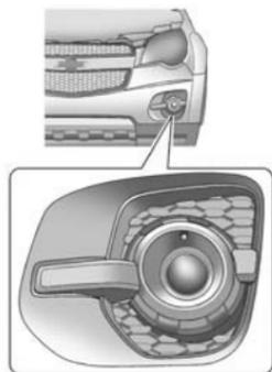
1. Locate the fog lamp assembly under the front fascia.
