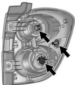
6. Turn the bulb socket counterclockwise and pull it out.
