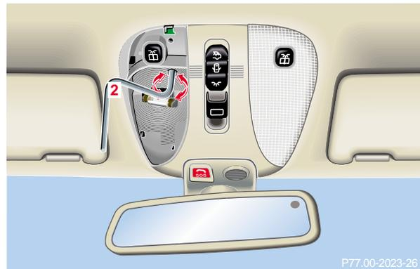
Obtain crank (2) (supplied with vehicle) and insert through hole.
