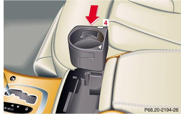
Press button (4) to unlock cup holder and fold into the storage compartment until it engages.
