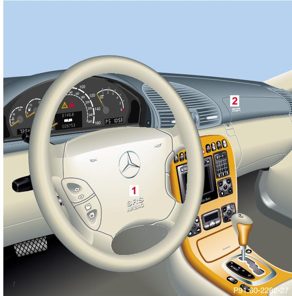
**1** Driver airbag**2** Front passenger airbag
