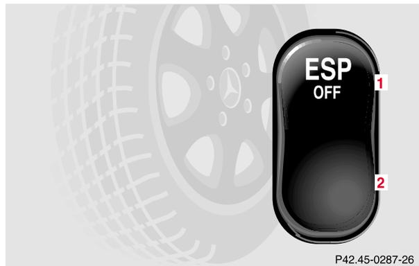
ESP control switch located on center console.
