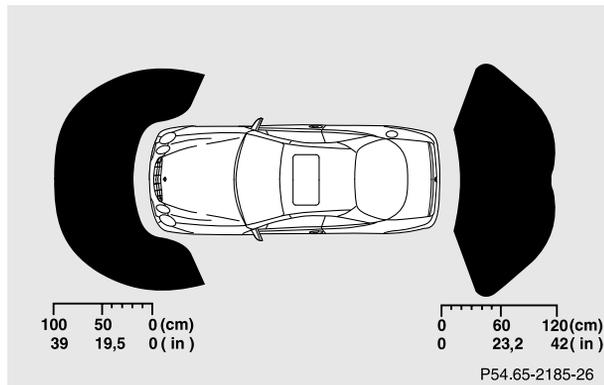
The first yellow segment lights up at these distances. Additional segments light up as the vehicle comes closer to the obstacle.
