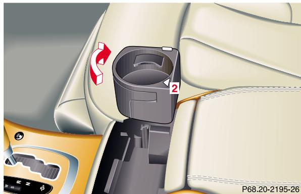
Press button (2) to open the second cup holder. The cup holder opens automatically.
