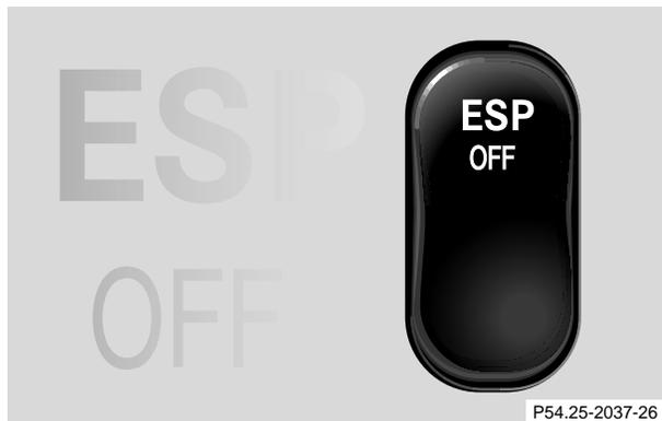
ESP control switch located on center console.
