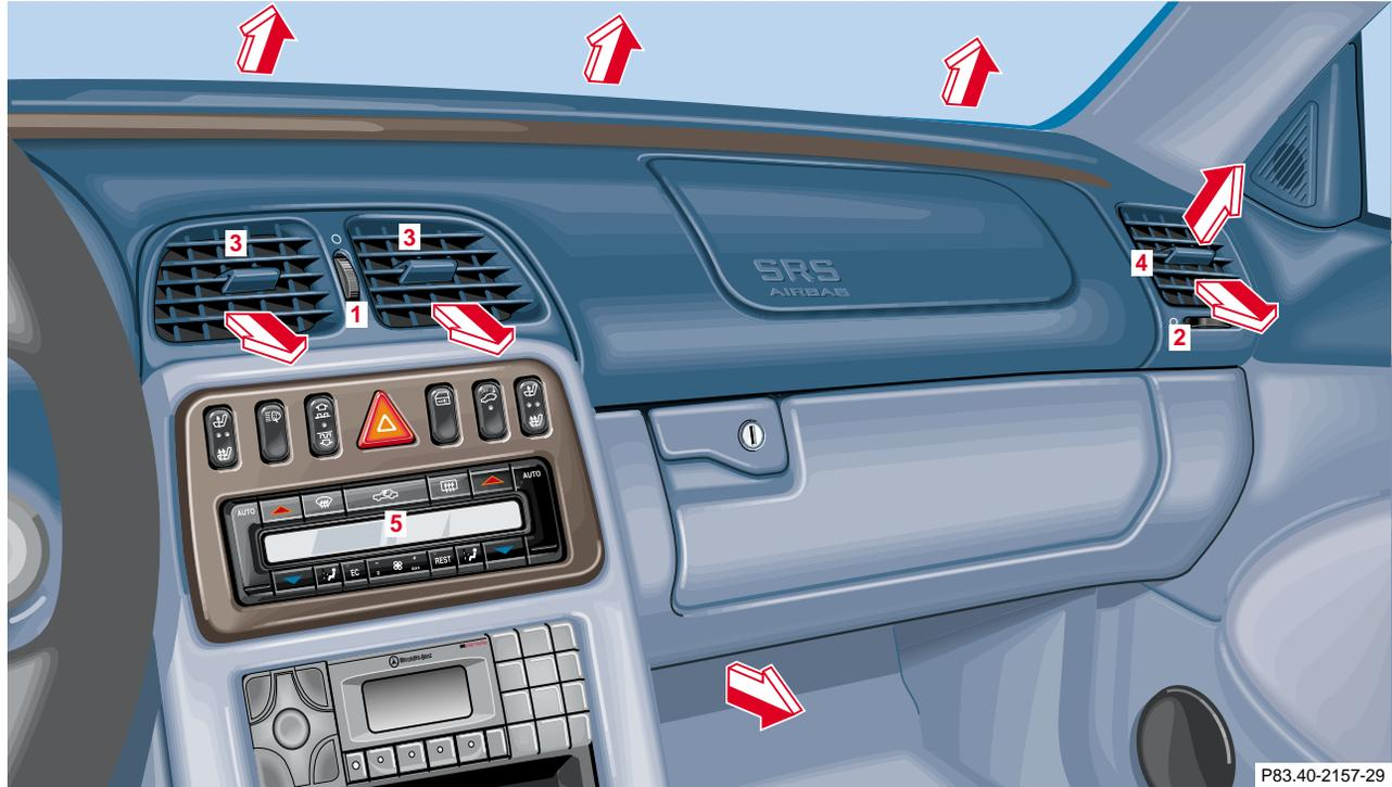
**1** Air volume control for center air outlets, turn wheel up to open.
