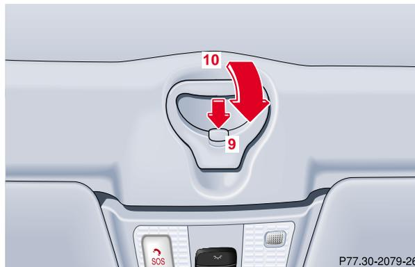
18. Press lock button (9) and fold down locking handle (10).
