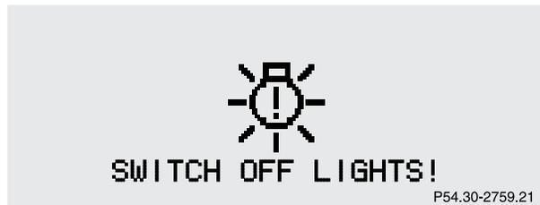
With the electronic key removed and the driver's door open, a warning sounds and the message "SWITCH OFF LIGHTS!" appears in the multifunction indicator if the vehicle's exterior lamps (except standing lamps) are not switched off.
