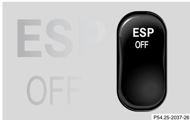
ESP control switch located on center console.
