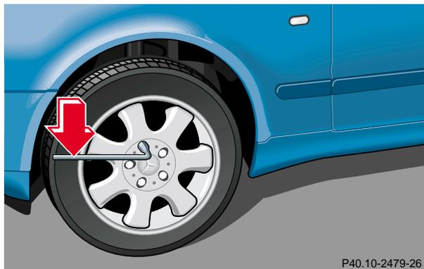
4. Using the wrench, loosen but do not yet remove the wheel bolts.
