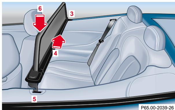
3. Insert end section in right opening (3) on quarter panel first. Then push left end section toward vehicle center (arrow 4) until it meets the left opening. Insert end section in left opening (5).
