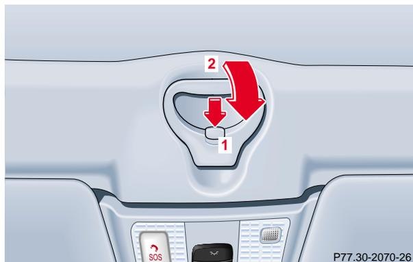
5. Press lock button (1) and fold down locking handle (2).
