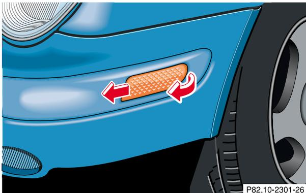
Carefully slide lamp towards front (arrow), and remove back and first.
