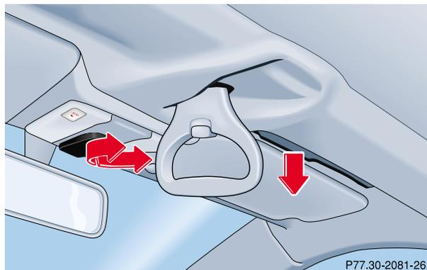
19. Turn locking handle 90° clockwise and pull soft top frame carefully down until it meets the windshield header attachment points.
