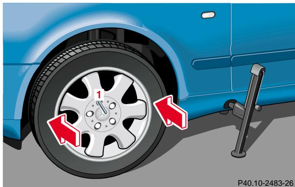
10. Clean contact surfaces of wheel and wheel hub. Install wheel on wheel hub. Insert wheel bolts and tighten them slightly.
