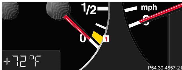
When the warning lamp (1) comes on after starting the engine, or if it comes on while driving, it indicates that the fuel level is down to the reserve quantity of approximately 2.1 gal (8 liters).
