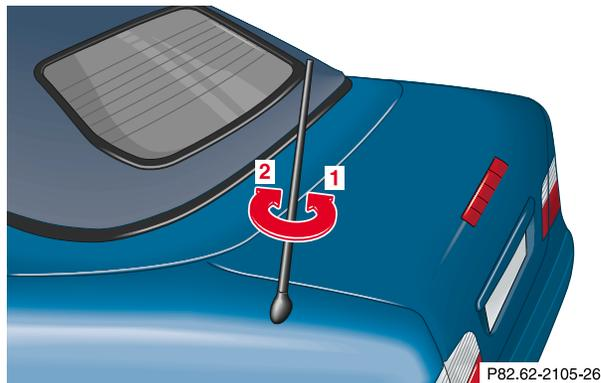
The non-retractable antenna should be removed before entering an automatic car wash, to avoid damage to the antenna mast or vehicle paint finish.
