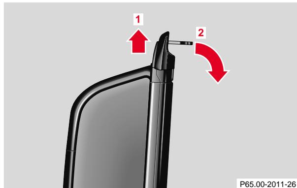
Pull end sections in direction of arrow (1) and fold in direction of arrow (2).
