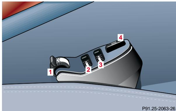
Some models may be equipped with multicontour seats. These seats have movable seat cushions, and inflatable air cushions built into the backrest to provide additional lumbar and side support.
