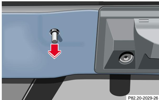
If the trunk is to remain open for a long period of time, the trunk lamp can be switched off by pulling out the plunger in the switch (arrow). This prevents the vehicle battery from being discharged.
