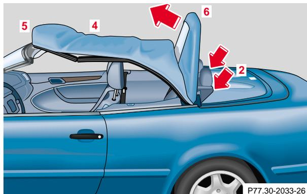
9. Do not place soft top frame (5) onto windshield header.
