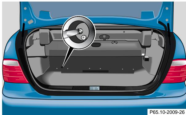
16. Using screwdriver (supplied in vehicle tool kit), turn screw clockwise to the stop.
