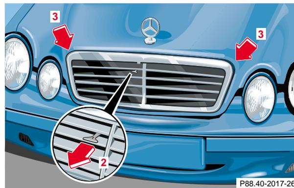
Pull handle (2) to its stop out of radiator grill and open hood (do not pull up on handle).
