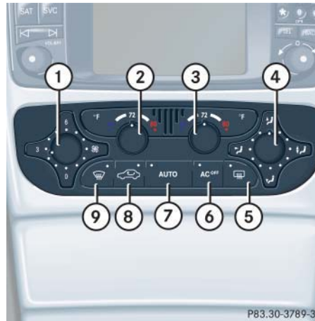
Climate control panel
