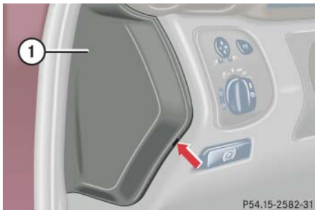
① Main fuse box cover
