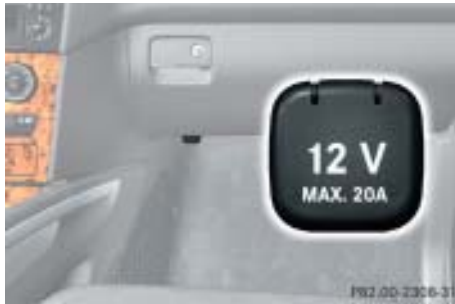
Power outlet in front passenger footwell
