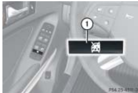
① Override switch
