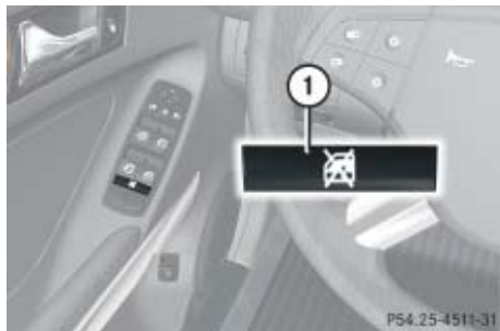
① Override switch
