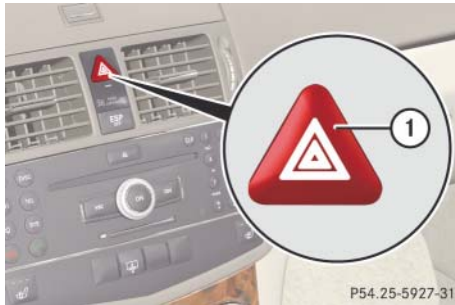
① Hazard warning flasher switch
