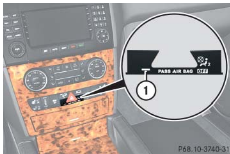
① Alarm system indicator lamp
