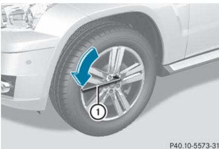
► Using lug wrench ①, loosen the bolts on the wheel you wish to change by about one
