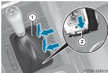
**!** Do not use any sharp-edged objects to remove the selector lever cover in the center console. This can damage the selector lever cover.
