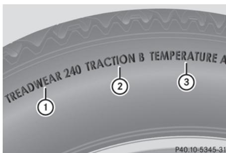
The Uniform Tire Quality Grading Standards are U.S. government specifications. Their purpose is to provide drivers with uniform reliable information on tire performance data. Tire manufacturers have to grade tires using three performance factors: ① tread wear, ② tire traction, and ③ heat resistance. All tires sold in North America are provided with the corresponding quality class mark on the sidewall of the tire, even though these regulations do not apply to Canada.
