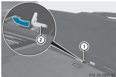
**!** The tailgate swings upwards and to the rear when opened. Therefore, make sure that there is sufficient clearance above and behind the tailgate.
