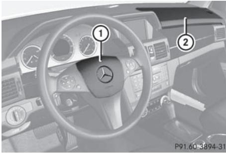
Driver's air bag ① deploys in front of the steering wheel; front-passenger air bag ② deploys in front of and above the glove box. They are deployed:
