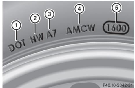
The TIN is a unique identification number. The TIN enables the tire manufacturers to inform purchasers of recalls and other safety-relevant matters. It makes it possible for the purchaser to easily identify the affected tires. The TIN is made up of manufacturer identification code ②, tire size ③, tire type code ④ and date of manufacture ⑤.
