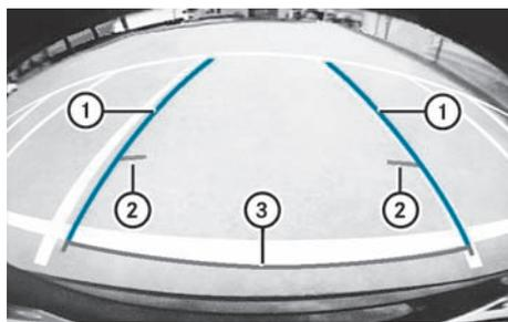
Guide lines ② and ③ show the approximate distance from the rear of the vehicle. Yellow guide line ② indicates a distance of approximately 3 ft (1 m) and red guide line ③ indicates a distance of approximately 10 in (0.25 m). The distances only apply to objects at ground level. Blue guide line ① depicts the width required for the vehicle. It is used to align the vehicle with the edge of the road, e.g. the curb.
