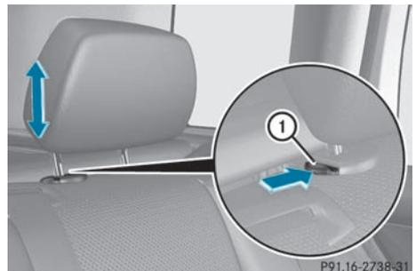
If the head restraint is fully lowered, it is necessary to press release catch ①.
