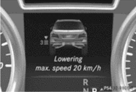
If you maintain or reduce your speed, you will see a message in white in the display while the vehicle is being lowered, such as the following: **Lowering Max. speed 20 km/h**
