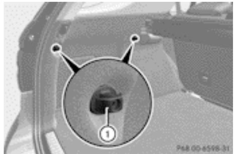
There are two securing hooks (1) on each side of the luggage compartment.
