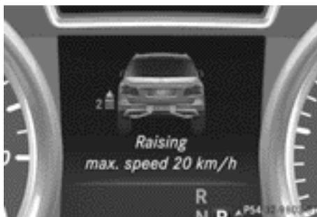
While the adjustment from off-road level 2 to off-road level 3 is taking place, you will see a message such as the following in the multifunction display: **Vehicle rising**
