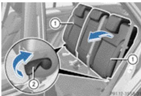
You can adjust the angle of the backrests in the second row of seats. There are ten detent positions.
