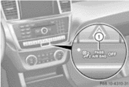
The front-passenger seat sensor system for child restraint systems detects whether a special Mercedes-Benz child seat with a transponder for automatic child seat recognition has been fitted. In this case,
