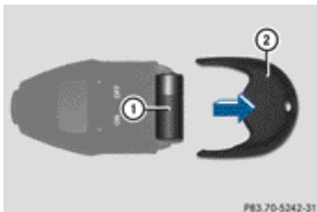
One 6 V pin battery, type 2CR11108 is required.
