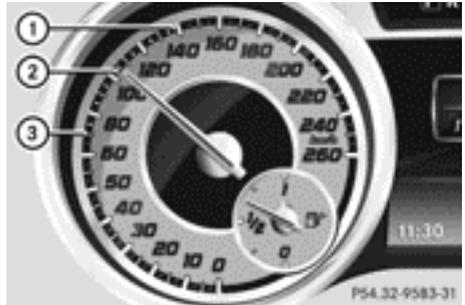
Example: DISTRONIC PLUS displays in the speedometer
