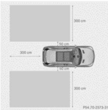
The Blind Spot Assist monitors the area up to 3.0 m behind your vehicle and directly next to your vehicle, as shown in the diagram.
