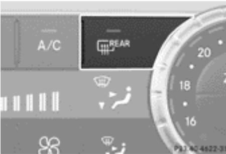
The rear window heating has a high current draw. You should therefore switch it off as soon as the window is clear. It otherwise switches off automatically after several minutes.
