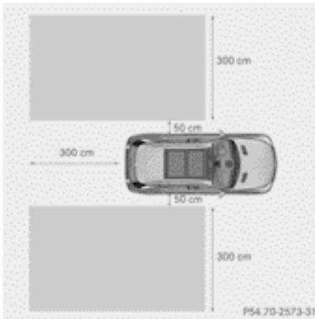
Active Blind Spot Assist monitors the area up to 3.0 m behind your vehicle and directly next to your vehicle, as shown in the diagram. For this purpose, Active Blind Spot Assist uses radar sensors in the rear bumper.
