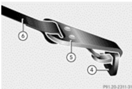
Top Tether provides an additional connection between the child restraint system secured with ISOFIX and the rear seat. It helps reduce the risk of injury even further.
