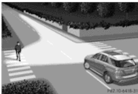
The cornering light function improves the illumination of the road over a wide angle in the direction you are turning, enabling better visibility in tight bends, for example. It can only be activated when the dipped-beam headlamps are switched on.
