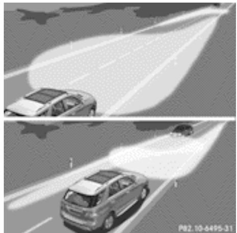
You can use this function to set the headlamps to change between dipped beam and main beam automatically. The system recognises vehicles with their lights on, either approaching from the opposite direction or travelling in front of your vehicle, and conse-
