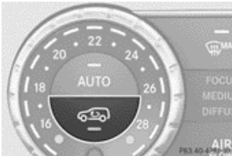
You can deactivate the flow of fresh air if unpleasant odours are entering the vehicle from outside. The air already inside the vehicle will then be recirculated.
