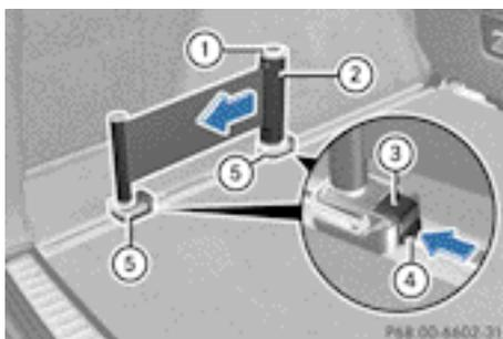
The luggage holder can be used to secure light loads against the side wall of the luggage compartment to prevent them from moving around.
