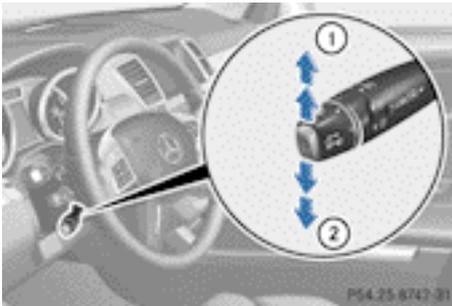
You can use the cruise control lever to limit the speed to any speed above 30 km/h while the engine is running.
