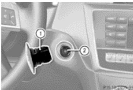
You can remove the Start/Stop button from the ignition lock and start the vehicle as normal using the key.
