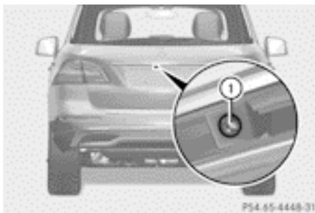
Reversing camera ① is in the handle on the tailgate.
