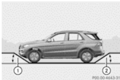
The table shows approach and departure angles ① and ② when the vehicle is loaded and ready to drive.
