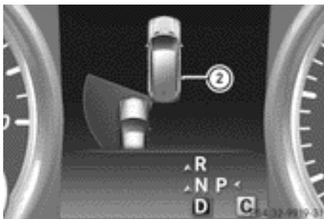
If Active Blind Spot Assist detects a risk of a lateral collision in the monitoring range, a course-correcting brake application is carried out. This is designed to help you avoid a collision.
