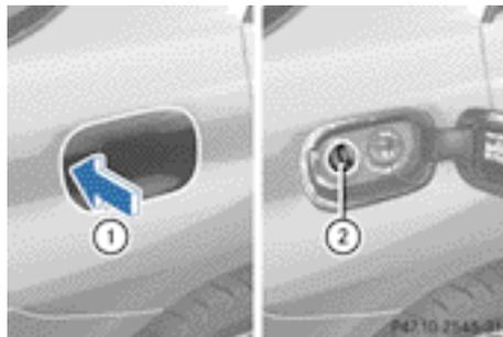
The fuel filler flap is unlocked or locked automatically when you open or close the vehicle with the key or using KEYLESS-GO.
