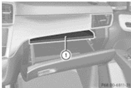
Partition ① for stowing flat objects is located in the upper section of the glove compartment. It can be removed to increase the stowage space in the glove compartment.
