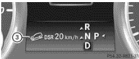
► **To increase or reduce the set speed in 1 km/h increments:** briefly press the cruise control lever, up ① for a higher set speed or down ② for a lower set speed. The set speed appears in the multifunction display with the
