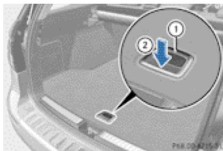
A removable insert under the luggage compartment floor contains the parts of the EASY-PACK load-securing kit. TIREFIT and the tyre-change tool kit, etc. are stored beneath this insert.
