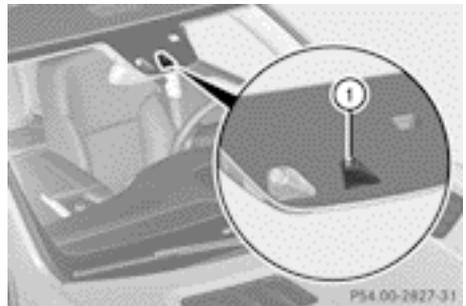
Active Lane Keeping Assist monitors the area in front of your vehicle by means of camera ① at the top of the windscreen. Active Lane Keeping Assist detects lane markings on the road and warns you before you leave your lane unintentionally. If you do not react to the warning, a lane-correcting application of the brakes can bring the vehicle back into the original lane.
