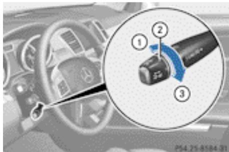
You can set the specified minimum distance for DISTRONIC PLUS by varying the time span between one and two seconds. With this function, you can set the minimum distance that DISTRONIC PLUS keeps to the vehicle in front, dependent on vehicle speed. You can see this distance in the multifunction display (▷ page 209).
