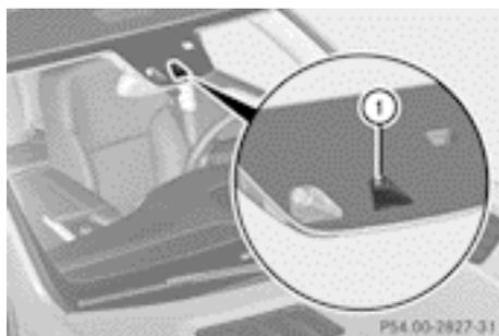
Speed Limit Assist detects the traffic signs with camera ① attached at the top of the windscreen.
