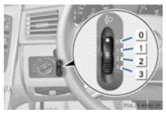
Headlamp range control (vehicles with steel suspension)
