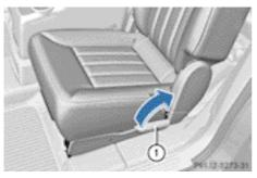
The release handle for the EASY-ENTRY feature is located on the entry side on the back of each outer seat in the 2nd row of seats.
