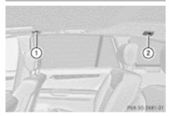
The safety net can be used in two different positions (behind the B-pillar or the C-pillar).
