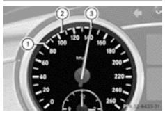
When DISTRONIC is activated, one or two segments in the set speed range light up.
