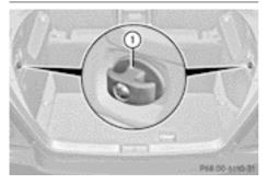
There is a mounting hook ① on each of the side panels in the luggage compartment. Only secure lightweight luggage items on the mounting hooks (maximum 4 kg).
