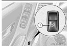
You can open and close the tailgate from the driver's seat when the vehicle is stationary and unlocked.
