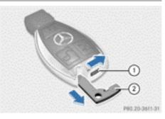
Push release catch ① in the direction of the arrow and at the same time, remove emergency key element ② from the key.
