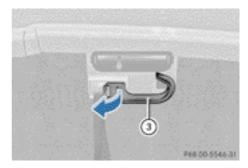
► Fold out hook ③ on the underside of the luggage compartment floor.
