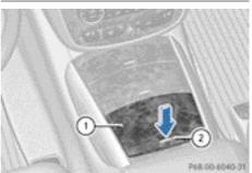
► To open: briefly press trim ② in the direction of the arrow. Cover ① swings upwards.
