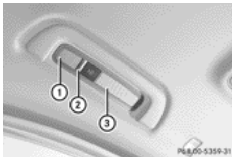
Rear-compartment overhead control panel
