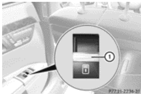
Door control panel in rear
