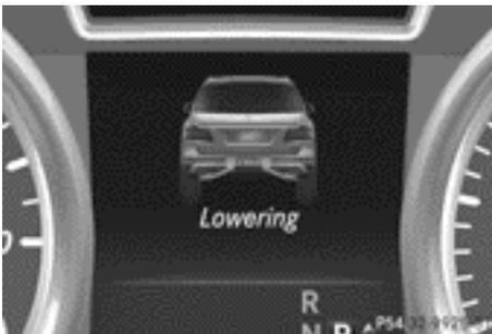
During the adjustment, the **Being Lowered** message, for example, appears in the multifunction display.
