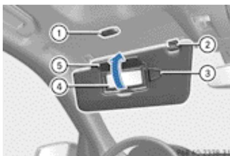
Mirror light ① only functions if the sun visor is clipped into retainer ② and mirror cover ⑤ has been folded up.
