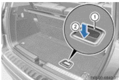
The TIREFIT kit, tire-change tool kit, etc. are located in the stowage compartment.
