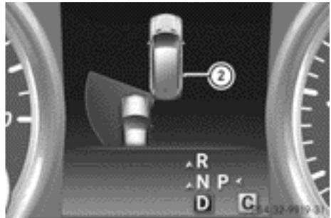
If Active Blind Spot Assist detects a risk of a lateral collision in the monitoring range, a course-correcting brake application is carried out. This is meant to assist you in avoiding a collision.
