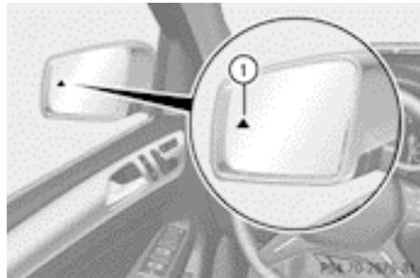
When you switch on the turn signals to change lanes and a vehicle is detected in the side monitoring range, you receive a visual and acoustic collision warning. You then hear a double warning tone and red warning lamp ① flashes. If the turn signal remains on, detected vehicles are indicated by the flashing of red warning lamp ①. There are no further warning tones.
