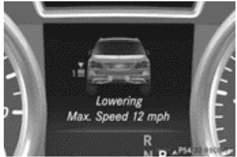
During the adjustment, the **Vehicle Lowering** message, for example, appears in the multifunction display.
