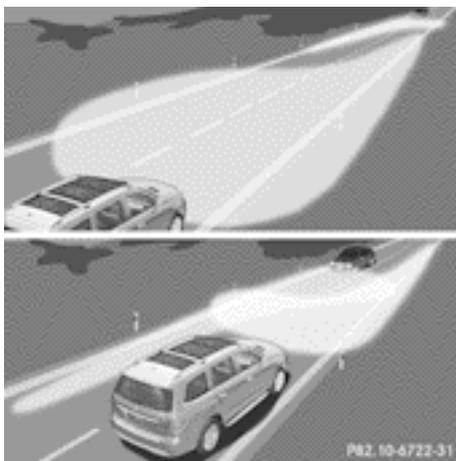
You can use this function to set the headlamps to change between low beam and high beam automatically. The system recognizes vehicles with their lights on, either
