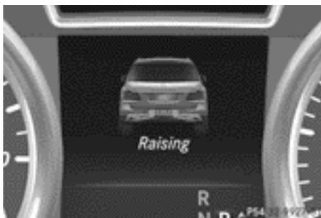
During the adjustment, the **Vehicle Rising** message, for example, appears in the multifunction display.
