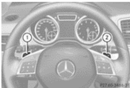
In the manual drive program you can change gears manually using steering wheel paddle shifters ① and ② (▷ page 171).
