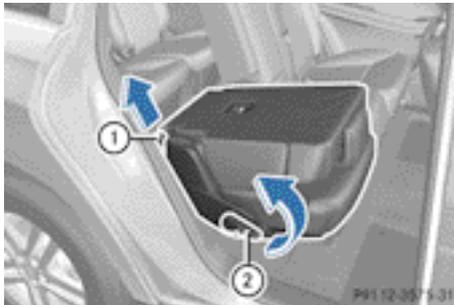
The release handle for the EASY-ENTRY/EXIT feature is located on the entry side on the back of each outer seat in the 2nd row of seats.
