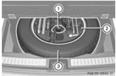
Emergency spare wheel (example: vehicle without lockable cargo compartment floor)
