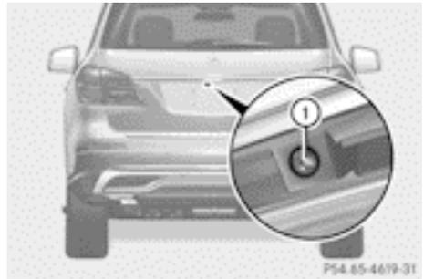
Rear view camera ① is in the handle on the tailgate.
