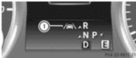
► Switch on Active Lane Keeping Assist using the on-board computer; to do so, select **Standard** or **Adaptive** (► page 275). Symbol ① appears in the multifunction display.
