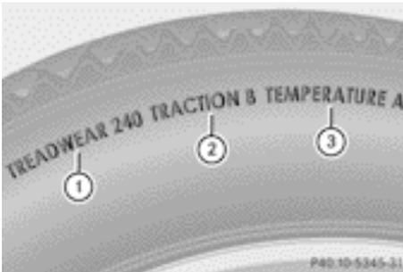
Uniform Tire Quality Grading Standards are U.S. government specifications. Their purpose is to provide drivers with uniform reliable information on tire performance data. Tire manufacturers have to grade tires using three performance factors: ① tread wear grade, ② traction grade and ③ temperature grade. These regulations do not apply to Canada. Nevertheless, all tires sold in North America are provided with the corresponding
