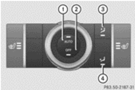
Rear-compartment control panel only in combination with special equipment seat heating
