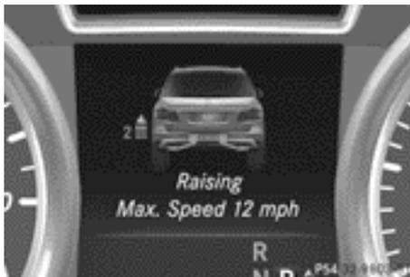
While the adjustment from off-road level 2 to off-road level 3 is taking place, you will see a message such as the following in the multifunction display: **Vehicle Rising Max. Speed 12 mph (20 km/h).**
