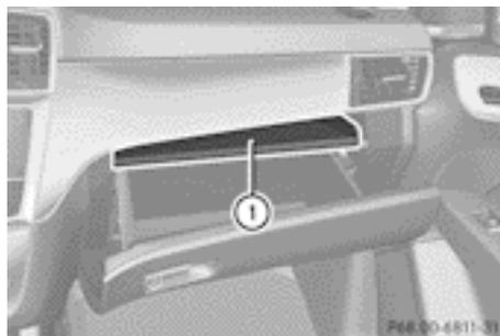
Partition ① for stowing flat objects is located in the upper section of the glove box. It can be removed to increase the stowage space in the glove box.
