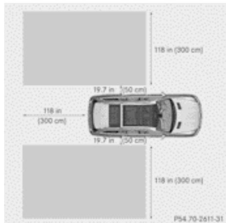
Active Blind Spot Assist monitors the area up to 10 ft (3.0 m) behind your vehicle and directly next to your vehicle, as shown in the diagram. For this purpose, Active Blind Spot Assist uses radar sensors in the rear bumper. If the lanes are narrow, vehicles driving in the lane beyond the lane next to your vehicle may be indicated, especially if the vehicles are not driving in the middle of their lane. This may
