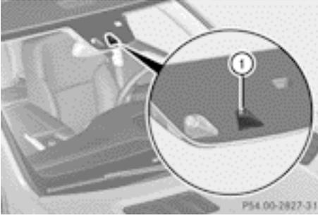
Active Lane Keeping Assist monitors the area in front of your vehicle by means of a camera ① at the top of the windshield. Active Lane Keeping Assist detects lane markings on the road and warns you before you leave your lane unintentionally. If you do not react to the warning, a lane-correcting application of the brakes can bring the vehicle back into the original lane.
