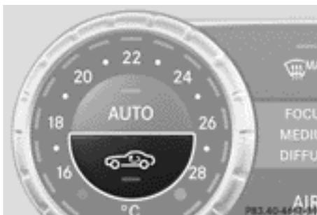
You can deactivate the flow of fresh air if unpleasant odors are entering the vehicle from outside. The air already inside the vehicle will then be recirculated.
