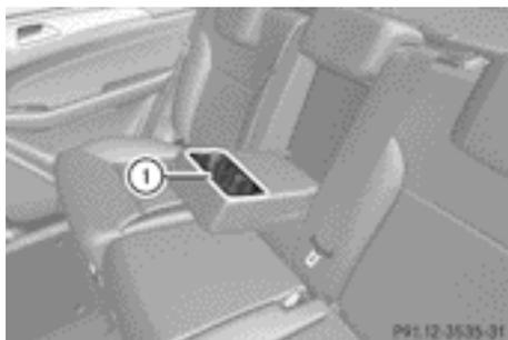
► Fold down the rear seat armrest. Cup holder ① is located in the rear seat armrest.
