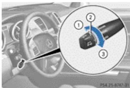
You can set the specified minimum distance for DISTRONIC PLUS by varying the time span between one and two seconds. With this function, you can set the minimum distance that DISTRONIC PLUS keeps to the vehicle in front, dependent on vehicle speed. You can see this distance in the multifunction display (▷ page 201).
