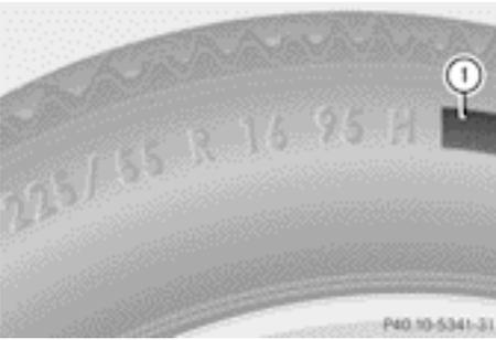
In addition to the load bearing index, load index ① may be imprinted after the letters that identify the speed index ⑥ on the sidewall of the tire (▷ page 411).
