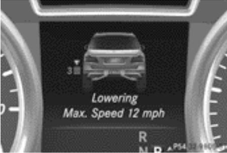
If you maintain or reduce your speed, you will see a message in white in the display while the vehicle is being lowered, such as the following: **Lowering Max. Speed 12 mph (20 km/h)**
