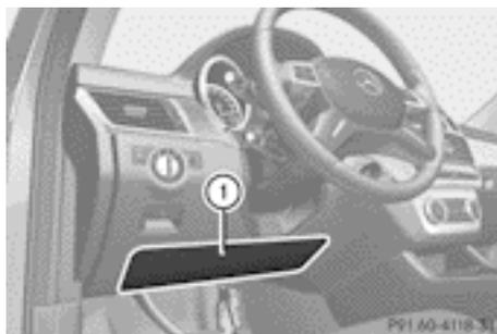
Driver's knee bag ① deploys under the steering column. The driver's knee bag is always deployed along with the driver's front air bag. The driver's knee bag is designed to operate together with the front air bags in frontal impacts if certain thresholds are exceeded. The driver's knee bag operates best in conjunction with correctly positioned and fastened seat belts.
