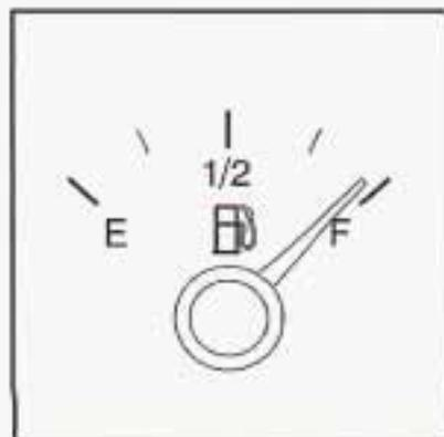
Your fuel gage shows about how much fuel is in your tank. The gage works only when the ignition switch is in the RUN position.
