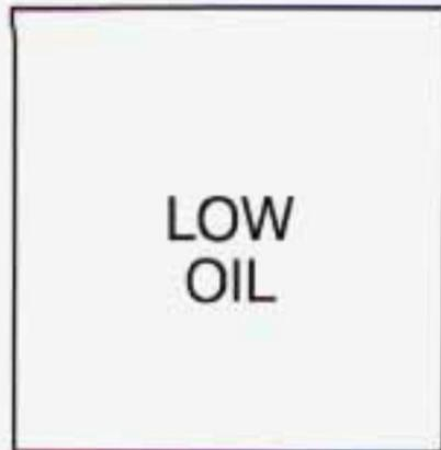
Your vehicle is equipped with an oil level monitoring system. When you start your engine, the warning light will come on briefly. If the light doesn't come on, have it repaired.
