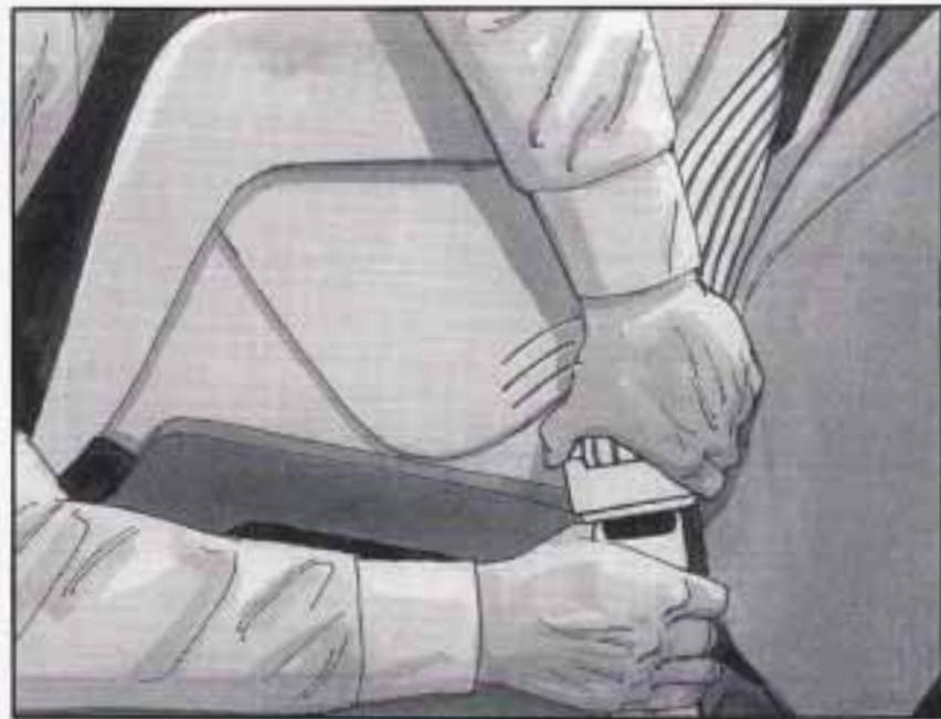
5. Tilt the latch plate to adjust the belt if needed.
