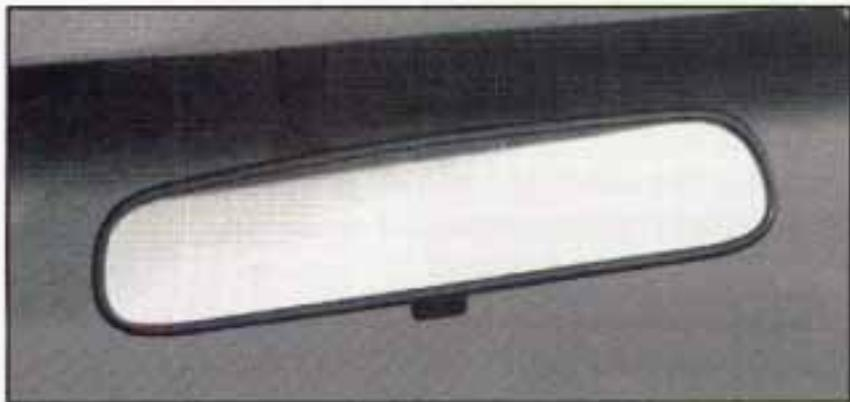
An inside rearview mirror is attached to your windshield. The mirror has pivots so that you can adjust it.
