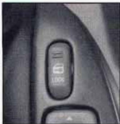
Push the power door lock switch to lock or unlock both doors at once.
