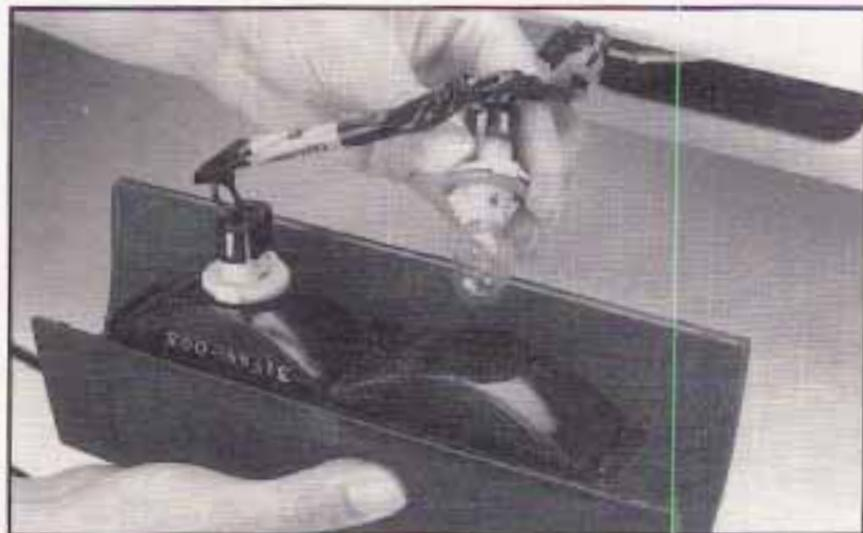
2. Gently pull the assembly out and remove the bulb from the back of the assembly.
