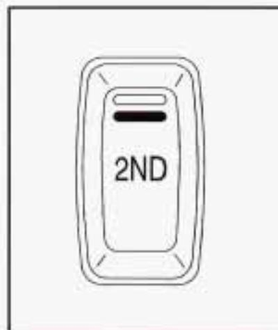
Your vehicle may be equipped with a second-gear start feature. Press **2ND GEAR START** to provide more traction when you are starting on ice or other slippery surfaces. A light on the switch will illuminate when the 2nd gear start is selected. The transmission will be in **SECOND (2)** gear when the vehicle begins to move. After starting in **SECOND (2)** gear, the vehicle will upshift normally.
