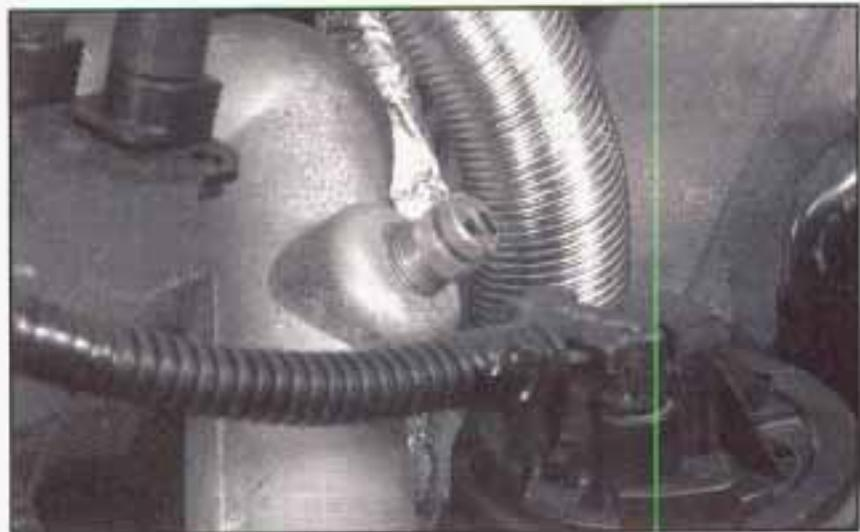
3. After the engine cools, open the coolant air bleed valve.
