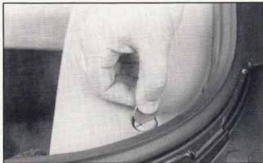
Find the plastic screw heads in the trim panel over the spare tire. (See "Compact Spare Tire" later in this section for more information about the compact spare.) Use a coin or a key to turn the screw heads until the slots point front and back. Gently lift the trim panel and move it out of the way.
