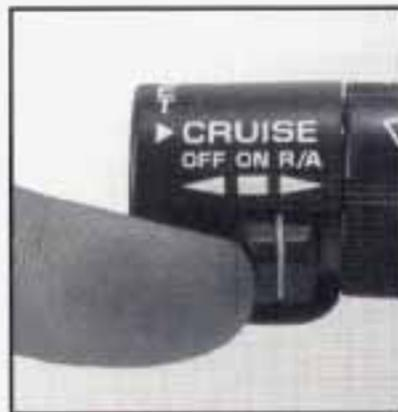
Suppose you set your cruise control at a desired speed and then apply the brake or clutch pedal. This, of course, shuts off the cruise control. But you don't need to reset it. Once you're going about 25 mph (40 km/h) or more, you can move the cruise control switch from ON to R/A (Resume/Accelerate) for about half a second.
