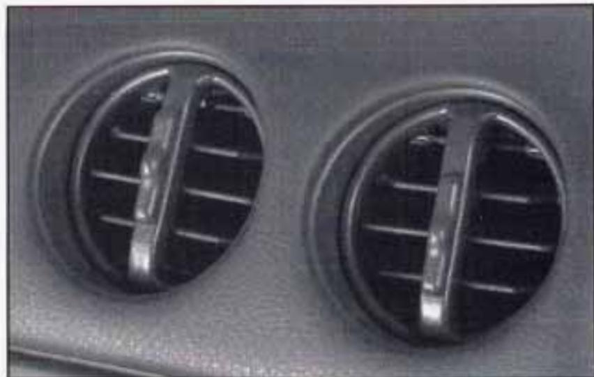
Your Pontiac's flow-through ventilation system supplies outside air into the vehicle when it is moving. Outside air will also enter the vehicle when the blower fan is running.
