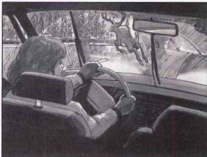
You can steer around the obstacle while braking hard. As you brake, your computer keeps receiving updates on wheel speed and controls braking pressure accordingly. Remember: Anti-lock doesn't change the time you need to get your foot up to the brake pedal or always decrease
