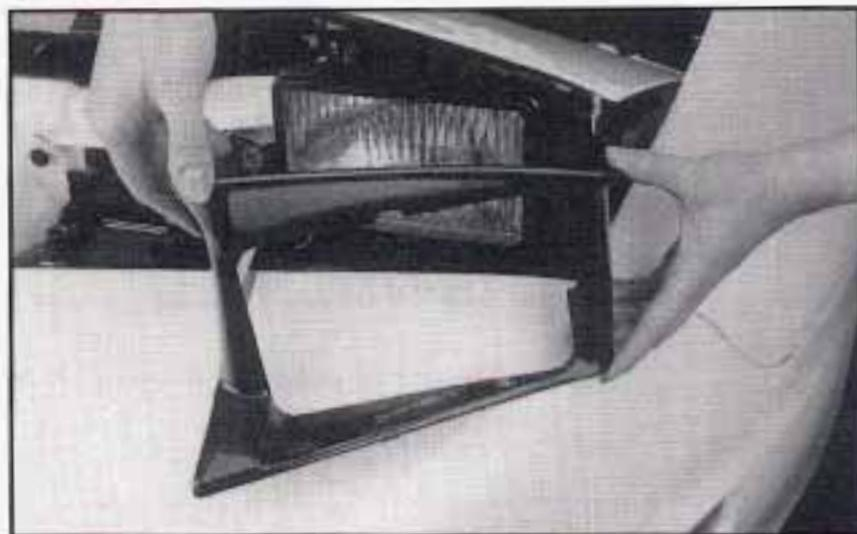
2. Unscrew the bezel with a screwdriver and remove it.
