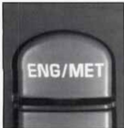
Push the ENG/MET button on the trip calculator to switch the HUD speed display from English to metric or metric to English. If you don't have the trip calculator, you can't change the display.
