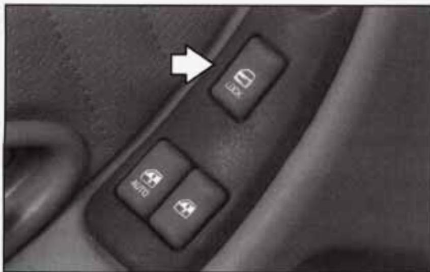
To unlock all doors from inside the vehicle, press the front of the power door lock switch on either front door. If your vehicle is equipped with a Content Theft-Deterrent system, the power door lock switch will not unlock the doors until the system is disarmed. See “Content Theft-Deterrent” in the Index for more details.
