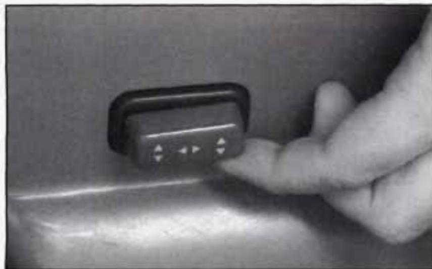
This switch is designed to control the movements of your seat cushion. It is located on the left side of the driver's seat cushion. To move the seat forward or rearward, push the switch forward or rearward. To raise or lower the seat, push the switch up or down. To raise or lower the front portion of your seat, push the front of the switch up or down. To raise or lower the rear portion of your seat, push the rear of the switch up or down.
