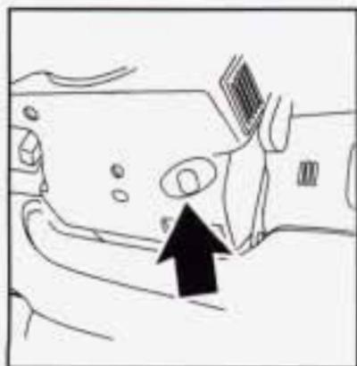
The first is located underneath the steering column below the lock cylinder.
