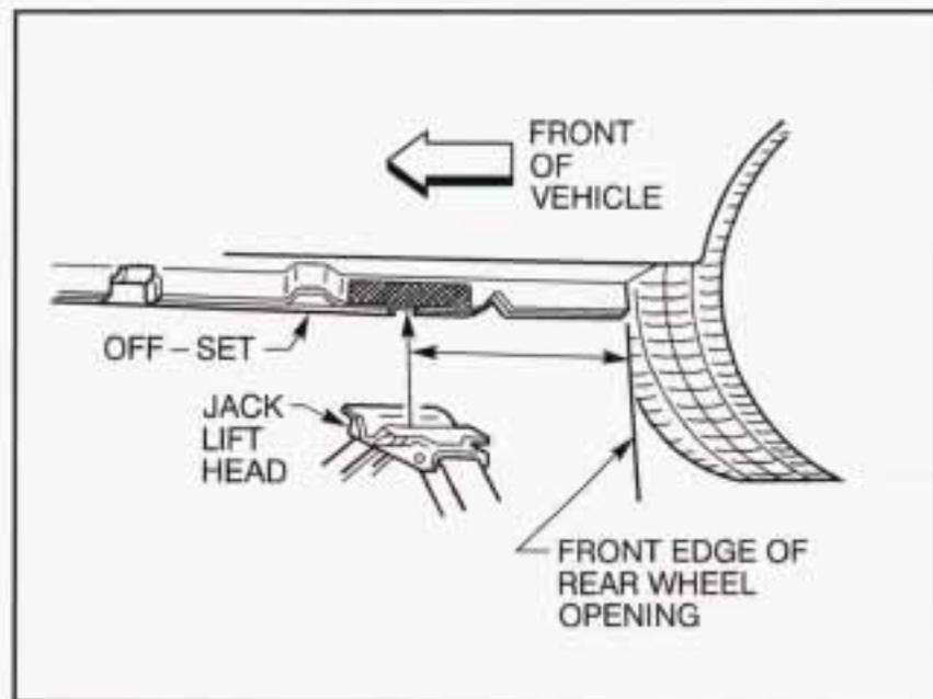
For jacking at the vehicle's rear location, put the jack lift head about 5.5 inches (14 cm) from the front edge of the rear wheel opening or just behind the off-set as shown.
