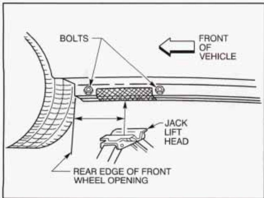
For jacking at the vehicle's front location, put jack lift about 6 inches (15 cm) from the rear edge of the front wheel opening or between the two bolts as shown.
