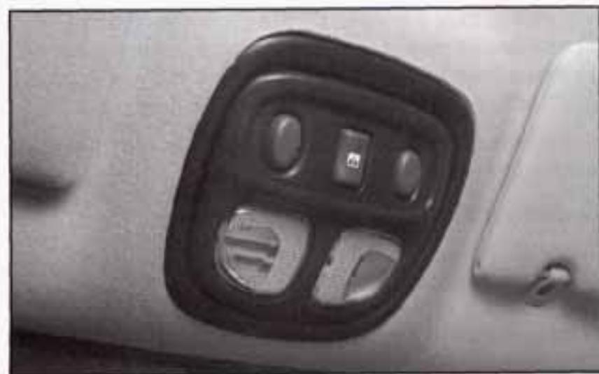
If your vehicle has the optional sunroof, you will have reading lamps in front of your sunroof switch. Press the button behind each reading lamp to turn them on and off.
