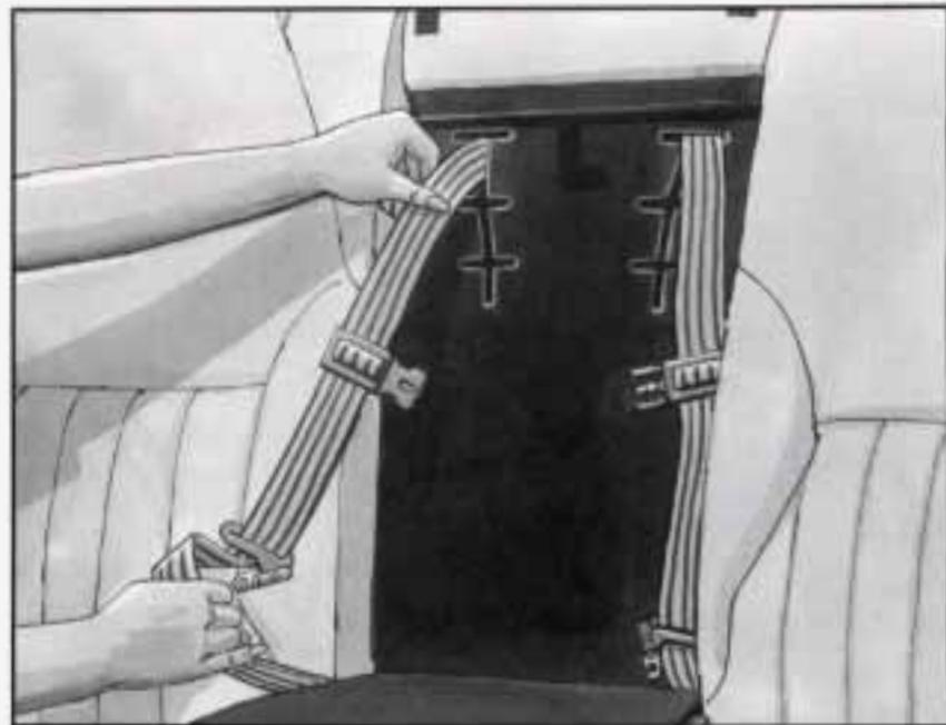
6. Feed a small amount of harness slack back into the slot.
