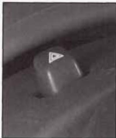
Press the switch on top of the steering column to make your front and rear turn signal lamps flash on and off. Your hazard warning flashers work no matter what position your key is in, and even if the key isn't in.
