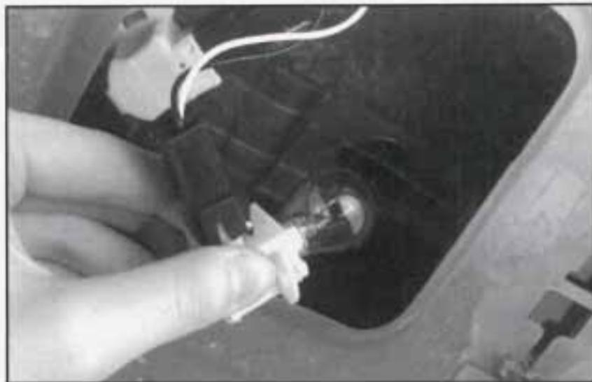
3. Remove the bulb by turning it a quarter of a turn counterclockwise.
