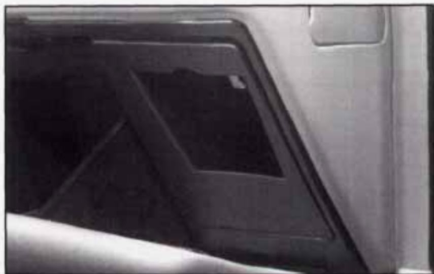
Some fuses are in a fuse block located inside of the glove box behind a small bin, on the right side. To open, pull on the plastic strap and pull the cover out. The fuse block is inside. On the back edge of this cover is a fuse puller and a fuse usage chart. To use the fuse puller, place the wide end of the fuse puller over the plastic end of the fuse. Squeeze the ends over the fuse and pull it out.
