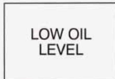
If the LOW OIL LEVEL light on the instrument panel comes on, it means you need to check *your* engine oil level right away.
