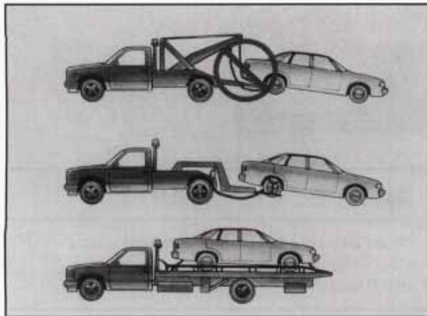
Use wheel-lift or car-carrier equipment. Additional ramping may be required for car-carrier equipment. Use safety chains and wheel straps. For rear towing, the parking brakes must be applied.
