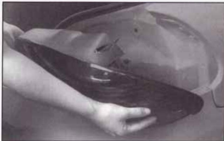
5. Carefully remove the taillamp assembly. Be careful to avoid scratching or chipping the paint on the vehicle.
