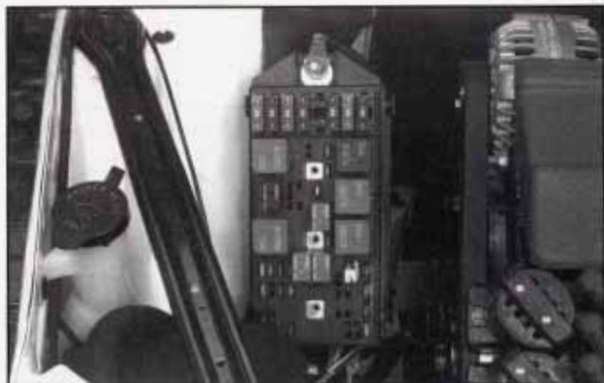
Some fuses are in a fuse block on the passenger's side of the engine compartment. Pull off the cover labeled FUSES to expose the fuses.
