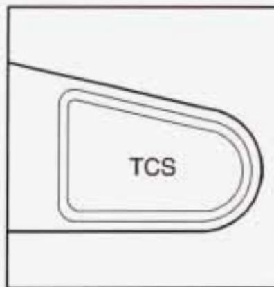
To turn the system off, press the TCS button on the far right end of the trip computer.
