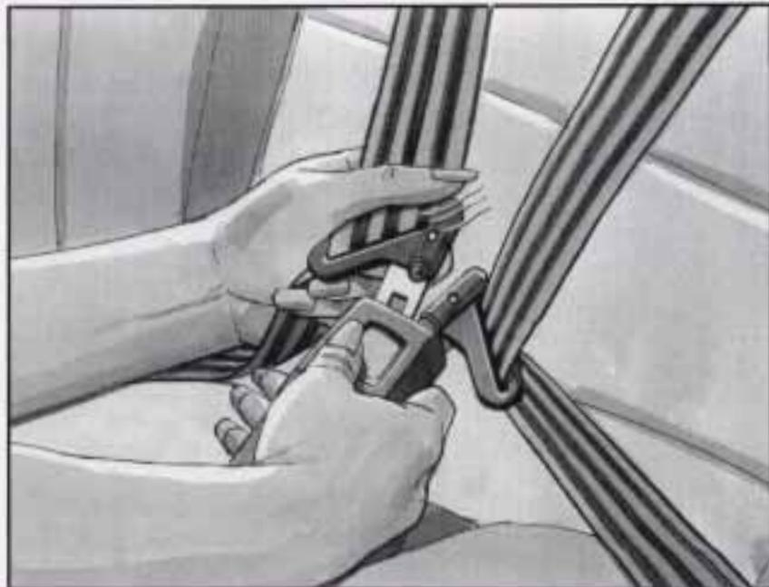
3. If the lap-shoulder harness is buckled, unlatch it by pushing the button on the buckle.
