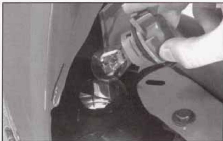
5. Remove the bulb from the socket.
