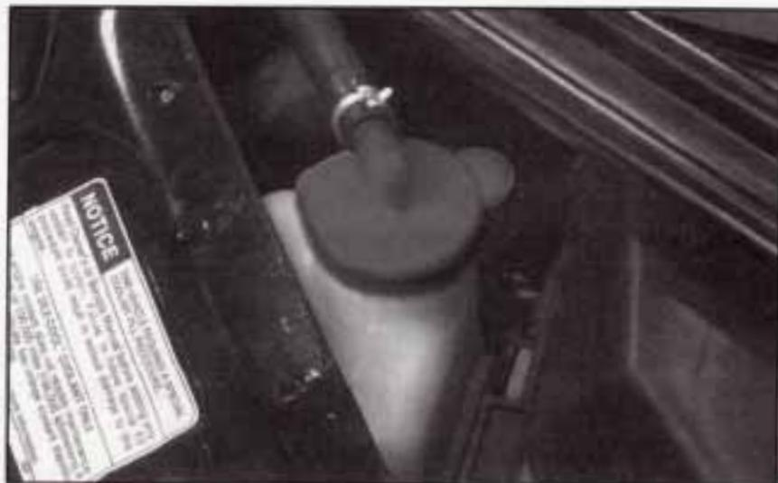
When your engine is cold, the coolant level should be at the COLD mark or a little higher. When your engine is warm, the level should be up to the HOT mark or a little higher.
