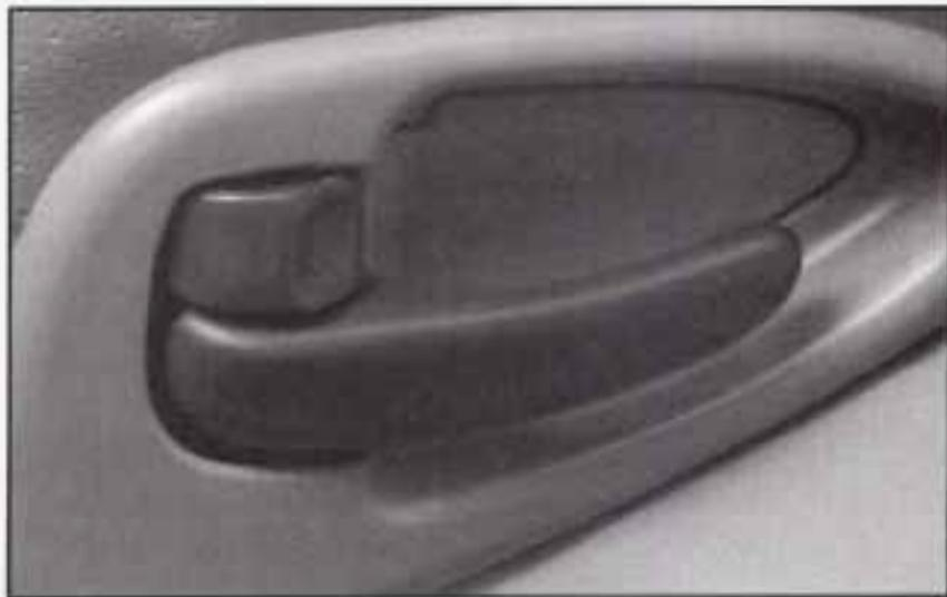
To unlock either front door from inside the vehicle, push the lock lever forward.
