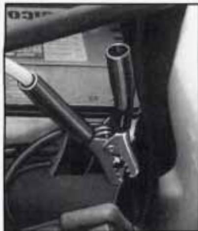
8. Now connect the black negative (-) cable to the good battery's negative (-) terminal. Don't let the other end touch anything until the next step. The other end of the negative (-) cable *doesn't* go to the dead battery.
