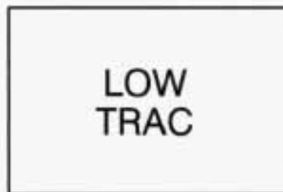
This light will come on when your traction control system is limiting wheel spin. See "Traction Control System Warning Light" in the index.
