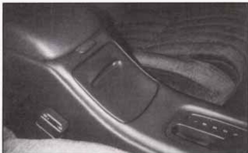
To open the armrest storage area, pull up on the front edge of the latch. The console has cassette and CD storage and a coinholder.
