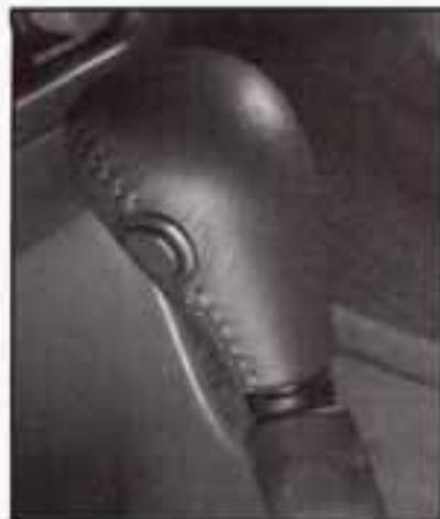
Press the performance shift button, located on the side of the console shift knob, to allow the transaxle to shift at higher engine speeds, increasing acceleration performance.
