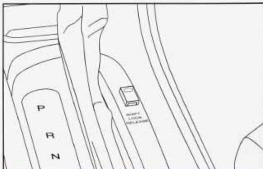
For vehicles with center console-mounted gear shift levers, the second access slot is located on the upper, right-hand side of the console shift panel. To use this slot:
