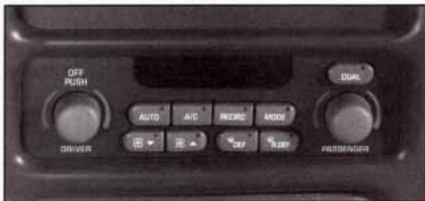
With this system, you set a "desired cabin" temperature. You can then either let the system automatically control airflow direction and amount (to maintain the desired cabin temperature) or you can manually adjust it. The system works best if you keep your windows closed while using it.
