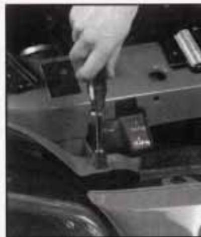
2. Remove the two bolts from the top of the headlamp assembly.
