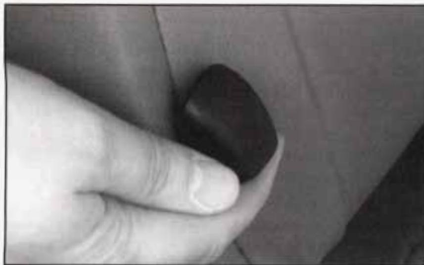
On two-door models, the right front seat is designed to make it easy to get in and out of the rear seat. Tilt the right seatback fully forward. The whole seat will now slide forward. If the seat will not tilt, lift the seatback latch, located on the back of the seat to tilt the seatback forward. The whole seat will now slide forward.
