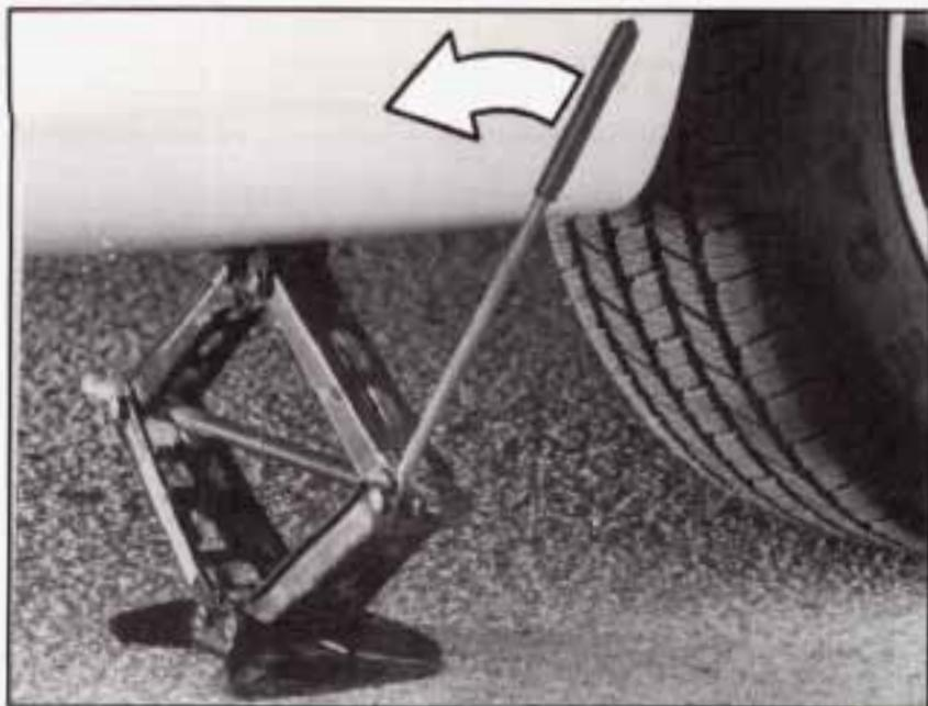
6. Lower the vehicle by turning the jack handle to the left. Lower the jack completely.
