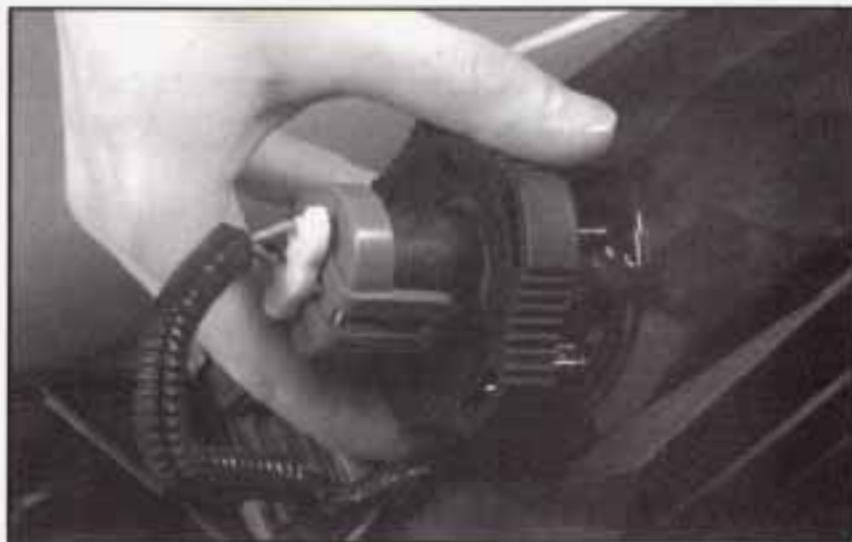
5. Turn the lamp socket ring a quarter of a turn counterclockwise to remove it from the headlamp assembly.
