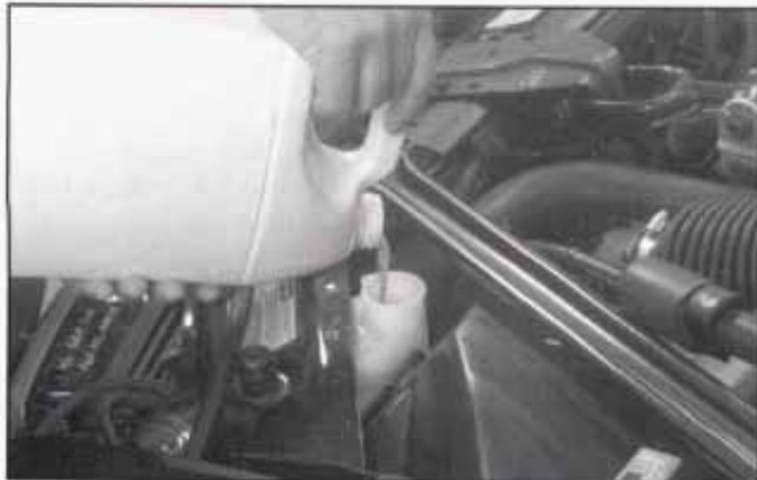
6. Then fill the coolant recovery tank to the FULL mark.
