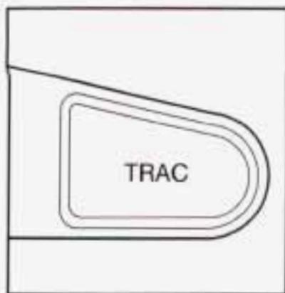
When you turn the system off, the Enhanced Traction System warning light will come on and stay on. If the Enhanced Traction System is limiting wheel spin when you press the button to turn the system off, the warning light will come on -- and the system will shut-off instantly. It will wait until there's no longer a current need to limit wheel spin.
