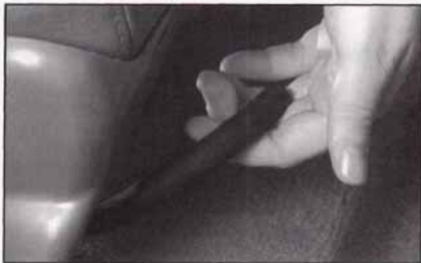
Lift the lever under the front of the seat up, using a twisting motion. This will unlock the seat. Slide the seat to where you want it and release the lever. Try to move the seat with your body to be sure the seat is locked in place.
