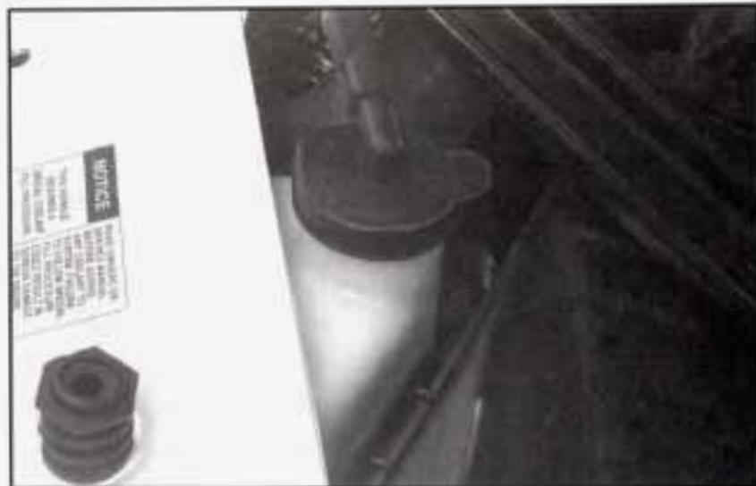
The coolant level should be at or above the COLD mark on the overflow hose in the coolant recovery tank. To check the coolant level, remove the cap on the coolant recovery tank. Check to make sure that the coolant level is up to the COLD fill level on the hose attached to the cap.
