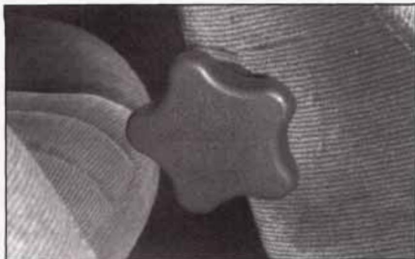
The knob that controls this feature is located on the right side of the driver's seat, about halfway down the seatback. Turn the knob clockwise to increase lumbar support. Turn the knob counterclockwise to decrease lumbar support.
