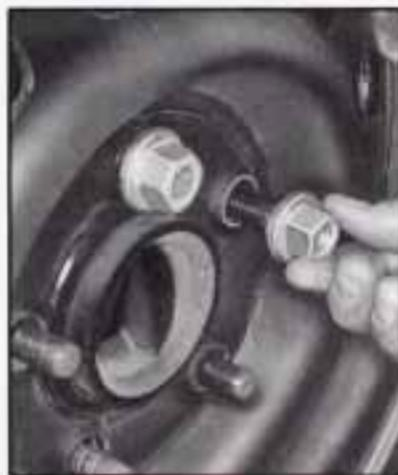
5. Replace the wheel nuts with the rounded end of the nuts toward the wheel. Tighten each nut by hand until the wheel is held against the hub.
