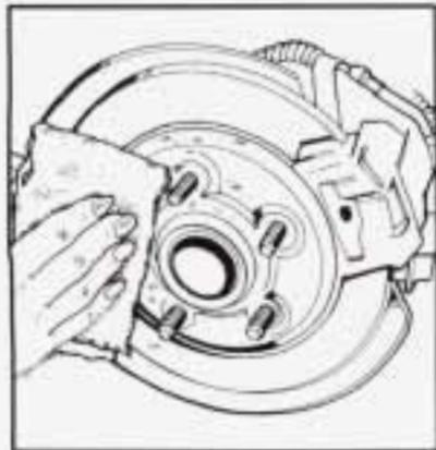
4. Remove any rust or dirt from the wheel bolts, mounting surfaces and spare wheel.
