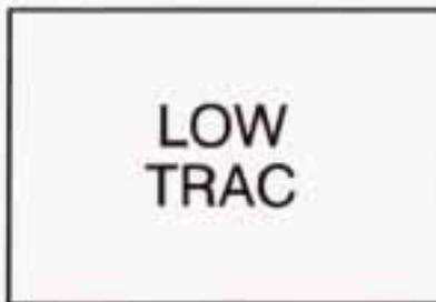
When your anti-lock system is adjusting brake pressure to help avoid a braking skid, this light will come on. See “Anti-Lock Brake System Warning Light” earlier in this section.
