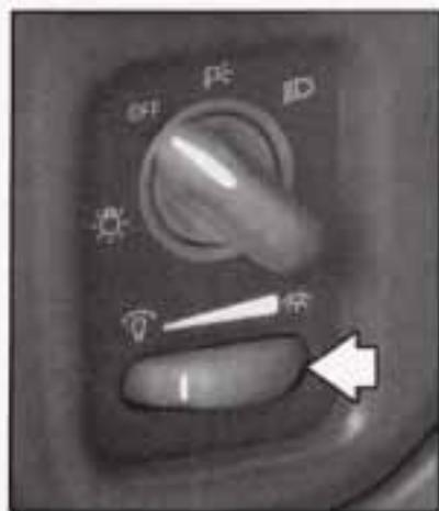
You can brighten or dim the instrument panel lights by turning the interior lamps dial.
