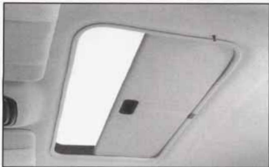
Your sunroof includes a sliding glass panel and a two-piece sunshade. The switch works only when the ignition or RAP is on. See "Retained Accessory Power" in the Index.
