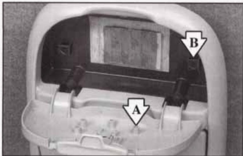
**SUNGLASSES STORAGE COMPARTMENT:** Your sunglasses storage compartment is the second compartment from the back on the overhead console. To open the sunglasses storage compartment, press the release latch forward and pull the compartment down to the full open position.
