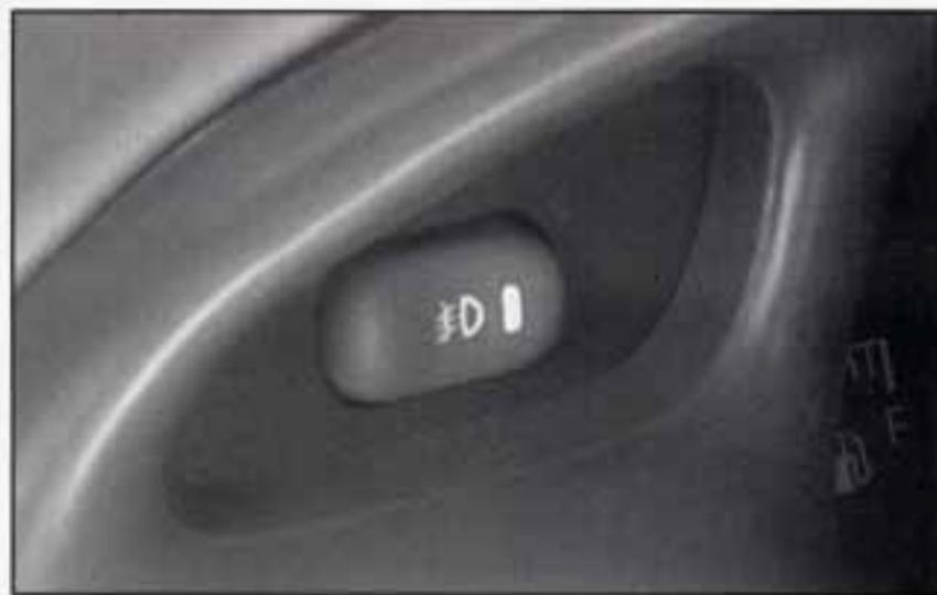
The fog lamps switch is located in the upper, left corner of the instrument panel, to the left of the instrument panel cluster.
