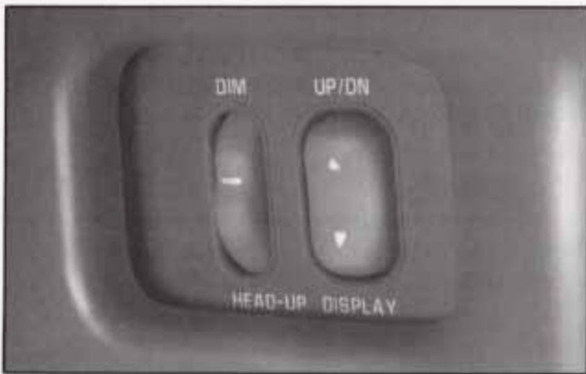
1. Start your engine and turn the DIM dial to the desired HUD image brightness.
