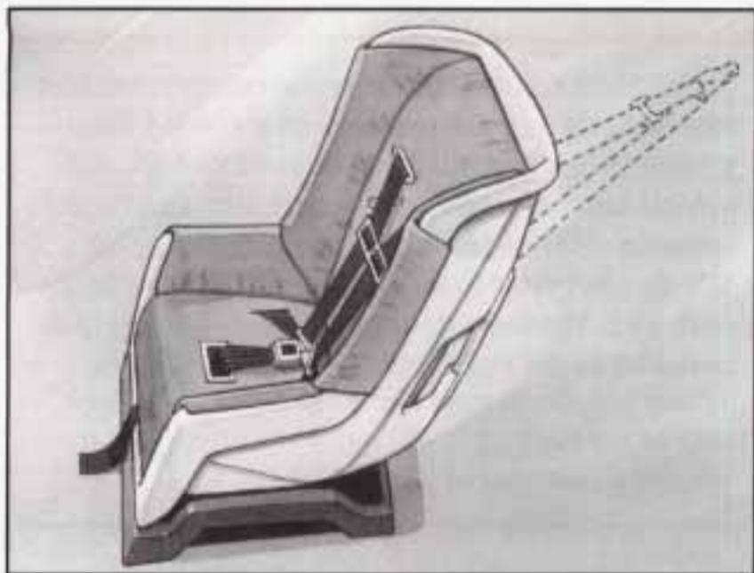
If your child restraint has a top strap, your dealer can obtain a kit with anchor hardware and installation instructions specifically designed for this vehicle. The dealer can then install the anchor for you. In Canada, this work will be done for you free of charge. Or, you may install the anchor yourself using the instructions provided in the kit.
