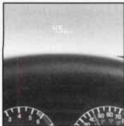
If you have the Head-Up Display (HUD), you can see the speedometer reading (in English or metric units) and a brief display of the current radio station or CD track, displayed “through” the windshield.
