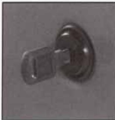
To unlock the trunk from the outside, insert the master key and turn it. You can also use the remote keyless entry transmitter, if your vehicle has this option.
