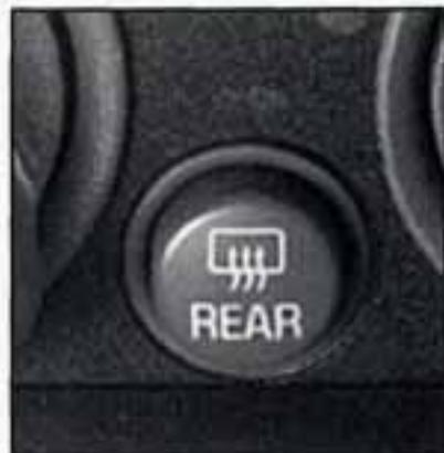
Your comfort control system has a button to operate your rear window defogger. The electronic comfort control system has a button marked REAR. The system with automatic temperature control has a button marked R.DEF.
