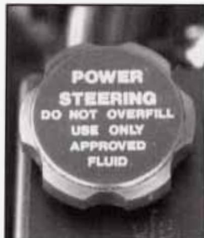
The power steering fluid reservoir is toward the rear of the engine compartment, on the passenger's side.
