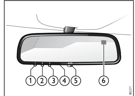
*Buttons for garage opener, autodimming and compass*
