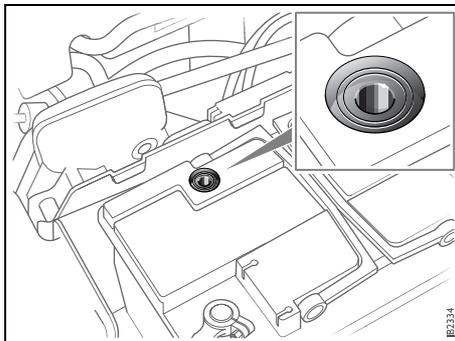
*Checking the battery electrolyte level.
