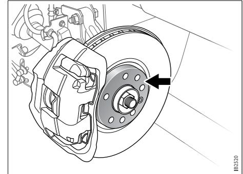
Clean any rust or dirt from the contact surfaces between the wheel and brake disc.
