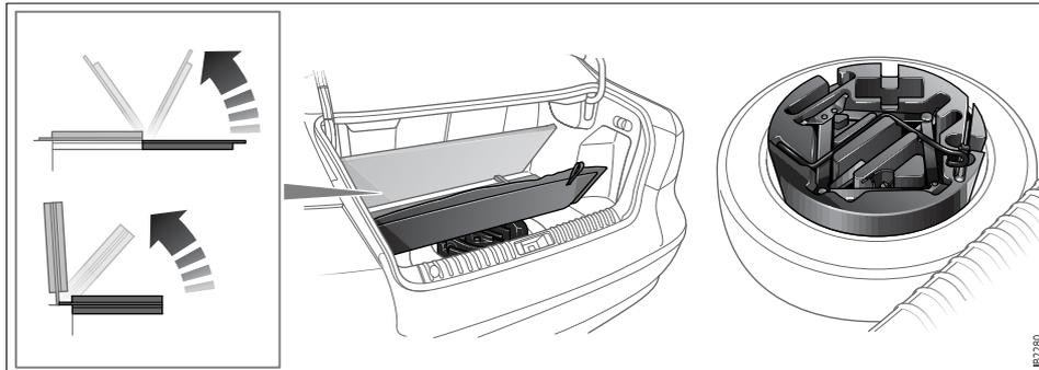
The spare wheel, the tools and the jack with its crank are carried under a panel in the trunk.
