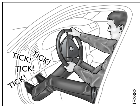
Braking with ABS brakes. When the system is operating, the brake pedal will pulsate gently and the system will make a ticking noise.
