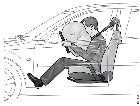
Inflated airbag (driver's side). Inflation and deflation of airbag takes approx. 0.1 s
