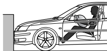
Sensors detect a deceleration and send a signal via the control module to a gas generator that inflates the airbag.
