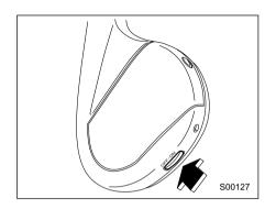
Press the <u>"OFF • ON"</u> button on the left earpiece to turn on the headphones: the <u>power</u> lamp <u>on the right earpiece</u> will come on.
