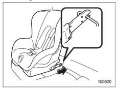
3. While following the instructions supplied by the child restraint system manufacturer, connect the lower hooks onto the lower anchorages located at "Q" marks on the bottom of the seatback. When the hooks are connected, make sure the adjacent seatbelts are not caught.
