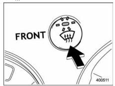
To defrost or dehumidify the windshield and front door windows, push the defroster button "w". When the "w" button is pushed, the indicator light on the button illuminates and the following operation is performed.
