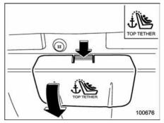
2. Open the lid of the cargo area, then remove the covers for the anchorages.
