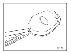
2. Open the key head using a flat-head screwdriver.
