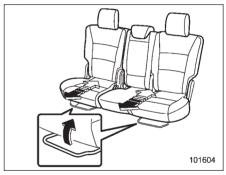
Pull the lever upward and slide the seat to the desired position.
