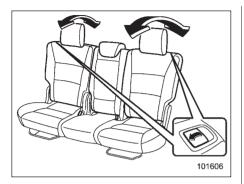
Pull the lever up and adjust the seatback to the desired position.
