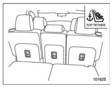
The tether anchorages (upper anchorages) are provided for all the seating positions of the second-row seat.
