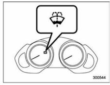
If you spray washer fluid on the windshield but the windshield washer fluid warning light illuminates or the supply of washer fluid appears to diminish, add washer fluid in the tank
