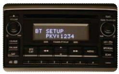
Put your phone into Bluetooth pairing mode and pair your phone to the system using the pass-key provided. When phone is successfully paired you will hear "The phone is paired and ready for use."
