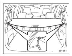
3. To extend the cover, pull the end of the cover out of the housing, then insert its hooks into the catches as shown. To rewind it, unhook it from the catches and it will rewind automatically. You should hold on to the cover and guide it back into the cover housing while it is rewinding.
