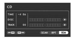
Highlight the "RDM" switch on the screen with the remote control joystick, then press the "ENTER" button.
