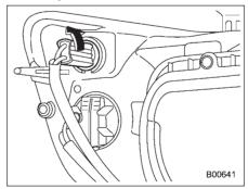
1. Remove the bulb socket from the
