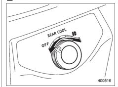
The rear air conditioner blows cool air out of the rear ventilators while the "A/C" button on the control panel is in the "ON" position. The fan speed of the rear air conditioner can be adjusted using the rear air conditioner dial behind the center console. The fan speed can be adjusted in four steps by turning the dial. Turn the dial to the "OFF" position to stop the fan.
