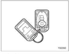
1. Carefully pry the remote engine start transmitter halves apart using a small flathead screwdriver
