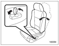
To adjust the angle of the seatback, move the control switch.
