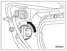
1. Remove the bulb socket from the headlight assembly by turning it counterclockwise.
