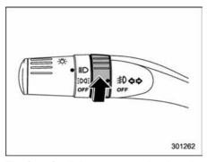
The front fog lights operate only when the light switch is in the "\( \)" position.
