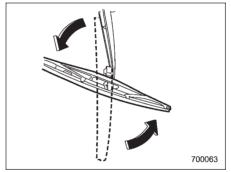
2. Turn the wiper blade assembly counterclockwise.
