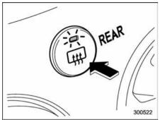
The outside mirror defogger shares the control switch with the rear window defoager. Therefore, the outside mirror defogger always operates with the rear window defogger.
