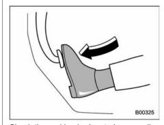
Check the parking brake stroke according to the maintenance schedule in the "Warranty and Maintenance Booklet". When the parking brake is properly adjusted, braking power is fully applied by depressing the pedal five to six notches gently but firmly (approximately 67 lbf [300 N, 30 kgf]). If the parking brake pedal stroke is not within the specified range, have the brake system checked and adjusted at your SUBARU dealer.
