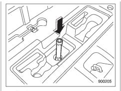
5. Fit the extension onto the hex-head hoist shaft end
