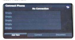
A pass-key pairing number will appear on the screen. Put your phone into Bluetooth pairing mode and pair your phone to the system using the pass-key provided.
