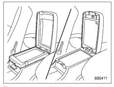
The center console box has a two-layer structure consisting of an upper compartment and a lower compartment.
