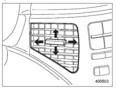
Move the tab to adjust the flow direction.
