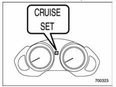
At this time, the cruise control set indicator light is illuminated on the combination meter.
