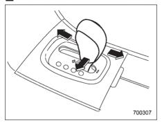
With the vehicle either moving or stationary, move the select lever from the "D" position to the manual gate then move it to the "+" end or "-" end of the manual gate to select manual mode.
