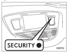
6. Briefly press the "□" button (for less than 2 seconds). All doors and the rear gate will lock, an electronic chirp will sound once, the turn signal lights will flash once and the indicator lights will start flashing rapidly. After rapid flashing for 30 seconds (standby time), the indicator lights will then flash slowly (twice approximately every 2 seconds), indicating that the system has been armed for surveillance.
