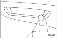
The rear gate light is located inside the vehicle on the rear gate. Push the right side of the switch to turn it on, and push the left side of the switch to turn it off.
