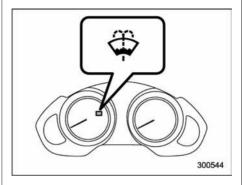
The windshield washer fluid warning light illuminates when the washer fluid level in the tank has dropped to the lower limit. If the warning light illuminates, refill the tank with fluid. For the tank refilling method, refer to "Windshield washer fluid" @ 11-28.
