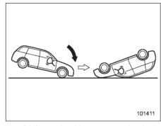
The SRS curtain airbags are not basically designed to deploy if the vehicle pitches end over end.
