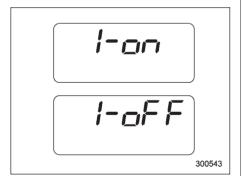
Briefly press the trip knob again. You can now establish the activated/deactivated setting for sequential illumination of the combination meter when the ignition switch is turned to the "ON" position. To change the current setting, press the trip knob for at least 2 seconds.
