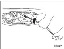
4. Tighten the towing hook securely using a jack handle.
