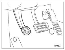
To set the parking brake, hold down the brake pedal while depressing the parking brake pedal as far as it will go.
