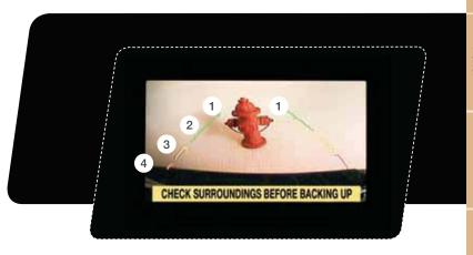
Vehicles with Navigation system have a rear view camera. When the selector lever is moved into "R" (Reverse) position, the rear view is shown on the display. Camera footage is live, real time as you see it on the rear view mirror. Also, width of the vehicle and distance from the vehicle are indicated as lines in the image on the display.
