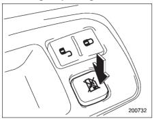
Push the lock switch. When the lock switch is in the "LOCK" position, the passengers' windows cannot be opened or closed.
