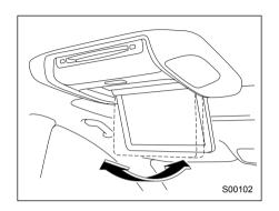
Adjust the display to the desired angle.
