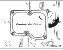
Open the access cover by removing the five clips and turning the access cover counterclockwise. The oil filter will be exposed.
