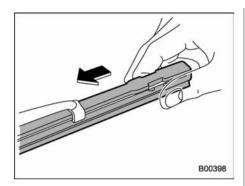
3. Align the claws of the metal support with the grooves in the rubber and slide the blade rubber assembly into the metal support until it locks.
