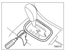
2. Remove the cover by prving on the edge with a flat-head screwdriver.
