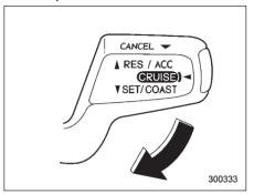
Push the control lever downward in the "SET/COAST" direction and hold it until the vehicle reaches the desired speed. Then, release the control lever. The vehicle speed at that moment will be memorized and treated as the new set speed.
