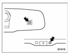
The mirror has a photosensor attached on both the front and back sides. Use care not to cover the sensors with stickers, or other similar items. Periodically wipe the sensors clean using a piece of dry soft cotton cloth or an applicator.
