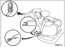
The second-row seat has four lower anchorages (bars) and three upper anchorages (tether anchorages) for accommodating such child restraint systems.
