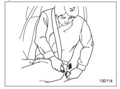
4. Insert the center seatbelt tongue plate in the center seatbelt buckle marked "CENTER" on the left-hand side until it clicks.
