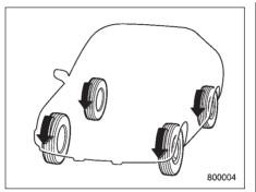
All-Wheel Drive distributes the engine power to all four wheels. AWD models provide better traction when driving on slippery, wet or snow-covered roads and when moving out of mud, dirt or sand. By shifting power between the front and rear wheels, SUBARU AWD can also provide added traction during acceleration, and added engine braking force during deceleration.
