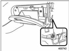
3. Remove the glove box by detaching the one clip on the side.
