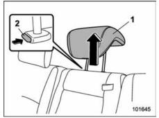
1. Raise the head restraint to the highest position at the seating position where the child seat has been installed using the seatbelt or lower anchorages; lift up the head restraint while pressing the release button.
