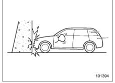
A head-on collision against a thick concrete wall at a vehicle speed of 12 to 19 mph (20 to 30 km/h) or higher activates only the driver's SRS frontal airbag or both driver's and front passenger's SRS frontal airbags. The airbag(s) will also be activated when the vehicle is exposed to a frontal impact similar in fashion and magnitude to the collision described ahove
