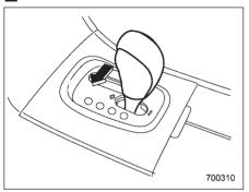
SPORT mode is used when power is needed for rapid acceleration or for uphill driving. To select this mode, move the select lever from the "D" position to the manual gate.
