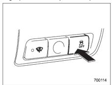
Traction Control system OFF switch
