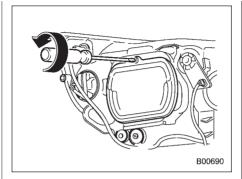
2. Use a screwdriver to remove the bulb cover
