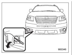
2. Wrap a flat-head screwdriver in vinvl tape or cloth, insert it into the gap between the cover and the front bumper, and use it to pry the cover open.
