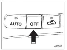
The Automatic Climate Control system turns off (the air conditioner compressor and fan turn off) when the "OFF" button is pressed.
