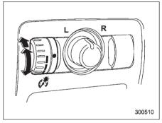
When the light switch is in the "OFF" position, you can adjust the brightness of the instrument panel illumination for better visibilitv.
