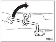
4. Tighten the towing hook securely using a wheel nut wrench.
