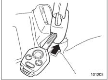
1. Insert a key or other hard pointed object into the slot in the connector (buckle) on the right-hand side and push
