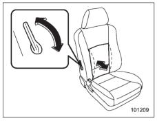
Pull the lever forward or backward Pulling the lever forward will increase the amount of support for your lower back. Pulling the lever backward will decrease the amount of support for your lower back.
