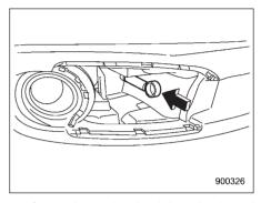
3. Screw the towing hook into the thread hole until the threads can no longer be seen.
