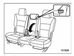
By pulling the tab on the center seat, you can fold only the seatback of the center seat
