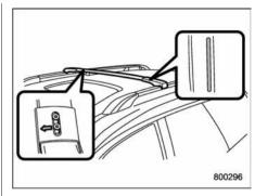
3. The crossbar with a 150 lbs (68 kg) load label attached onto it is the front crossbar. An arrow is marked on the back of the front crossbar for correct installation. Install the front crossbar so that the arrow faces the front of the vehicle.
