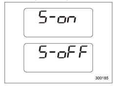
It is possible to activate or deactivate the movement of the meter needles and gauges and sequential illumination of the combination meter that takes place when the ignition switch is turned to the "ON" position.
