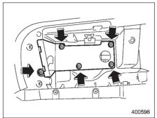
4. Remove the air filter cover by detaching the five clips.
