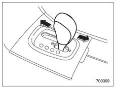
Shift to the next-higher gear by briefly pushing the select lever toward the "+" end of the manual gate.
