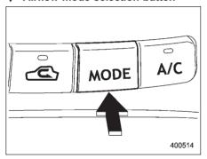
Select the desired airflow mode by pushing the airflow mode selection button. The selected airflow mode is shown on the center of the dial.
