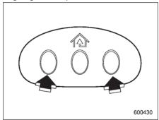
2. Press and hold the two outside buttons until the HomeLink® indicator light begins to flash (after 10 seconds). Release both buttons.
