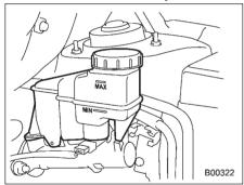
Check the fluid level on the outside of the reservoir. If the level is below "MIN", add the recommended brake fluid to "MAX". Use only brake fluid from a sealed container.
