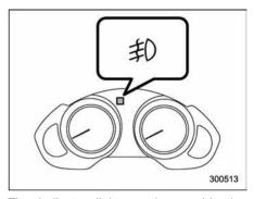
The indicator light on the combination meter will illuminate when the fog lights are illuminated.
