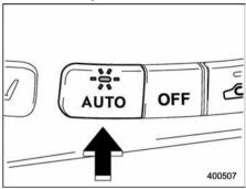
When the "AUTO" button is pressed, the indicator light on the button illuminates. In this state, fan speed, airflow distribution. air inlet control, and air conditioner compressor operation are automatically controlled.
