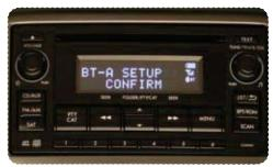
Pass-key for pairing will be given audibly as well as be displayed on the radio display.
