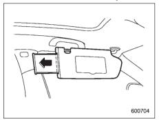
With the sun visor positioned over the side window, you can use the sun visor extension plate to prevent glare through the gap between the sun visor and center pillar. To use the extension plate, pull it toward the rear of the vehicle. When you have finished using it, stow it by pushing it toward the front of the vehicle
