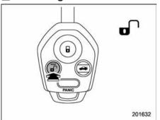
Press the "on" button to unlock the driver's door. An electronic chirp will sound twice and the turn signal lights will flash twice. To unlock all doors and the rear gate, briefly press the "on" button a second time within 5 seconds.
