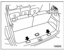
Two tether anchorages are attached to the rear edge of the cargo area.
