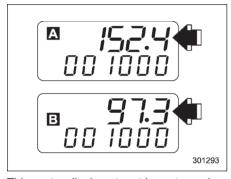
This meter displays two trip meters when the ignition switch is in the "LOCK", "Acc" or "ON" position.
