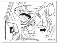
Raise the lever. The seatback of the second-row seat will tip forward and the seat will slide forward.
