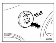
The rear window defogger operates only when the ignition switch is in the "ON" position.
