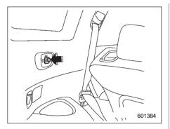
3. Insert the projections located on the both ends of the sleeve into the recesses of the retainers.
