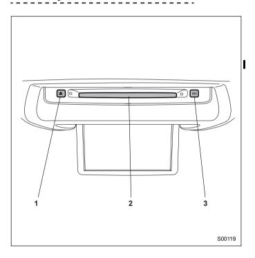
The DVD player can be operated when the ignition switch is in the "ACC" or "ON" position. Load a disc by inserting it into the disc slot of the player, with the label side facing up. The disc will be carried inward automatically when you insert it partially. The disc indicator light will turn on when the disc reaches the full inward position. To eject the disc, press the "Eject (A)" button. The disc will come out and the indicator light will go out.
