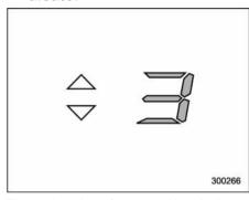
The select lever/gear position indicator shows the position of the select lever. When manual mode is selected, the gear position indicator shows the current gear position and the upshift/downshift indicator illuminates. Refer to "Automatic transmission" @7-12.
