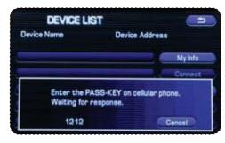
Put your phone into Bluetooth pairing mode and pair your phone to the system using the pass-key provided. When the phone is successfully paired the screen will show the phone's name on the list.
