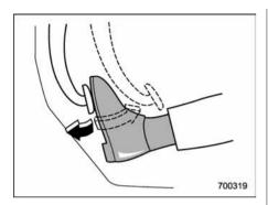
To release the parking brake, hold down the brake pedal while depressing the parking brake pedal and slowly releasing
