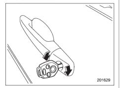
To lock the driver's door from the outside with the key, turn the key toward the front. To unlock the door, turn the key toward the rear.
