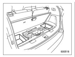
Hang the hook provided on the underside of the lid on the rear edge of the roof to keep the lid open.
