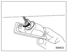
3. Remove the bulb socket from the license plate light assembly by turning it counterclockwise.
