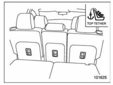
Three tether anchorages, i.e., ones for the right, center and left seats, are already installed on the back of each seatback. Open the cover flap to use each anchorage.
