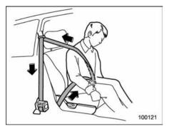
The driver's and front passenger's seatbelts have a seatbelt pretensioner. The seatbelt pretensioners for the driver's seat and front passenger's seat operate at the same time as the frontal, and side SRS airbags. If the vehicle rolls over, they operate simultaneously with the curtain airbag.
