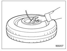
2. Insert the retainer through the center hole of the temporary tire (with the outside
