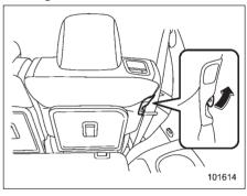
Raise the lever from the third-row seat. The seatback of the second-row seat will tip forward and the seat will slide forward. Before driving the vehicle, adjust the fore/aft position of the second-row seat, raise the seatback, and make sure the seatback is securely locked in position.
