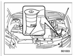
Remove the washer tank filler cap, then add washer fluid until it reaches the "FULL" mark on the tank.
