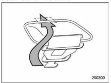
2. With the belt held by hand, allow the retractor to roll up the belt slowly. You should hold the webbing end and guide it back into the retractor while it is rolling up. Neatly store the tongue plate in the recess on the ceiling and then insert the connector (tongue) plate into the slot located at the front of the recess.
