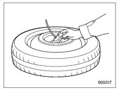
8. Tilt the retainer at the end of the cable
