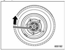
17. Use the wheel nut wrench to securely tighten the wheel nuts to the specified
