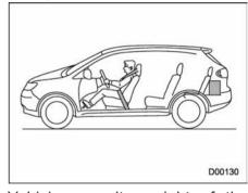
Vehicle capacity weight of the vehicle is 1,157 lbs (525 kg), which is indicated on the vehicle placard with the statement "The combined weight of occupants and cargo should never exceed 525 kg or 1,157 lbs".
