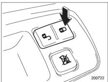
5. Before the electronic tone stops sounding, push the "\(\overline{1}\)" side of the power door locking switch the same number of times as the leftmost digit of the transmit-
