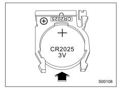
Install a new battery (Type CR2025 or equivalent) in the holder. Make sure the battery's positive (+) side and the "+" mark on the holder are on the same side. Slide the battery holder into the remote control until it clicks.
