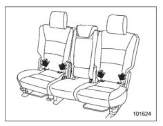
The lower anchorages (bars) are used for installing a child restraint system only on the window-side seating positions. For each window-side seating position, two lower anchorages are provided.
