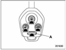
Rear gate unlock button : Unlock/disarm button ☐: Lock/arm button A: Panic button
