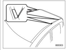
Each of the two roof moldings has two mounting points for crossbars. Each mounting point is fitted with a cover. Use a screwdriver to remove the covers. When installing the crossbars on the roof molding, follow the manufacturer's instructions.
