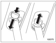
The shoulder belt anchor height should be adjusted to the position best suited for the passenger. Always adjust the anchor height so that the shoulder belt passes over the middle of the shoulder without touching the neck.
