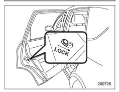
Each rear door has a child safety lock that prevents the door from being opened even if the inside door handle is pulled.
