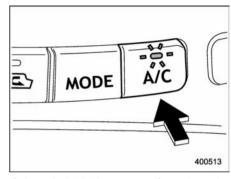
If the windshield starts to fog when the climate control system is operated in the AUTO mode, push the air conditioner button to defog and dehumidify.
