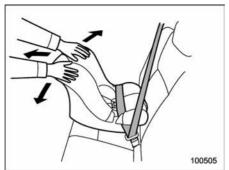
8. Push and pull the child restraint system forward and from side to side to check if it is firmly secured.
