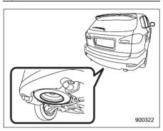
The spare tire is stored in the spare tire holder located under the cargo area.
