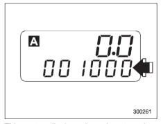
This meter displays the odometer when the ignition switch is in the "LOCK", "Acc" or "ON" position.
