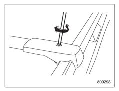
6. Adjust the alignment of the crossbar on the roof rails, and if available, use a T-30 torx<sup>®</sup> bit and torque wrench and tighten the T-30 torx<sup>®</sup> head screws to 30 to 35 lbf·in (3.4 to 4.0 N·m, 0.35 to 0.41 kgf·m) of torque (or tighten securely with the torx<sup>®</sup> wrench provided).
