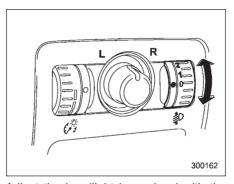
Adjust the headlight beam level with the following dial positions according to the number of passengers and load condition.
