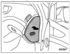
1. Remove the instrument panel side cover
