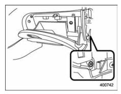
10. Secure the glove box with the one clip.11. Install the instrument panel side cover.
