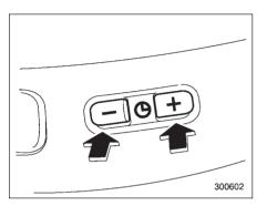
To adjust the time shown by the clock, press the "+" button or the "-" button. The indicated time will change in 1-minute increments. If you keep the button pressed, the rate at which the indicated time changes will speed up.
