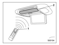
To use the remote control, direct its signal-emitting eye toward the signal reception window of the display.
