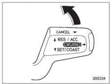
Push the control lever upward in the "RES/ ACC" direction and hold it until the vehicle reaches the desired speed. Then, release the control lever. The vehicle speed at that moment will be memorized and treated as the new set speed.
