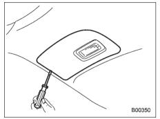
1. Use a flat-head screwdriver to remove the rear gate light assembly from the rear gate trim.
