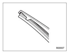
Securely retain both ends of the rubber with the stoppers on the plastic support ends. If the rubber is not retained properly, the wiper may scratch the rear window glass.
