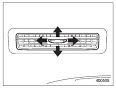
Move the tab or rotate it to adjust the flow direction.
