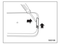
While holding the battery holder pushed in the direction of the arrow with your fingernail inserted in the slot, slide out the holder in the direction of the arrow using a cross-head mini screwdriver.
