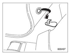
A retaining pin is located on the driver's side of the vehicle next to the fuel filler door release. Fit the grommet in the carpet onto the pin to prevent the carpet from moving.
