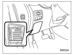
The fuses are designed to melt during an overload to prevent damage to the wiring harness and electrical equipment. The fuses are located in two fuse boxes. One is located under the instrument panel behind the fuse box cover on the driver's seat side.
