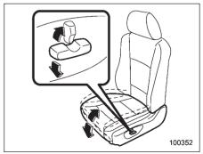
To adjust the seat cushion angle, pull up or push down the front end of the control switch.
