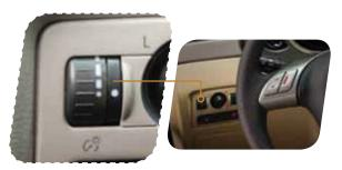
When the dial is turned downward, illumination becomes dim. When the dial is turned upward, illumination becomes bright. When the dial is fully turned upward while the light switch is on, instrument panel illumination becomes bright.
