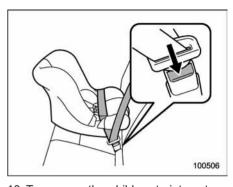
10. To remove the child restraint system. press the release button on the seatbelt buckle and allow the belt to retract completely. The belt will return to the FLR mode.
