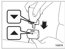
3. After confirming that the webbing is not twisted, insert the connector (tongue) attached at the webbing end into the buckle on the right-hand side until a click is heard. Make sure that the "\(\nsigma\)" mark on the connector (tongue) and the "\(\nsigma\)" mark on the buckle are aligned.
