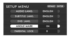
On the SETUP MENU screen, highlight "ANGLE MARK" with the remote control joystick, followed by pressing the "ENTER" button. Then, the angle mark display switches between "ON" and "OFF" each time the "ENTER" button is pressed. Select either "ON" or "OFF" as desired.
