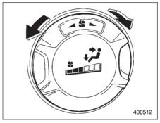
The fan speed control dial has 7 positions: AUTO position and 6 different fan speed positions.
