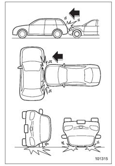
The driver's and front passenger's SRS frontal airbags are designed not to deploy
