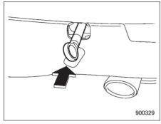
3. Screw the towing hook into the thread hole until its thread can no longer be seen.
