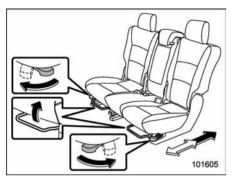
When the right seat or the left seat pair is slid rearward, it stops partway at the lock point so as not to trap the legs of passengers sitting on the third-row seat.
