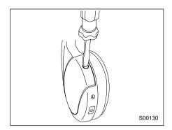
Remove the battery cover on the left earpiece by loosening the screw with a flathead screwdriver.
