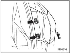
2. Using a Phillips screwdriver, remove the upper and lower screws. Then, slide the rear combination light assembly rearward and remove it from the vehicle.
