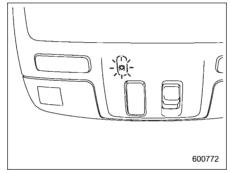
The automatic ambient light illuminates when the ignition switch is in the "ON" position and the light control switch is in the "soos" position or "SO" position. The light dimly illuminates the area around the center console. The light turns off when the light control switch is in the "OFF" position. Also, the brightness of the light is adjusted by the illumination brightness control dial.
