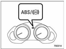
The ABS warning light illuminates when the ignition switch is turned to the "ON" position and turns off after approximately 2 seconds.
