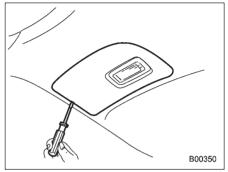
1. Use a flat-head screwdriver to remove the light cover from the rear gate trim.
