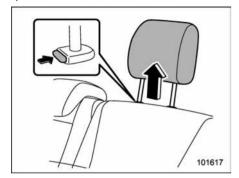
1 Remove the head restraint at the window-side seating position where the child restraint system has been installed with the lower anchorages or seatbelt; lift up the head restraint while pressing the release button. Store the head restraint in the cargo area. Avoid placing the head restraint in the passenger compartment to prevent it from being thrown around in the passenger compartment in a sudden stop or a sharp turn.
