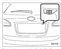
A rear view camera is attached to the rear gate. When the ignition switch is "ON" and the select lever is set to "R", the rear view camera automatically displays the rear view image behind the vehicle on the navigation monitor or on the inside mirror.
