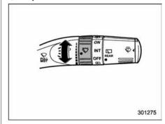
When the wiper switch is in the "T" position, turn the dial to adjust the operating interval of the wiper.
