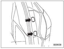
1. Remove the two covers by inserting the tip of a flat-head screwdriver.
