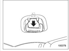
Center seatbelt is stowed in the recess of the ceiling.
