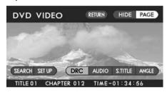
Highlight the "DRC" switch on the screen with the remote control joystick, then press the "ENTER" button. The display will switch to the dynamic range control selection screen.
