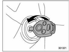
The key can be turned from "Acc" to "LOCK" only when the select lever is in the "P" position.
