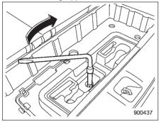
3 Turn the hoist shaft end clockwise with the wheel nut wrench to wind the cable up completely until you hear a few clicking sounds. Confirm that the temporary spare tire holding cable has been wound up completely by shaking the temporary tire.
