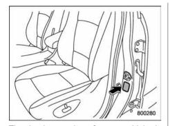
The load capacity of your vehicle is determined by weight, not by available cargo space. The maximum load you can carry in your vehicle is shown on the vehicle placard attached to the driver's side door pillar. It includes the total weight of the driver and all passengers and their belongings, any optional equipment such as a trailer hitch, roof rack or bike carrier. etc., and the tongue load of a trailer.
