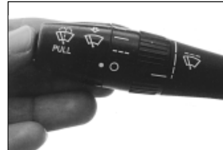
Pull upward for windshield wash and wipe. Pull towards driver for FLICK WIPE (Spring Return)
