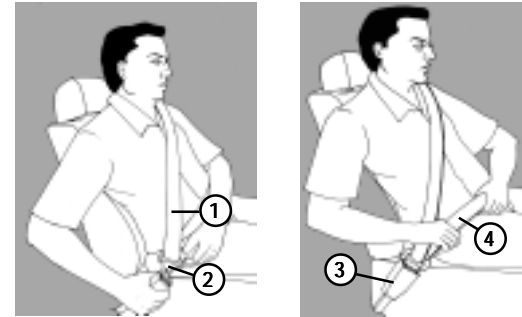
1. Seat Belt 2. Tongue 3. Lock Buckle 4. Lap Belt
