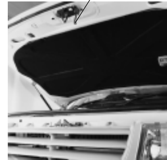
Additional lock lever under the bonnet centre
