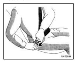
Adjust the seat as needed (front seats only) and sit up straight and well back int eh seat. To fasten your belt, pull it out of the retractor and insert the tab into the buckle.
