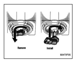
Turn the bulb clockwise and remove it. Install a new bulb, turn it counterclockwise, then plug in the connector.
