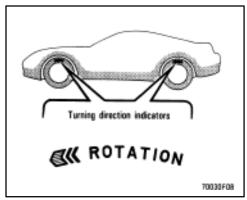
Do not perform rotation of the tires, from front to rear or from left to right, or using the compact spare tire. Performing such tire rotation may result in the tires interfering with the body or in uneven wear of the tires, so that steerability of the vehicle is impaired.
