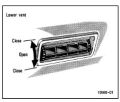
If air flow control is not satisfactory, check the instrument panel vents. The instrument panel vents may be opened or closed as shown.
