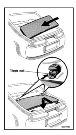
Put in the roof from the left side as shown. Then insert the front edge of the roof in the front holders, and engage the rear edge with the rear holders.
