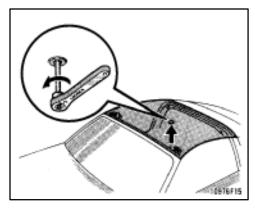
3. Unlock the center lock by inserting the wrench and turning it a 1/4 turn counterclockwise.
