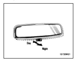
Pull the lever toward you to reduce glare from the headlights of the vehicle behind you during night driving.
