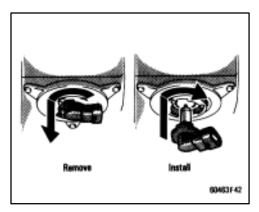
Turn the bulb counterclockwise and remove it. Install a new bulb, turn it clockwise, then plug in the connector.
