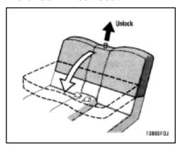
FOLDING DOWN REAR SEAT Unlock the seatback, and fold it down.
