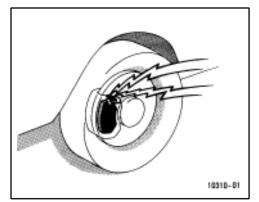
The brake pas wear limit indicators on your disc brakes give a warning noise when the brake pads are worn to where replacement is required.
