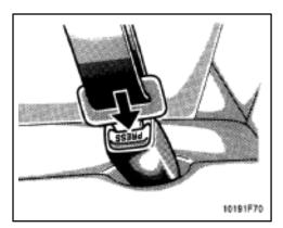
To remove the convertible seat, press the buckle–release button and allow the belt to retract completely. The belt will move freely again and be ready to work for an adult or older child passenger.
