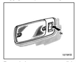
To turn the luggage compartment light on, open the back door and push the switch. Closing the back door will turn the light off.
