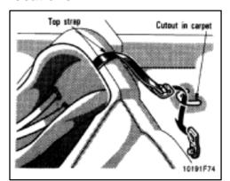
If your child restraint system requires the use of a top strap, latch the hood onto the anchor bracket and tighten the top strap.
