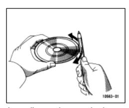
A new disc may have rough edges on its inner and outer perimeter. Remove the rough edges by pressing the side of a ball-point pen or pencil against the inner and outer perimeter of the disc as shown.
