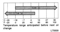
If you use SAE 10W-30 engine oil in extremely low temperatures, the engine may become difficult to start, so SAE 5W-30 engine oil is recommended.
