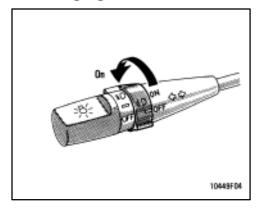
To turn on the front fog lights, twist the knob of the headlight and turn signal switch lever. They will come on when the headlights are turned on low beam.
