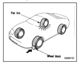
Block the wheel diagnoally opposite the flat tire to keep the vehicle from rolling when it is jacked up.
