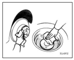
Before putting on wheels, remove any corrosion on the mounting surfaces with a wire brush or such. Installation of wheels without good metal—to—metal contact at the mounting surface can cause wheel nuts to loosen and eventually cause a wheel to come off while driving. Therefore after the first 1600 km (1000 miles), check to see that the wheel nuts are tight.
