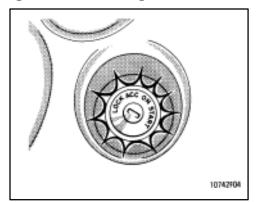
For easy access to the ignition switch, the ignition switch light comes on when either side door is opened.
