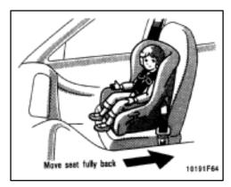
®Only when it is unavoidable should a forward–facing child restraint system be used on the front seat. Always move the seat as far back as possible because the force of deploying airbag would cause serious injury to the child.
