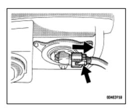
Unplug the connector while depressing the lock release.
