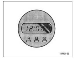
Once the electrical power source has been disconnected from the clock, the time is automatically set to 1:00 (one o'clock).
