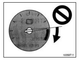
The tachometer indicates engine speed in thousands of rpm (revolutions per minute). Use it while driving to select correct shift points and to prevent engine lugging and overreving.
