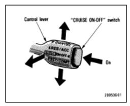
The cruise control allows you to cruise the vehicle at a desired speed over 40 km/h (25 mph)even with your foot off the accelerator pedal.
