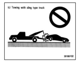
(c) Towing with sling type truck
