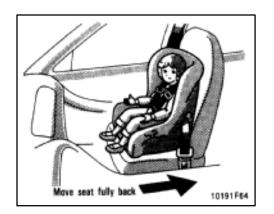
®If you must use a forward-facing child restraint system in the front seat, the seat must be moved as far back as possible. For instructions concerning the installation of a child restraint system, see "Child restraint" in this chapter.
