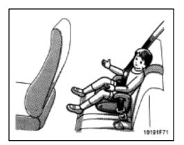
(C)BOOSTER SEAT INSTALLATION A booster seat is used in forward–facing only.
