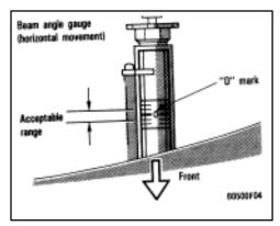
Look at the beam angle gauge (horizontal movement). The "0" mark should not deviate by more than one mark on either side of the gauge.
