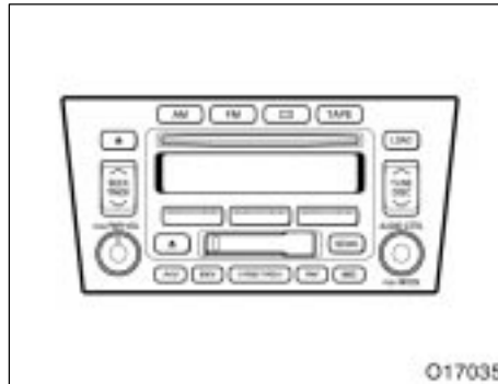
Type 2: AM-FM ETR radio/cassette player/ compact disc auto changer controller/ compact disc auto changer
