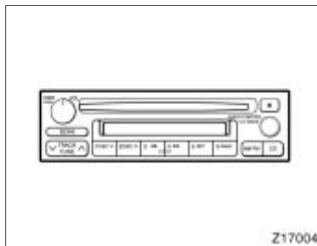
Type 4: AM-FM ETR radio/compact disc player
