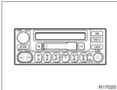
Type 2: AM-FM ETR radio/cassette player/compact disc auto changer controller
