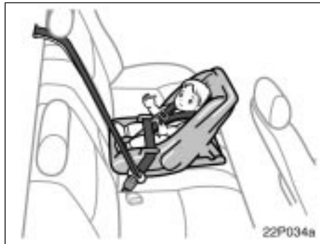
(A) INFANT SEAT INSTALLATION An infant seat is used in rear-facing position only.
