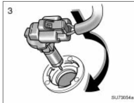
3. Install a new bulb base by turning it clockwise to the front of the vehicle.
