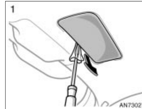
Remove the cover with a flat-bladed screwdriver which is wrapped with a cloth.
