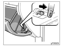
1. Open the glove box, and slide off the damper as shown.
