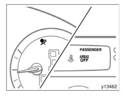
The SRS warning light and "AIRBAG OFF" indicator light will come on if there is a malfunction in the front passenger occupant classification system.
