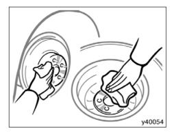
Before putting on wheels, remove any corrosion on the mounting surfaces with a wire brush or such. Installation of wheels without good metal-to-metal contact at the mounting surface can cause wheel nuts to loosen and eventually cause a wheel to come off while driving.
