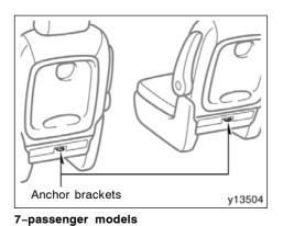
Use the anchor brackets on the back of the second seats to attach the top strap. Anchor bracket is installed for each second seating position.
