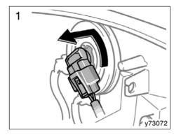
1. Open the hood. Turn the bulb base counterclockwise to the front of the vehicle as shown.
