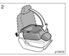
2. Pull the seatback folding lever and fold the seatback down.
