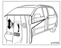
Open the sliding door fully and move the lock lever to the "LOCK" position as shown on the label. Then close the sliding door.
