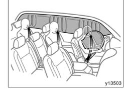
The SRS (Supplemental Restraint System) side airbags and curtain shield airbags are designed to provide further protection for the driver and all window-side passengers in addition to the primary safety protection provided by the seat belts.
