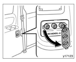
To use the input terminal adapter, open the cover.
