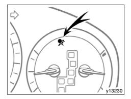
This indicator comes on when the ignition switch is turned to the "ON" position. It goes off after about 6 seconds. This means the SRS front airbags are operating properly.
