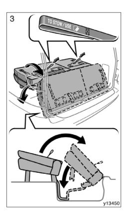
3. Pull and hold the seat lock release strap ("TO STOW/USE" printed on its surface) and lift up the seat rearward. Then push the seat down.
