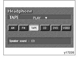
The mode display which is selected by the joy stick is colored blue. When the "ENT" button is pushed, the mode display changes to green. If the mode display is gray, it cannot be selected.
