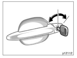
When either front door is unlocked with a key, the front personal lights and ignition switch light will come on and remain on for about 15 seconds before fading out. (For details, see "Front personal lights" on page 164 and "Ignition switch light" on page 166 in Section 1–5.)
