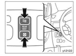
The quarter windows can be operated with the "REAR VENT" switch on the instrument panel.
