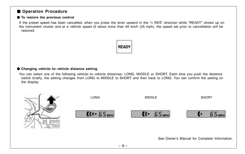
In addition to the vehicle-to-vehicle distance control mode described in this quick reference guide, dynamic laser cruise control has conventional (fixed speed) cruise control mode for cruising at fixed speeds. For the conventional (fixed speed) cruise control mode, see Section 1-7 in the "Owner's Manual".
