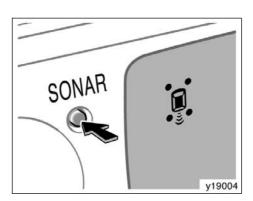
If the indicator is continuously on, have your Toyota dealer check the system. If the indicator remains blinking but you do not hear the buzzer sound, clean the sensors with soft cloth.
