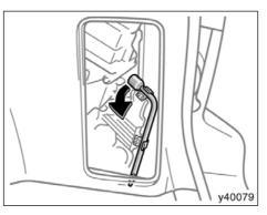
To remove the wheel nut wrench, first disengage the upper part of the wrench from the holding bracket and remove it.
