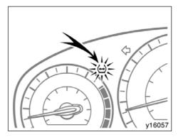
When initializing the system, make sure the low tire pressure warning light blinks three times. If the warning light does not blink three times, initializing will be failed and the tire pressure warning system will not function properly.
