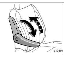
To adjust the armrest, lower the armrest to the lowest position and raise it to the desired angle. Raising the armrest to the highest position unlocks the armrest to let you return it to the lowest position.
