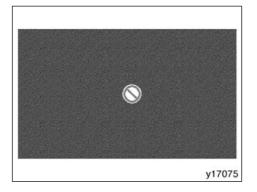
If " $\otimes$ " appears on the screen when you select a switch, it indicates that the switch cannot work.
