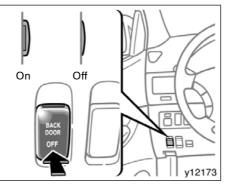
This switch is used to turn on and off the power back door system. In order to operate the power back door, the "BACK DOOR OFF" switch on the instrument panel must be pushed out. (The orange line on the top of the switch indicates that the power back door system is on.) To disable the power back door feature, push in the switch.
