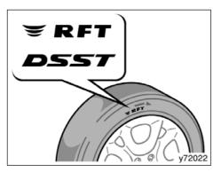
Some vehicles are equipped with run-flat (RFT) tires. The run-flat tire allows you to continue driving for up to 160 km (100 miles) at a speed below 90 km/h (55 mph) even if any tire goes flat. However, in some conditions (such as high temperatures), you could not continue driving for up to 160 km (100 miles).
