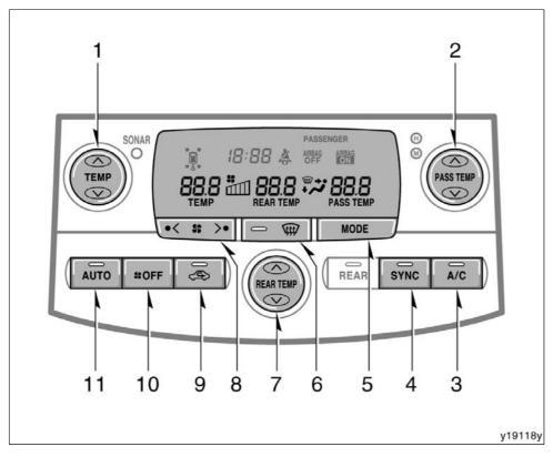
Temperature selector ("TEMP") (with "SYNC" button indicator on—simultaneous setting on driver, front passenger and rear passenger sides) (with "SYNC" button indicator
