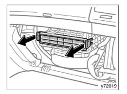
3. Remove the filter case from the filter outlet as shown in the illustration.
