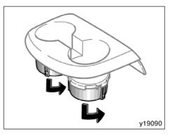
Before installing the cup holder, push down the bottom of the cup and turn it counterclockwise to lock.
