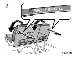
2. Pull the seatback angle adjusting strap ("TO FOLD/LIFT SEATBACK" printed on its surface), then fold down the seatback.
