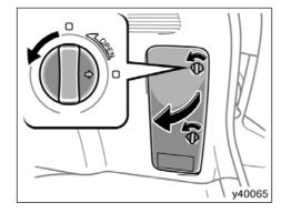
To remove the tools, turn the knob counterclockwise and remove the cover.
