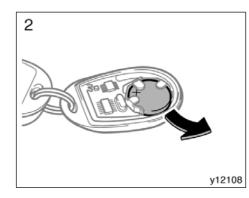
2. Remove the discharged transmitter battery.
