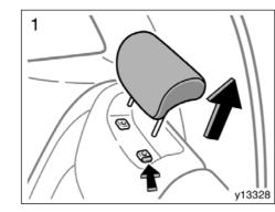
TO USE THE ANCHORAGES: 1. Remove the head restraint.
