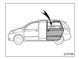
When the sliding door window is opened more than about 15 cm (6 in.), the sliding door will stop at halfopened position for safety reasons. Close the window and then operate the sliding door.
