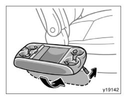
To fold down the table, pull up the lock release lever and push against the driver's seat side.
