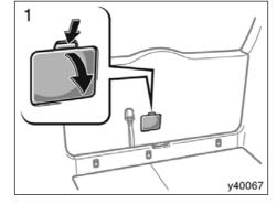
If the back door opener does not operate, you can open the back door from the inside.
