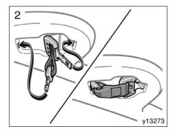
2. To stow the center seat belt, pull it slightly out of its cover. It will automatically roll back partway. Roll the seat belt backwards as shown above and insert it into the slot of its cover. Make sure the tabs are securely locked in the cover.
