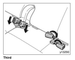
The seat belt buckles of the second seats (7-passenger models) and third seats can be stowed when not in use.
