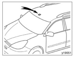
The compass sensor is on the roof of the vehicle.
