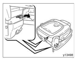
If you lock the rear legs before the front legs are locked securely, disengage the rear leg lock by pushing the red pin inside each rear leg. Then reinstall the seat following the correct procedure.
