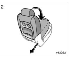
2. Fold down the seatback while pulling the seatback angle adjusting strap.
