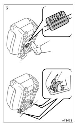
2. Push the foot pedal forward to securely latch the front leg locks. Make sure the front leg is locked securely, fold down the seat and engage the rear leg lock.
