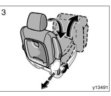
3. Fold down the seatback while pulling the seatback angle adjusting lever or strap and swing up the seat.
