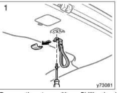
Remove the strap with a Phillips-head screwdriver.
