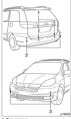
The Toyota park assist system is designed to inform you of the approximate distance between your vehicle and an obstruction by indicator and buzzer while driving at approximate 10 km/h (6 mph) or less when parking the vehicle. This system uses sensors to detect obstructions.
