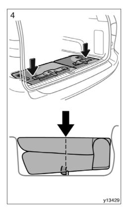
4. Push the seat against the floor and make sure it is locked securely.
