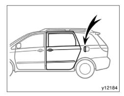
When the fuel filler door is opened, the left side siding door will not open. Close the fuel filler door securely and then operate the sliding door.
