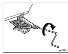
6. After making sure that no one is in the vehicle, raise it high enough so that the spare tire can be installed.
