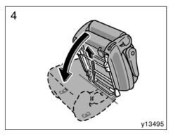
4. Pull and hold the front leg release strap and fold down the seat. Then the front leg locks will disengage and you can remove the seat.
