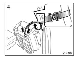
4. Take the holding strap out of the pocket. Pass the strap through the assist grip, and hook it as shown in the illustration.
