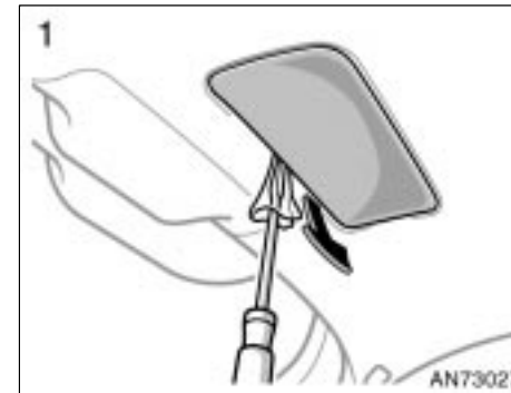
Remove the cover with a flathead screwdriver which is wrapped with a cloth.
