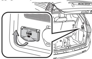
Designed for car accessories. Engine switch/“ENGINE START STOP” switch must be in the “ACC” or “ON” position to be used.
