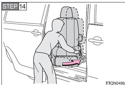
Rotate the seat into a position which does not cause the left edge of the seat cushion to make contact with the vehicle body.
