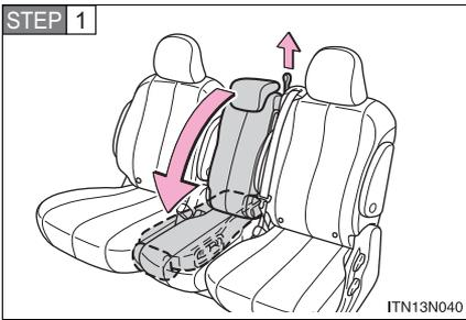
Pull the lock release strap and fold down the second center seatback.
