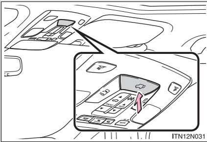
Press and hold the switch to open/close the back door.
