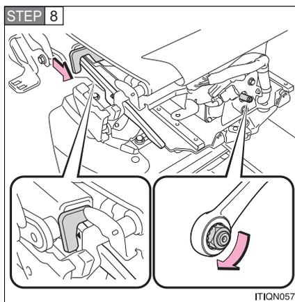
Turn the bolt with yellow marking using the combination wrench, and move the AUTO ACCESS SEAT until the marks are aligned as shown in the illustration.
