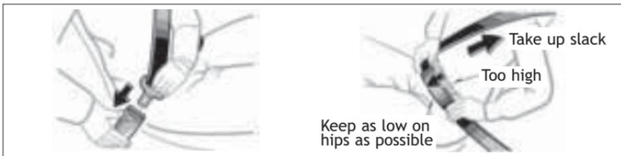
If belt is fully extended, then retracted even slightly, it cannot be re-extended beyond that point, unless fully retracted again. This feature is used to help hold child restraint systems securely.
