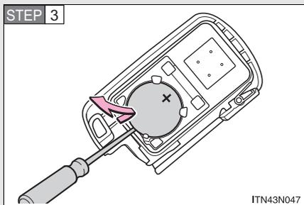
Remove the depleted battery.
