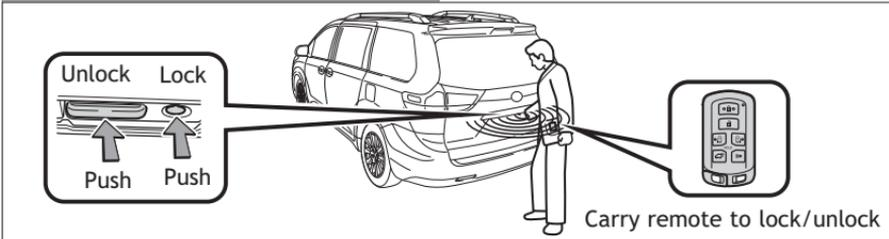
\* Driver door unlocking function can be programmed to unlock driver side doors only, or all doors. Grasping any passenger door handle will unlock all doors.
