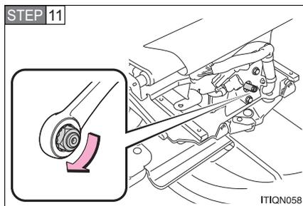
Turn the bolt with yellow marking using the combination wrench, and move the AUTO ACCESS SEAT until the bolt can no longer be turned.
