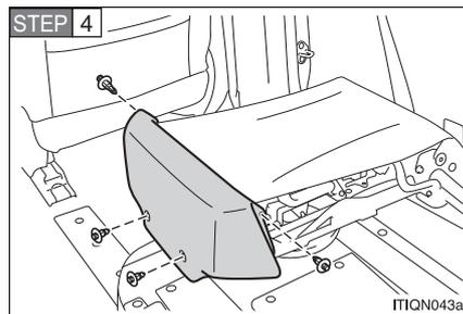
Remove the 4 clips and remove the unit cover. (→P. 57)
