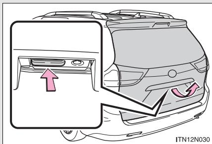
Raise the back door while pressing the back door opener to release the lock to open the back door.
