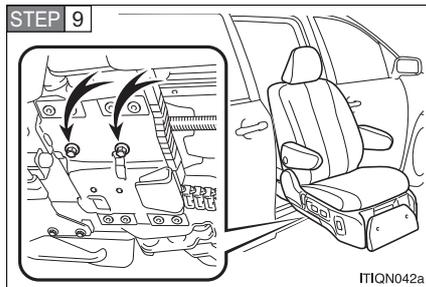
Use the combination wrench to remove the 2 bolts on the underside of the AUTO ACCESS SEAT.
