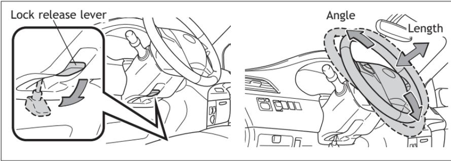
Hold wheel, push lever down, set angle and length, and return lever.
