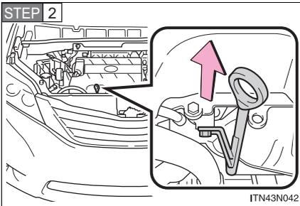
Holding a rag under the end, pull the dipstick out.
