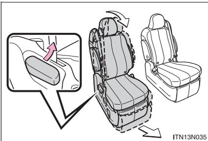
Pull the seatback angle adjustment lever and fold down the seatback. The seat can slide forward. Move the seat to the front-most position.
