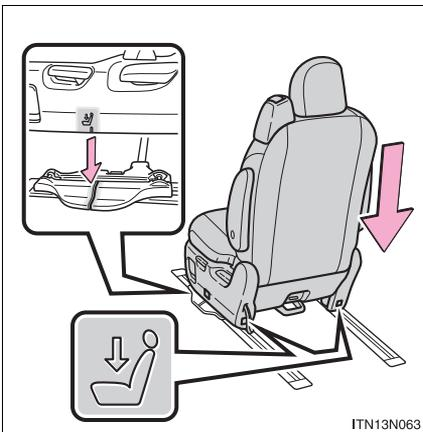
Align the marking on the seat back cover to the rail.
