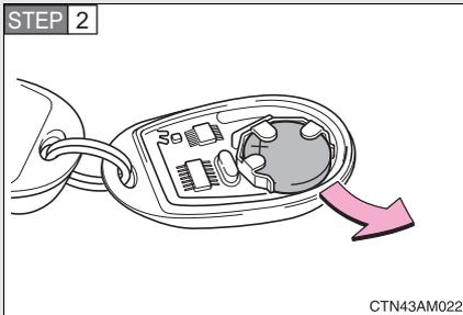
Remove the discharged transmitter battery.
