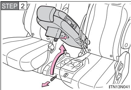
Pull the lock release strap under the seat to remove the seat. Retract the cushion leg.
