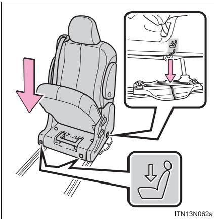
Align the marking on the seat front cover to the rail.
