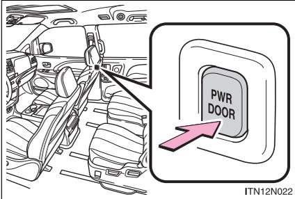
Press the switch to open and close each sliding door.
