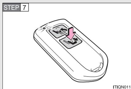
Press and hold the seat lower switch on the wireless remote control to rotate and lower the AUTO ACCESS SEAT.
