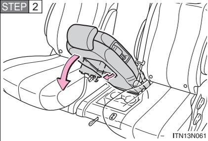
Unfold the cushion leg and push down on the seat to engage the front lock.
