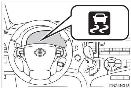
If the vehicle is in danger of slipping or if any of the drive wheels spins, the slip indicator light flashes to indicate that the Enhanced VSC/TRAC systems are operating.
