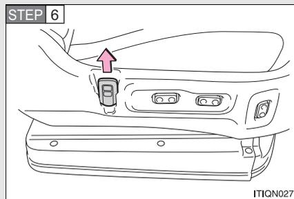
Remove the wireless remote control from the AUTO ACCESS SEAT.
