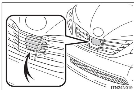
The radar sensor detects vehicles or other obstacles on or near the road ahead and determines whether a collision is imminent based on the position, speed, and heading of the obstacles.
