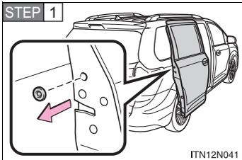
Remove the plug from the rear edge of the sliding door.
