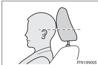
Make sure that the head restraint is adjusted so that the center of the head restraint is closest to the top of your ears.
