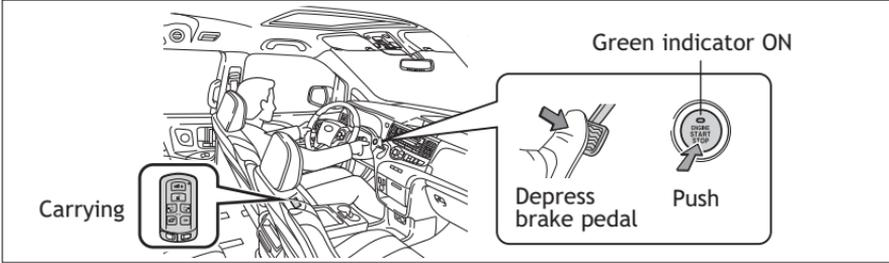
**NOTE:** Gear shift lever must be in Park and brake pedal depressed.
