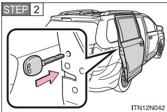
Insert a key in the hole and push the mechanical cancel lever.
