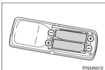
Remove the depleted batteries and install new 2 AA batteries.
