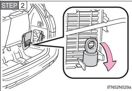
Remove the adapter socket.
