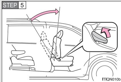
Fold the front passenger seat-back while pulling the seat-back angle lever.
