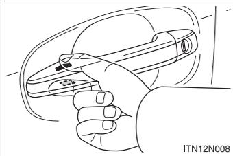
Touch both lock sensors on the upper and lower part of the front door handle simultaneously.
