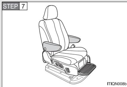
Adjust the armrest and foot restraint on the AUTO ACCESS SEAT to the down-most position.
