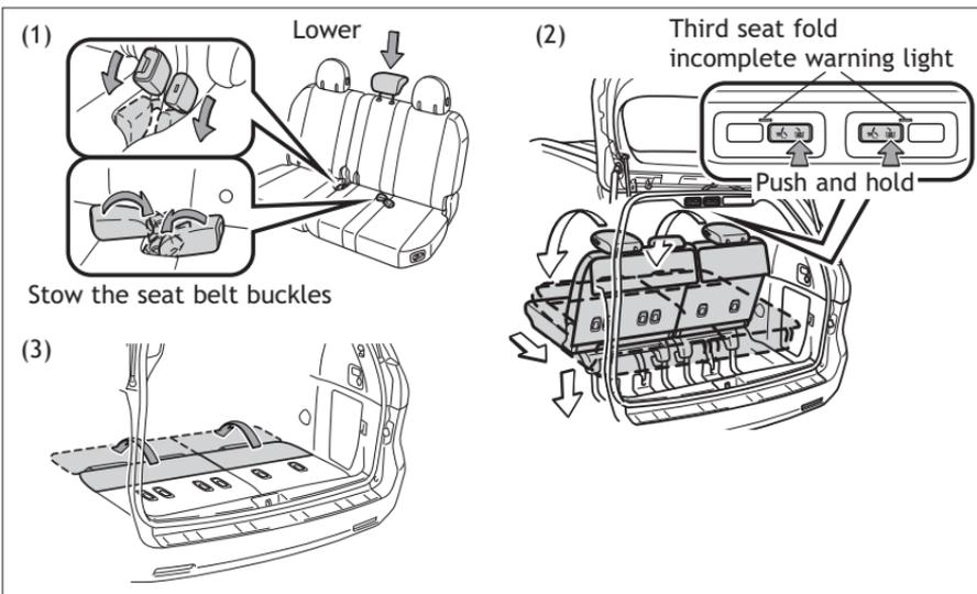
An alarm will sound for 10 seconds and the **3RD SEAT** indicator will light up on the instrument panel if the seat is not fully open or stowed when vehicle is shifted out of Park.
