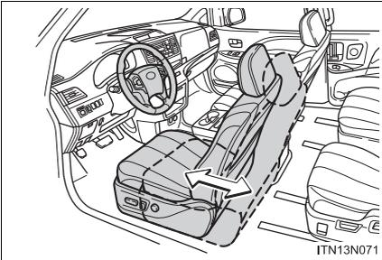
Exiting the vehicle: When all of the following actions have been performed, the seat will move backward (auto away function):
