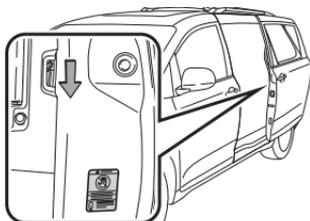
Moving the lever to "LOCK" will allow the door to be opened only from the outside.
