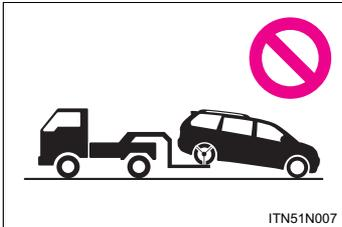
2WD models: Never tow this vehicle from the rear with the front wheels on the ground. This may cause serious damage to the transaxle. If towing from the rear, use towing dolly.
