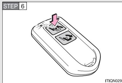
Press and hold the seat raise switch on the wireless remote control to rotate and raise the AUTO ACCESS SEAT.
