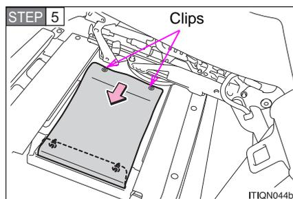
Remove the clips from the unit, and roll back the cover. (→P. 57)
