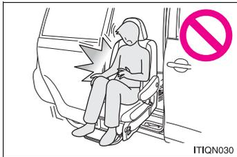
**l** Do not try to close the right-hand sliding door while operating the AUTO ACCESS SEAT. Otherwise, the hands or feet of the occupant may hit the door, possibly causing injuries.
