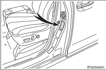
For the GAWR, see the Certification Label. For the maximum load of the tire, see the load limit at maximum cold tire inflation pressure mentioned on the sidewall of the tire. (→P. 749)
