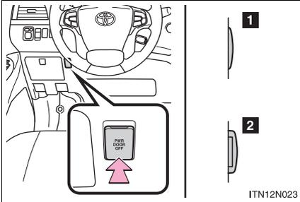
Turn the main switch off to disable the power back door system.
