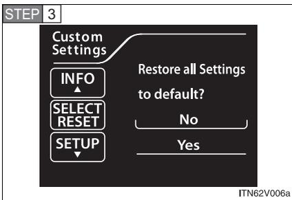
Select “Yes” by pressing the “INFO” or “SETUP” button, and press the “SELECT RESET” button.
