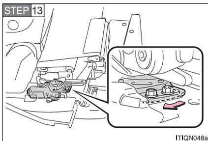
Use the combination wrench to loosen the two bolts, then slide the motor out of the way and disconnect it from the gear.
