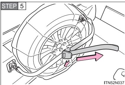
Pull strap to tighten and secure tire.
