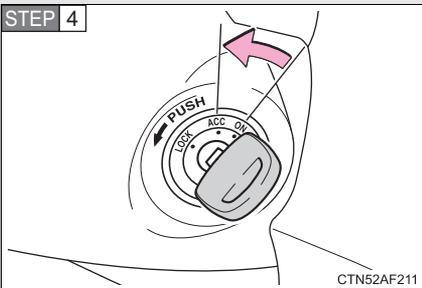
Vehicles without a smart key system: Stop the engine by turning the engine switch to "ACC".
