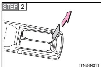
Remove the insulating sheet.
