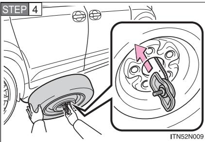
Take the spare tire out from underneath the vehicle and remove the holding bracket.
