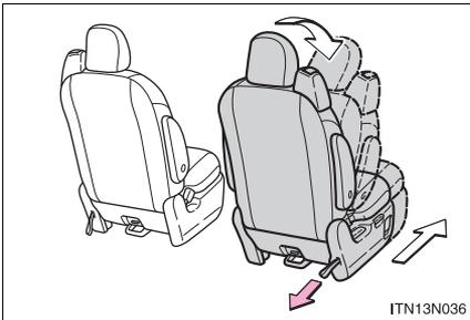
Pull the strap and fold down the seatback. The seat can slide forward.
