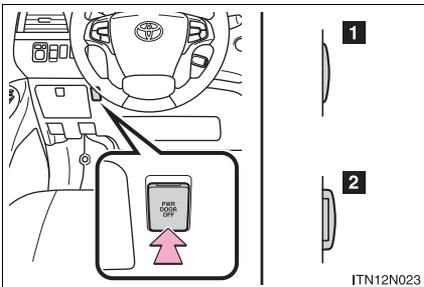
Turn the main switch off to disable the power sliding door system.
