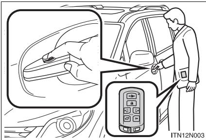
Touch the lock sensor (the indentation on the upper part of the door handle) to lock all the doors.
