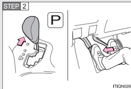
Shift the shift lever to P and set the parking brake.
