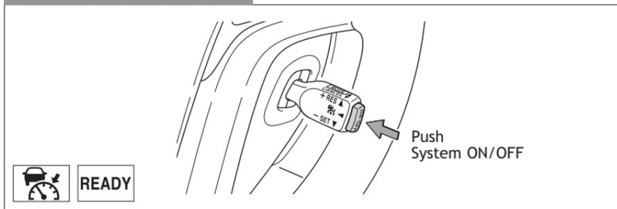
The distance control mode will cruise at a set speed, decelerate to maintain a selected distance from a slower vehicle traveling in front of you, and accelerate back up to the selected speed if the vehicle in front changes lanes or speeds up.
