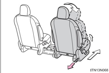
Pull the strap and fold down the seatback. The cushion will tip up. The seat can slide forward. Move the seat to the front-most position.
