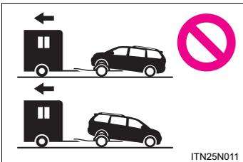
AWD models: Never tow this vehicle with any of the wheels on the ground. This may cause serious damage to the transaxle and Active Torque Control 4WD system.
