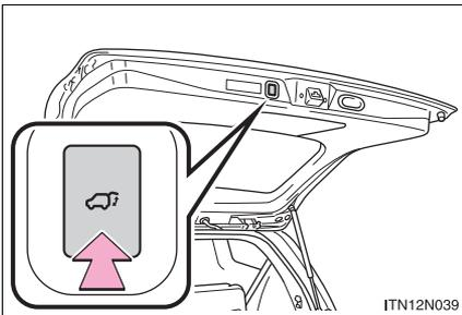
Press the switch to close the back door.
