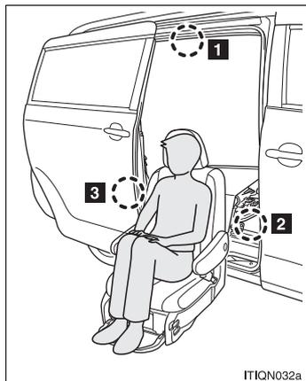
When operating the AUTO ACCESS SEAT, make sure that the occupant's head, arms and legs do not hit the door opening.
