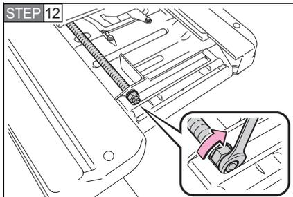
Turn the bolt with yellow marking clockwise using the combination wrench, and slide the seat until the marks are aligned as shown in the illustration.
