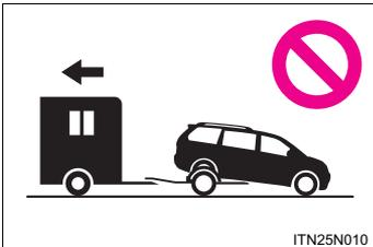
2WD models: Never tow this vehicle from the rear with the front wheels on the ground. This may cause serious damage to the transaxle.
