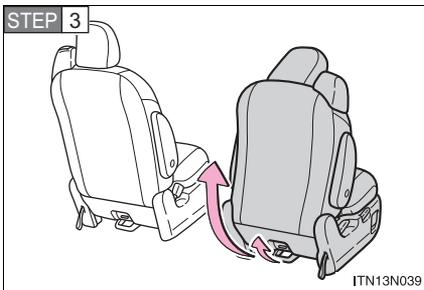
Pull the release lever behind the seatback and simultaneously lift the seat to remove.
