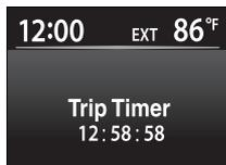
Displays the elapsed time since the timer was reset.
