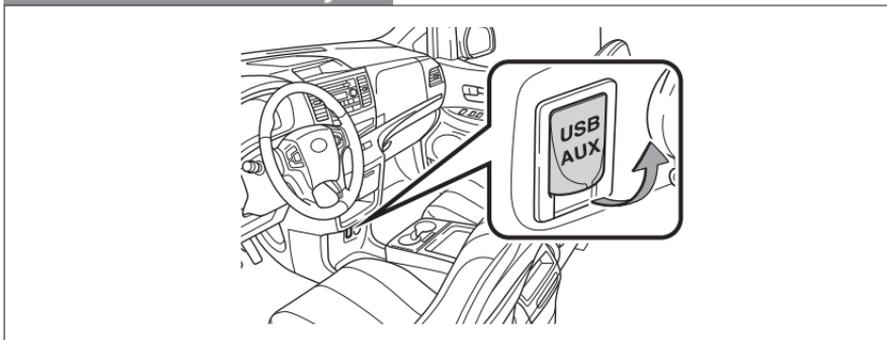
By inserting a mini plug into the AUX or USB/AUX audio jack, you can listen to music from a portable audio device through the vehicle's speaker system while in AUX or USB/AUX mode.
