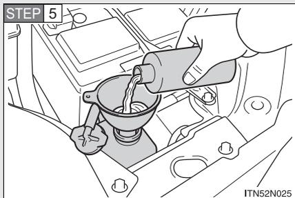
Add engine coolant if necessary.
