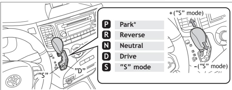
\* The "ENGINE START STOP" switch/engine switch must be "ON" and the brake pedal depressed to shift from Park.
