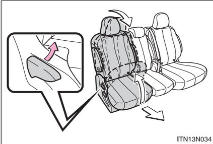
Pull the seatback angle adjustment lever and fold down the seatback. The cushion will tip up. The seat can slide forward. Move the seat to the front-most position.
