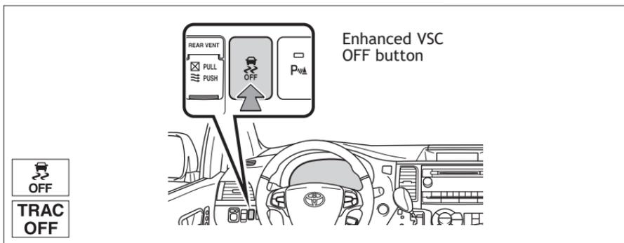
The Enhanced VSC OFF button is used to switch between modes related to the TRAC and Enhanced VSC functions.
