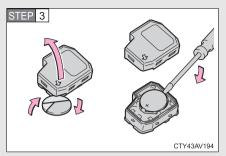
Open the case cover using a coin protected with tape etc. and remove the depleted battery using a small flathead screwdriver.
