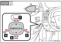
To adjust the mirror, press the switch.
