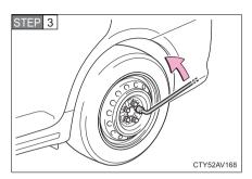
Slightly loosen the wheel nuts (one turn).
