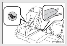
LATCH anchors are provided for the outer rear seats. (Buttons displaying the location of the anchors are attached to
