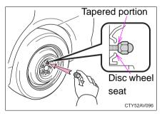
When replacing a steel wheel with a steel wheel, tighten the wheel nuts until the tapered portion comes into loose contact with the disc wheel seat.
