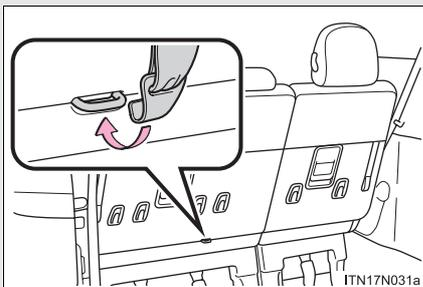
An anchor bracket is provided for center seat.
