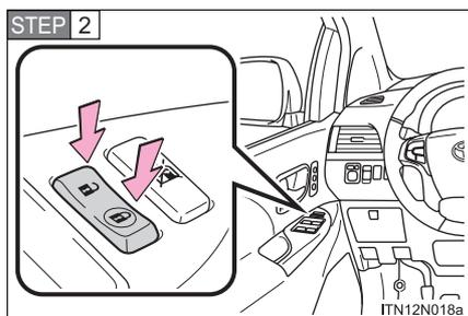
Shift the shift lever to P or N, and press and hold the door lock switch (🔒 or 🔓) for approximately 5 seconds and then release.
