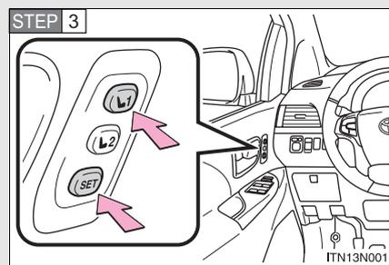
Press the "SET" button, then within 3 seconds press button "1" or "2" until the signal beeps.
