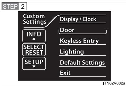
Select the setting you wish to change by pressing the “INFO” or “SETUP” button, then press the “SELECT RESET” button to select.
