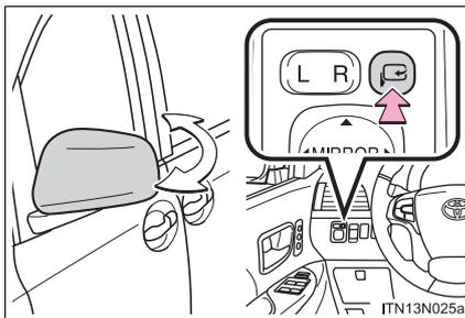
Press the switch to fold the mirrors.
