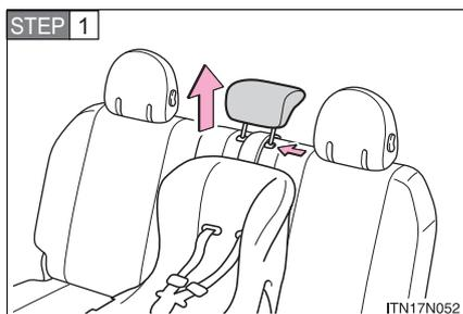
Secure the child restraint system using the seat belt or LATCH anchors. Adjust the head restraint to the uppermost position.
