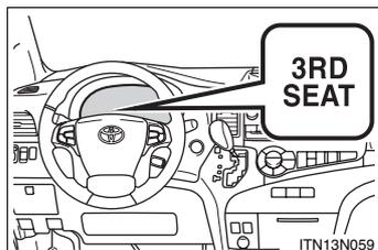
The warning light comes on if the third seat operation is not yet complete when the engine switch is turned to the “ON” position (vehicles without a smart key system) or the “ENGINE START STOP” switch is in IGNITION ON mode (vehicles with a smart key system).
