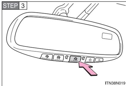
Test the operation of the HomeLink® by pressing the newly programmed button.
