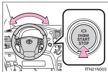
The green indicator light on the “ENGINE START STOP” switch will flash and a message will be shown on the multi-information display. Press the “ENGINE START STOP” switch while turning the steering wheel left and right.
