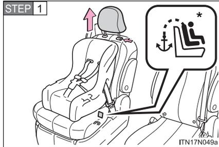
Secure the child restraint system using the seat belt or LATCH anchors, and adjust the head restraint to the uppermost position.
