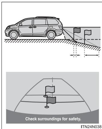
When the grade behind the vehicle slopes down sharply, objects appear to be closer than they actually are.
