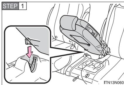
Engage the rear pins with the hooks.
