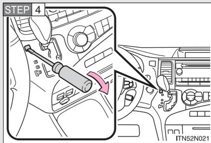
Pry the cover up with a flat-head screwdriver or equivalent tool.
