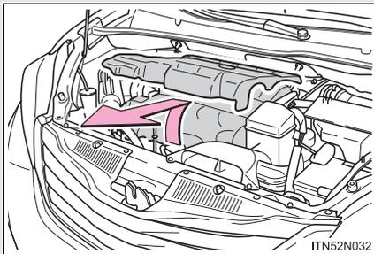
Lift the edge of the cover to fixed pins, and then pull the cover towards you to remove.
