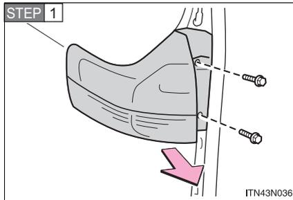
Remove the securing bolts and remove the unit.
