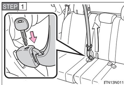
Insert the key or tab "A" into the hole on the center seat belt buckle to release the hooked tab "B" and allow the belt to retract.
