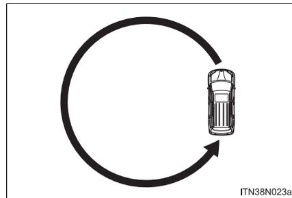
When "C" appears on the display, drive the vehicle at 5 mph (8 km/h) or less in a circle until a direction is displayed.
