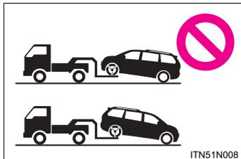
AWD models: Never tow this vehicle with any of the wheels on the ground. This may cause serious damage to the transaxle and Active Torque Control 4WD system. Use a towing dolly.
