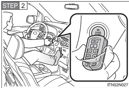
**STEP 2** Touch the Toyota emblem side of the electronic key to the “ENGINE START STOP” switch.
