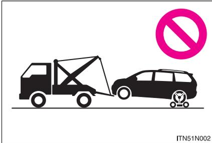
Do not tow with a sling type truck to prevent body damage.
