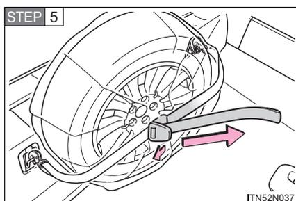
Pull strap to tighten and secure tire.
