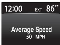
Displays the average vehicle speed since the engine was started or since the function was reset.
