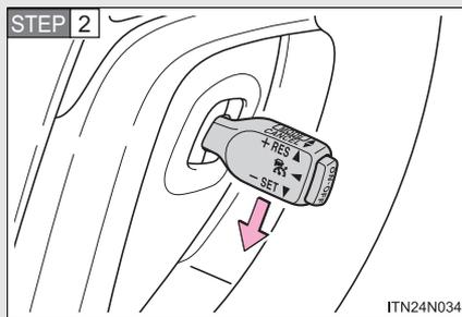
Accelerate or decelerate to the desired speed and push the lever down to set the speed.
