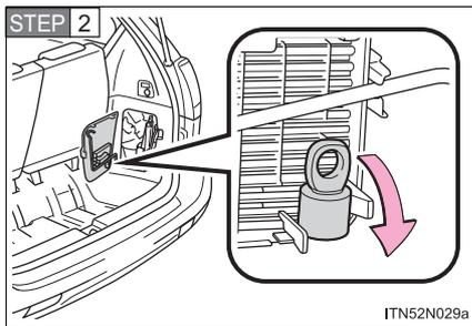
Remove the adapter socket.
