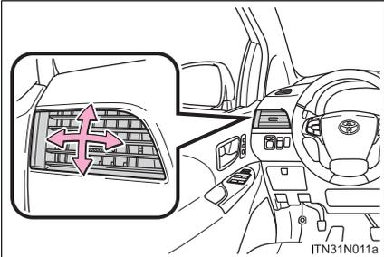
Adjusting: Direct air flow to the left or right, up or down.
