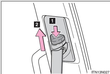
**1** Push the seat belt shoulder anchor down while pressing the release button.
