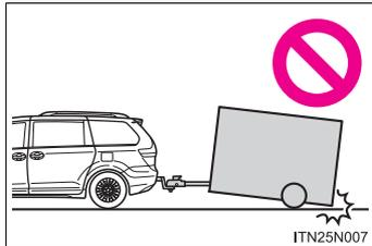
No matter which class of tow hitch applies, for a safe trailer hookup, the trailer ball setup on must be proper height for the coupler on the trailer.
