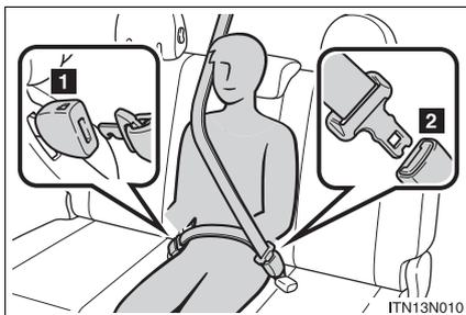
Make sure that the buckle **1** is securely latched for ready use of the center seat belt.
