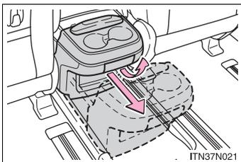
Pull up the lever and slide the console box.
