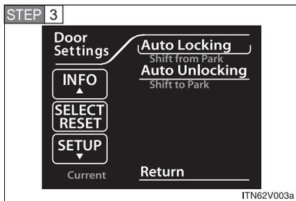
Select the setting you wish to change by pressing the “INFO” or “SETUP” button, and press the “SELECT RESET” button.
