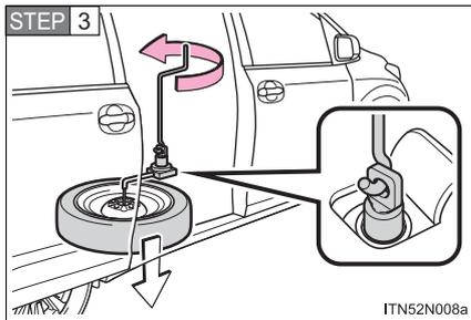
Attach the adapter socket over the spare tire clamp bolt.
