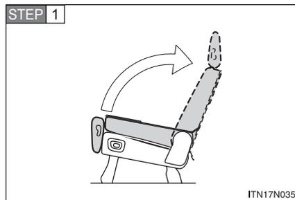
Fold down the seatback by pressing the folding/returning switch (→P.110). Raise the seatback by pressing the same switch, the returning switch (→P.114) or the seatback angle adjustment switch (→P.101). (The seatback will automatically stop.) Do not touch the switch while the seatback is moving, because the operation will stop.
