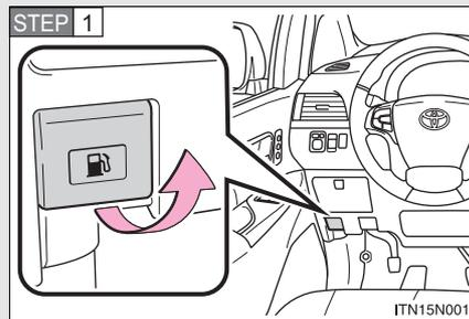
Pull up the opener to open the fuel filler door.
