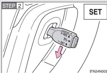
Accelerate or decelerate the vehicle to the desired speed, and push the lever down to set the speed.
