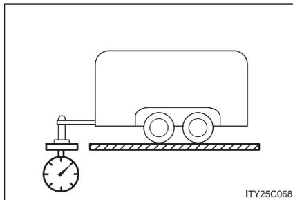
The load placed on the trailer hitch ball. (→P. 362)
