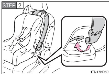
Latch the hook onto the anchor bracket and tighten the top tether strap.
