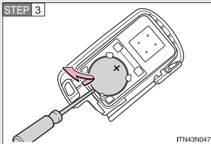
Remove the depleted battery.
