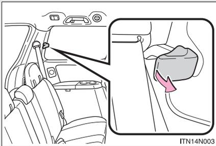
Pull the handle and swing the window fully out to open.
