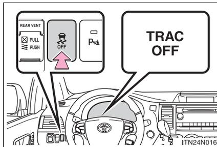
To turn the TRAC system off, quickly press and release the button.
