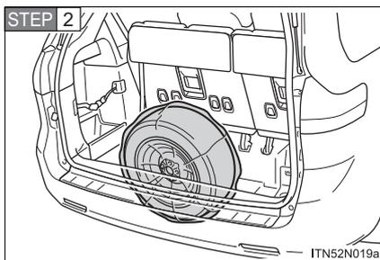
Place tire standing up in rear tub, after putting the tire in the tire bag.
