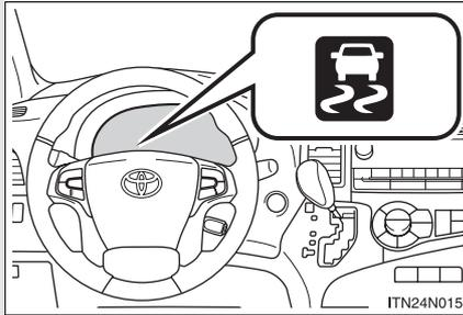
To engage hill-start assist control, further depress the brake pedal when the vehicle is stopped completely.
