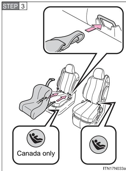
Latch the hooks of the lower straps onto the LATCH anchors. If the child restraint has a top tether strap, the top tether strap should be latched onto the top tether strap anchor.
