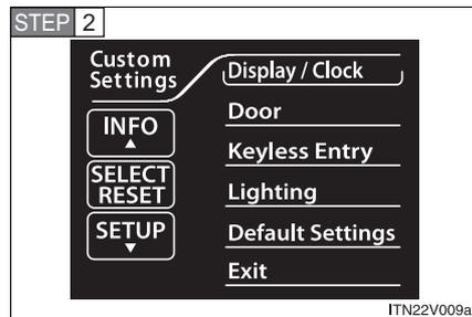
Select “Display / Clock” by pressing the “INFO” or “SETUP” button, and press the “SELECT RESET” button.
