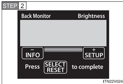
Press the “INFO” or “SETUP” button to adjust the brightness.
