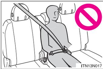
Do not use the third center seat belt with either buckle released. Fastening only one of the buckles may result in death or serious injury in case of sudden braking or a collision.
