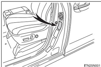
For the GAWR, see the Certification Label. For the maximum load of the tire, see the load limit at maximum cold tire inflation pressure mentioned on the sidewall of the tire. (→P. 801)
