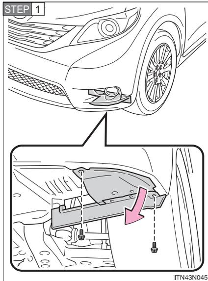
Remove the engine under cover bolt and pull down the engine under cover.
