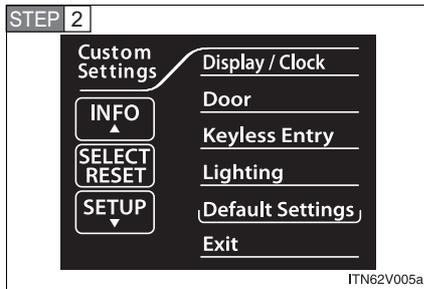
Select “Default Settings” by pressing the “INFO” or “SETUP” button, and press the “SELECT RESET” button.
