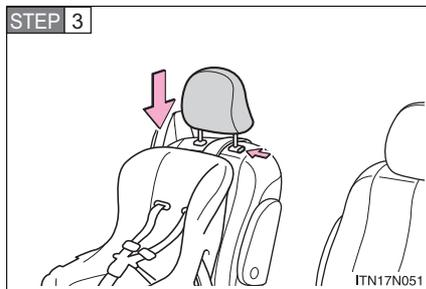
Adjust the head restraint to the downmost lock position.
