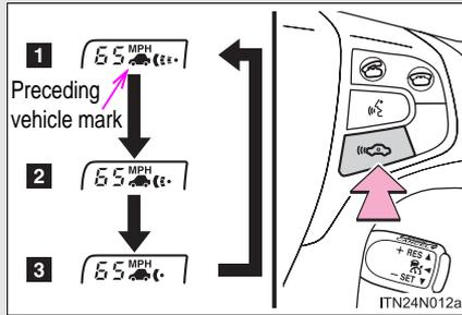
Pressing the button changes the vehicle-to-vehicle distance as follows:
