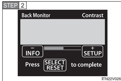
Press the “INFO” or “SETUP” button to adjust the contrast.
