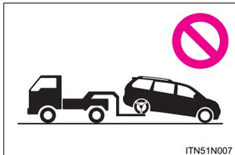
2WD models: Never tow this vehicle from the rear with the front wheels on the ground. This may cause serious damage to the transaxle. If towing from the rear, use a towing dolly.
