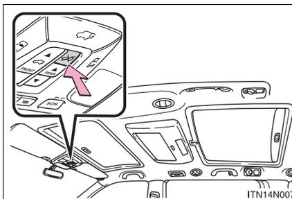
Press the switch to disable the rear moon roof operation from the rear seat.
