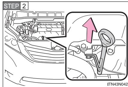
**STEP 2** Holding a rag under the end, pull the dipstick out.
