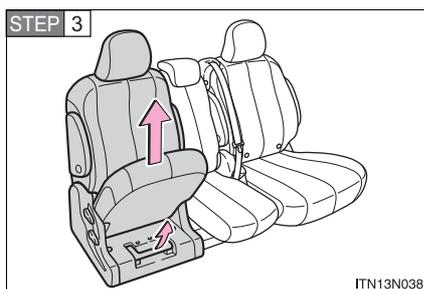
Pull the release lever under the cushion and simultaneously lift the seat to remove.
