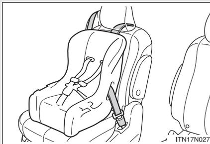
Seat belts equipped with a child restraint locking mechanism (ALR/ELR belts except driver's seat belt) (→P. 131)
