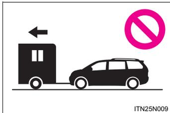
Do not tow your vehicle with four wheels on the ground.
