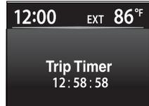
Displays the elapsed time since the timer was reset.
