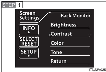
Select “Contrast” on the “Screen Settings” screen, and press the “SELECT RESET” button.
