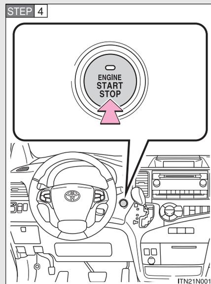
Press the “ENGINE START STOP” switch.
