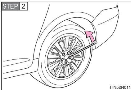
Slightly loosen the wheel nuts (one turn).
