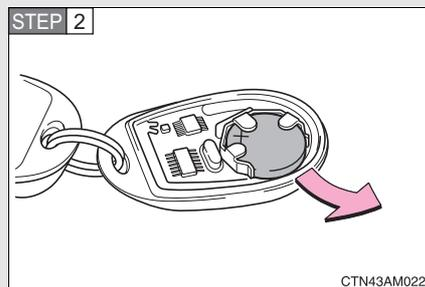
Remove the discharged transmitter battery.
