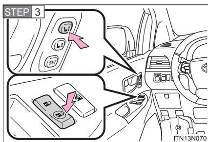
Press the desired button (“1” or “2”) to recall the position. Then, while keep pressing the button, press the driver’s door lock switches (either lock or unlock) until the signal beeps.
