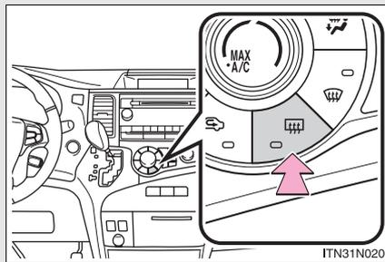
Turns the rear window and outside rear view mirror defoggers and windshield de-icer on/off.
