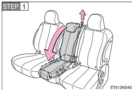
Pull the lock release strap and fold down the second center seatback.
