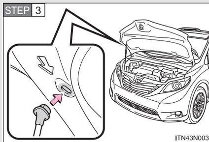
Hold the hood open by inserting the supporting rod into the slot.
