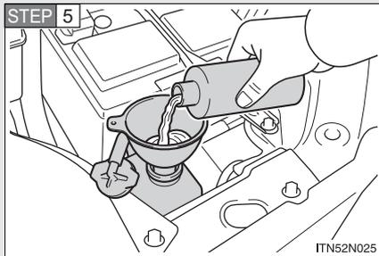
Add engine coolant if necessary.
