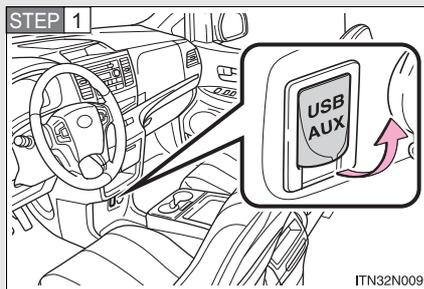
Open the cover and connect an iPod using an iPod cable.
