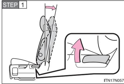
Fold the seatback while pulling the lever and move to the rear-most recline position.
