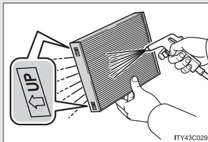
If the filter is dirty, clean by blowing compressed air through the filter from the underside.
