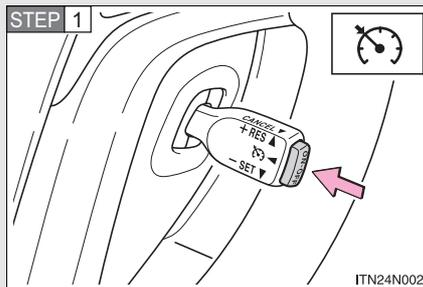
Press the “ON-OFF” button to activate the cruise control.
