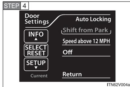
Choose a desired setting by pressing the “INFO” or “SETUP” button, then press the “SELECT RESET” button to select.
