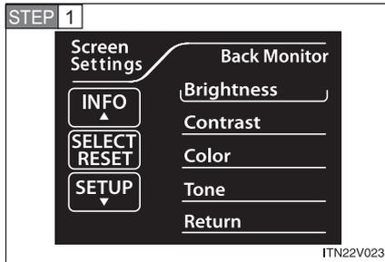
Select “Brightness” on the “Screen Settings” screen, and press the “SELECT RESET” button.
