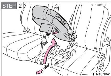
Pull the lock release strap under the seat to remove the seat.
