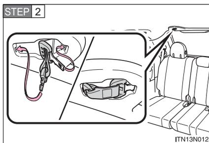
Stow the seat belt tabs in the cover set in the roof as shown.
