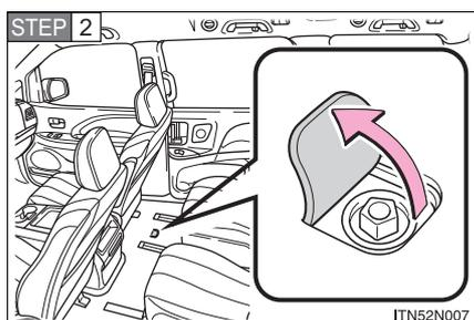
Open the right side sliding door and you will find the flap on the floor. Pull back the flap to find the spare tire clamp bolt.
