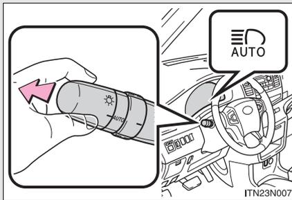
Push the lever away from you with the headlight switch in the **AUTO** position when the “ENGINE START STOP” switch is in IGNITION ON mode (vehicles with a smart key system) or the engine switch is in the “ON” position (vehicles without a smart key system).
