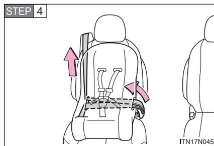
While pushing the child restraint system into the rear seat, allow the shoulder belt to retract until the child restraint system is securely in place.
