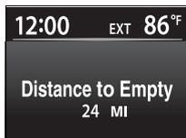
Displays the estimated maximum distance that can be driven with the quantity of fuel remaining.
