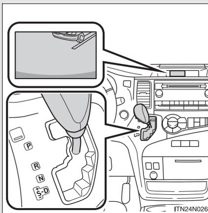
The rear view image is displayed when the shift lever is in the R position.
