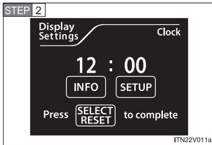
Press the “INFO” button to adjust the hours and the “SETUP” button to adjust the minutes.
