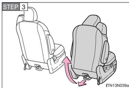
Pull the release lever behind the seatback straight back, then up. While moving the lever up, simultaneously lift the seat to remove.
