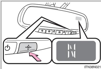
To turn the compass on or off, press the switch.
