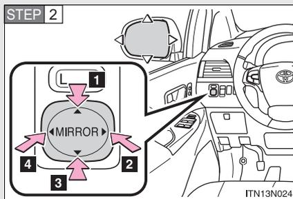
To adjust the mirror, press the switch.
