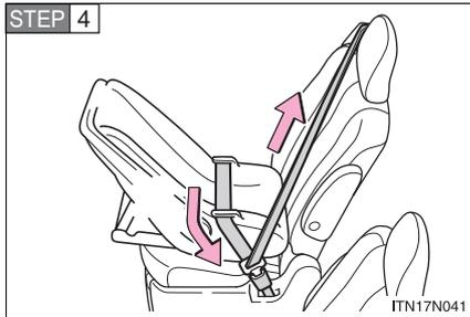
While pushing the child restraint system down into the rear seat, allow the shoulder belt to retract until the child seat is securely in place.
