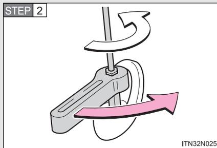
Loosen the antenna with the wrench and remove it.
