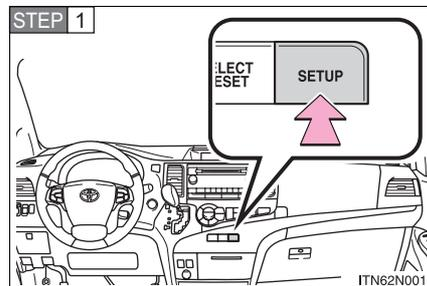
Press the “SETUP” button while the vehicle is stopped.
