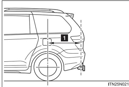
**1** Hitch receiver pin hole position: 37.3 in. (949.8 mm)
