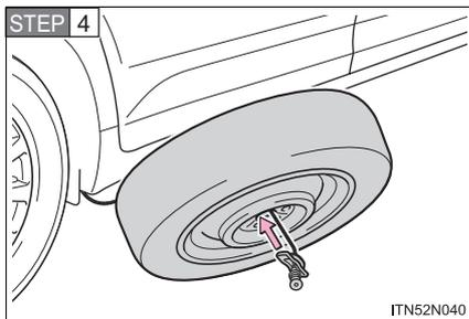
Take the spare tire out from underneath the vehicle and remove the holding bracket.
