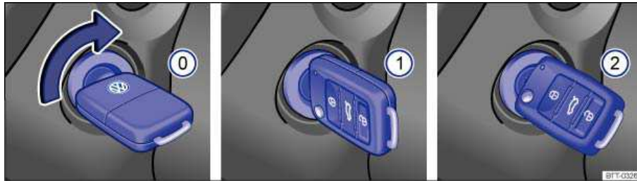
Fig. 111 In the ignition switch: Vehicle key positions.
