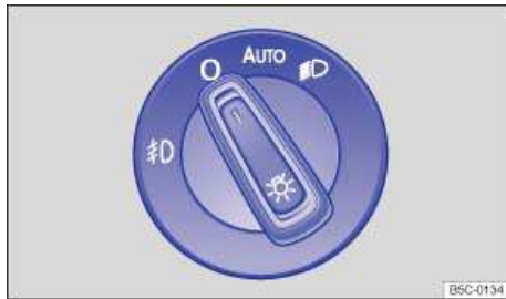
Fig. 72 Headlight switch next to the steering wheel (with fog lights and automatic headlight control).
