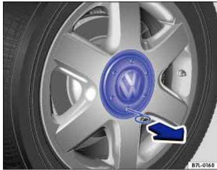
Fig. 155 Pulling the hubcap off.
