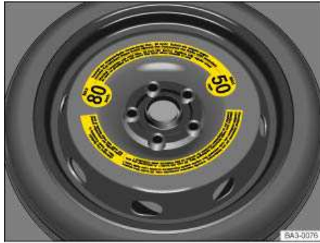
Fig. 95 In the luggage compartment: Compact spare wheel.
