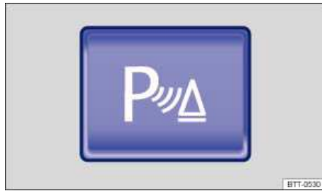
Fig. 130 In the center console: Button to switch the Park Distance Control system on or off.
