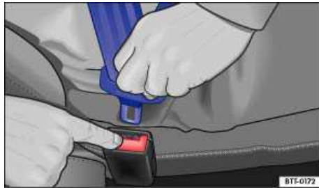
Fig. 52 Releasing the buckle tongue from the belt buckle.
