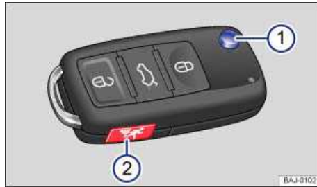
Fig. 20 Remote control vehicle key with panic button.
