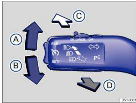
Fig. 70 Turn signal lever and high beam switch.
