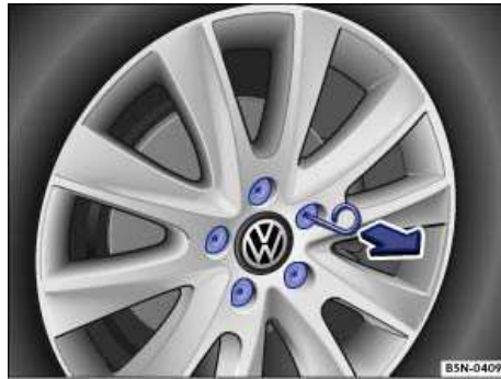
Fig. 157 Pulling cover caps off wheel bolts.
