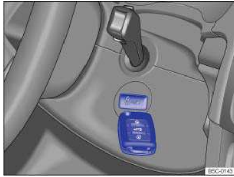
Fig. 113 Hold the remote control vehicle key to the right of the steering column: Emergency starting feature on vehicles with Keyless Access.
