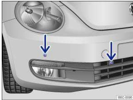
Fig. 129 In the front bumper: Park Distance Control system sensors.
