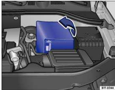
Fig. 143 In the engine compartment: Open the sleeve covering of the vehicle battery.
