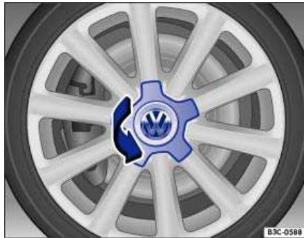
Fig. 156 Twisting the hubcap off.
