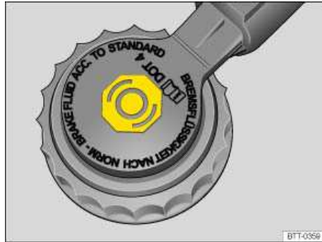
Fig. 122 In the engine compartment: Brake fluid reservoir cap.
