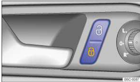
Fig. 25 In the vehicle doors: Power locking button.
