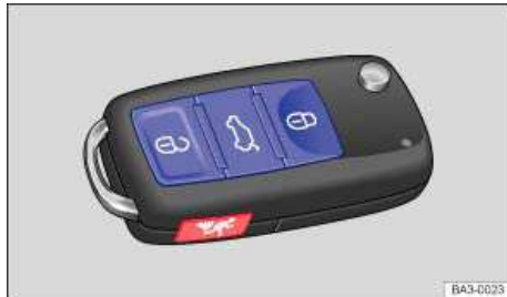
Fig. 24 Remote control vehicle key with panic button.
