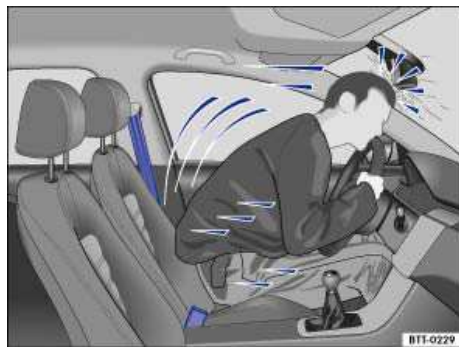
Fig. 48 The unbelted driver is thrown forward.
