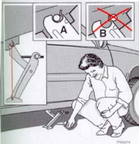
Jack attachment - front wheel drive models
