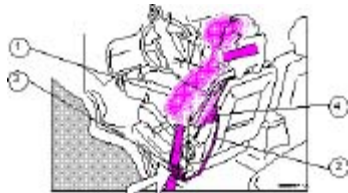
1 - Airbag, 2 - cable, 3 - sensor unit,
