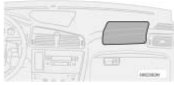
Passenger side airbag - location
