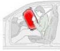
Driver's side airbag - in steering wheel hub
