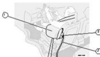
1 - Airbag, 2 - wire, 3 - gas generator/sensor unit
