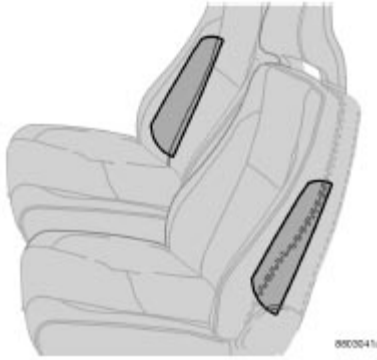
Location of the side impact (SIPS) airbag
