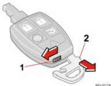
Removing the key blade
