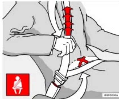
Adjusting the seat belt
