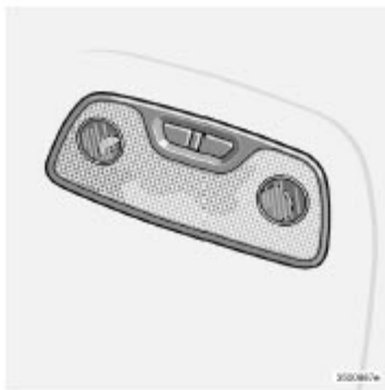
Rear reading lights (in ceiling)
