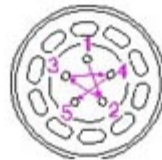
Correct tightening order for wheel bolts
