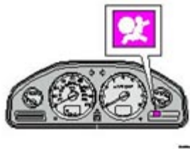
SRS warning light
